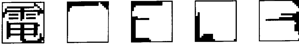
Fig. 4.2 Contour features of a Chinese character: (a) a Chinese character; (b) top-bottom contour feature; (c) left-right contour feature; (d) bottom-top contour feature; (e) right-left contour feature.
