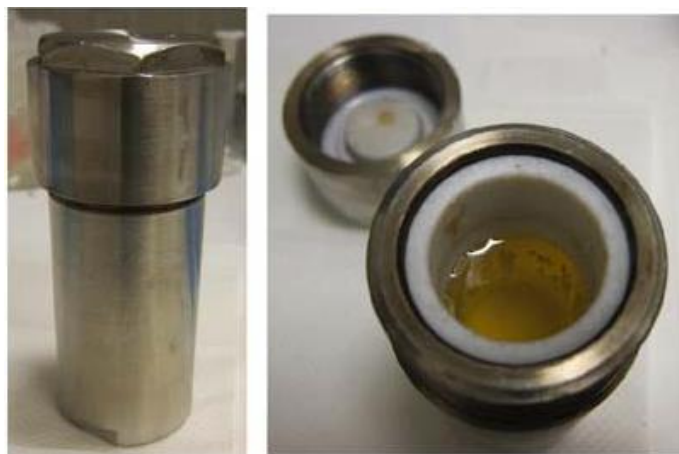
Figure 10 Photographs of the autoclave for one-step hydrothermal synthesis. The white part is the Teflon lining of the container.
