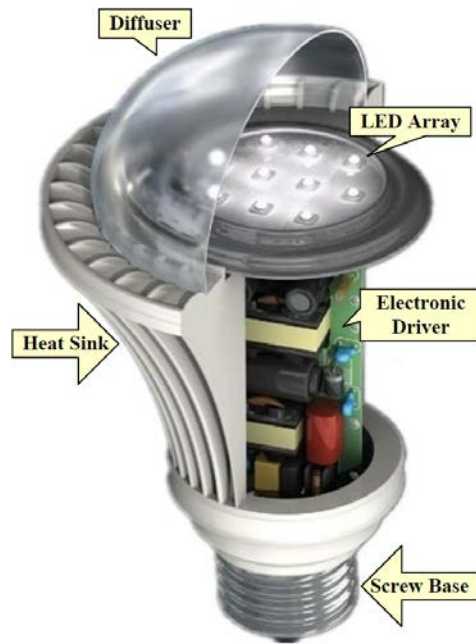
Figure 1.2: Breakdown of an LED lamp.
