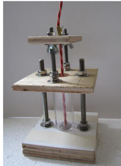
Figure 5-1 Schematic diagram and photograph of the cross-sectional sample preparation device
