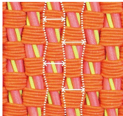
Figure 6-10 Alignment of 4-ply auxetic yarns in the fabric sample
