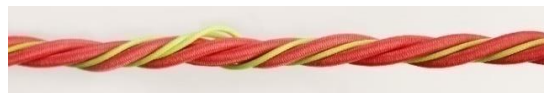
Figure 4-15 Photograph of 6-ply auxetic yarn sample at the end of the first cycle.
