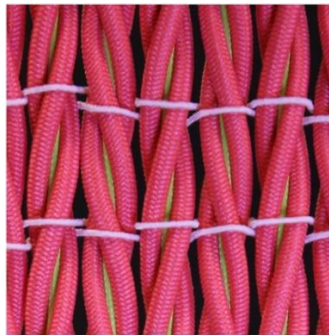
Figure 6-22 Sample F12 at strain of 0.4
