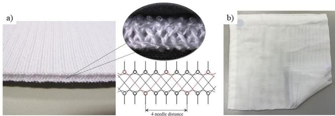
Figure 4.1 a) spacer fabric and its cross section and b) 4-layered cotton fabric.
