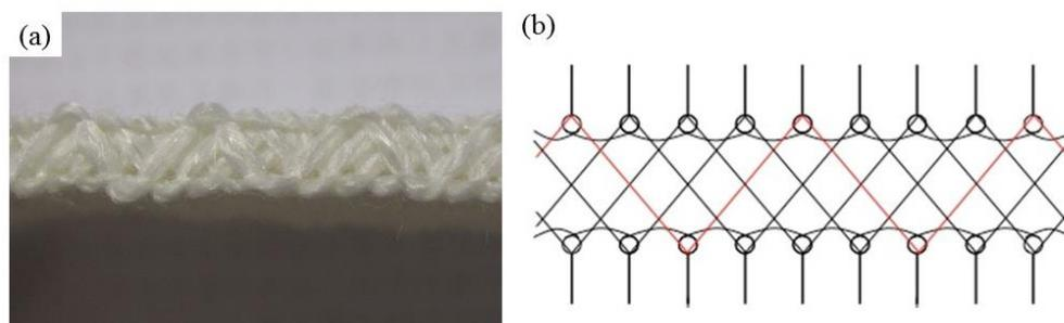
Figure 2.7 Tuck structure of a typical weft-knitted spacer fabric produced with flat knitting machine: (a) real fabric, (b) scheme.
