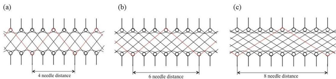
Figure 3.2 Spacer fabric structures with (a) 4, (b) 6, (c) 8 needle connecting distance.
