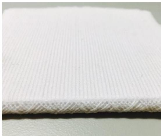
Figure 3.3 3D view of a typically fabricated spacer fabric.
