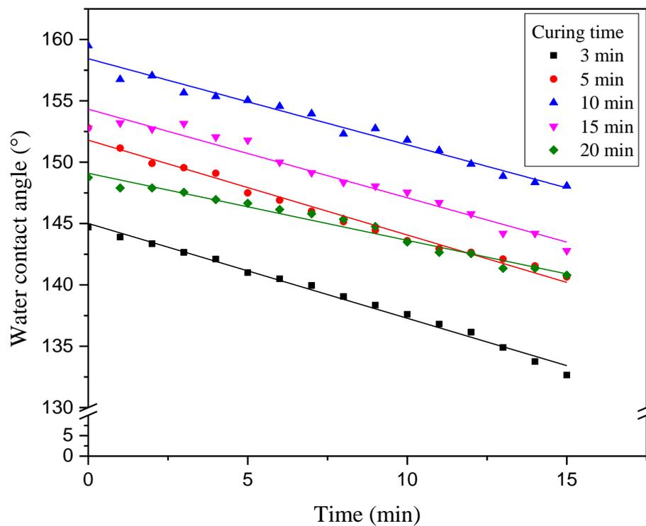
Figure 5.10 Effect of curing time on water contact angle.
