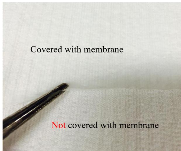
Figure 5.2 Covering of the electrospun nanofibrous membrane onto spacer fabric.
