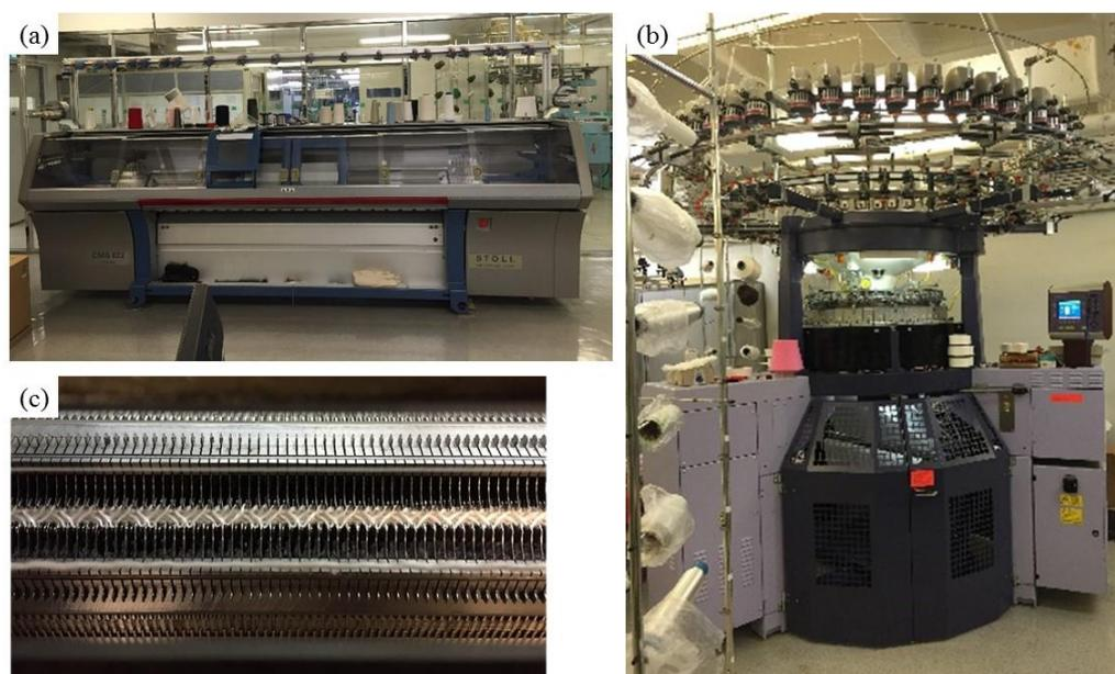
Figure 2.6 (a) A STOLL computerized flat knitting machine; (b) a Terrot double jersey circular machine; (c) knitting a spacer fabric on the computerized flat
