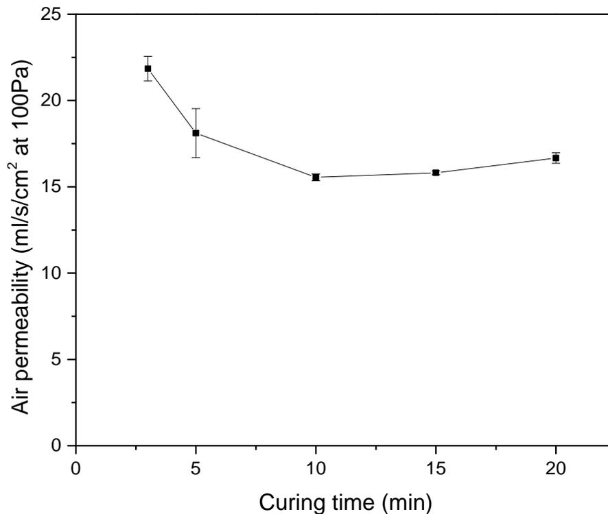
Figure 5.11 Effect of curing time on air permeability.
