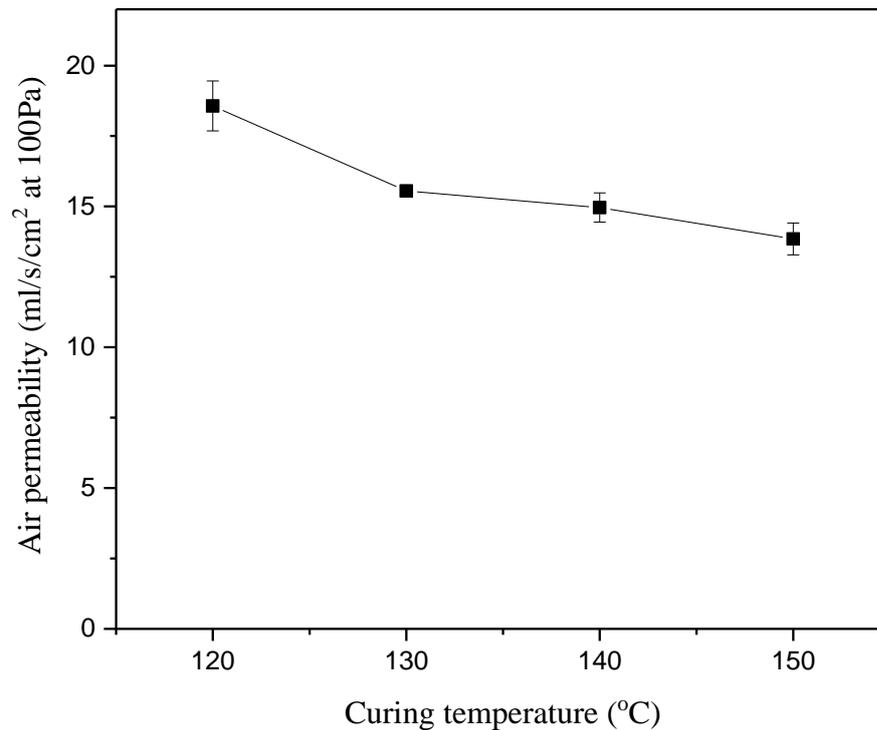
Figure 5.13 Effect of curing temperature on air permeability.
