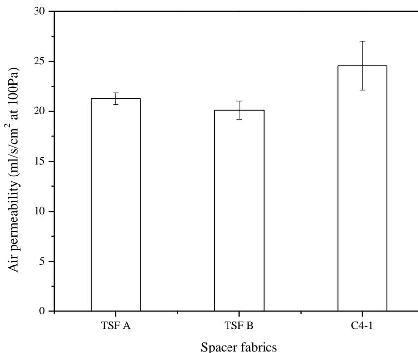
Figure 5.7 Air permeability of spacer fabrics.
