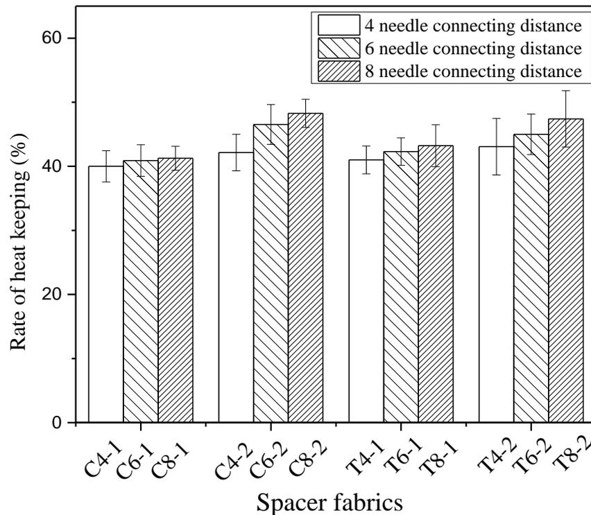
Figure 3.10 Rate of thermal property of spacer fabrics.
