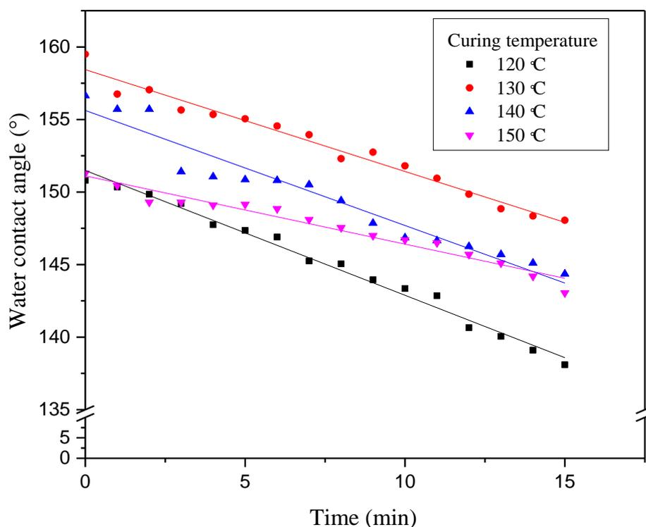
Figure 5.12 Effect of curing temperature on water contact angle.
