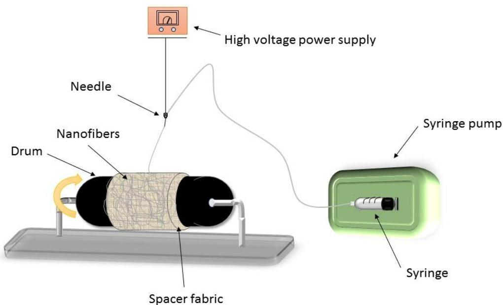
Figure 5.1 Fabrication process of the electrospun nanofibrous membrane on spacer fabric.
