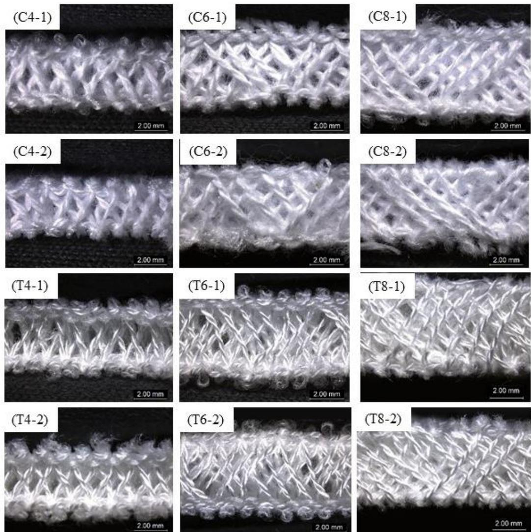
Figure 3.4 Cross-section of spacer fabrics.
