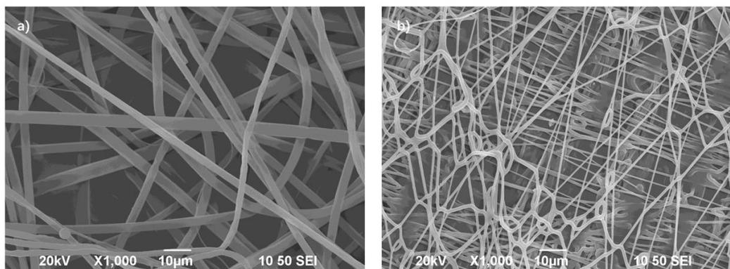
Figure 5.4 SEM images of a) polystyrene and b) polyurethane electrospun nanofibrous membranes.
