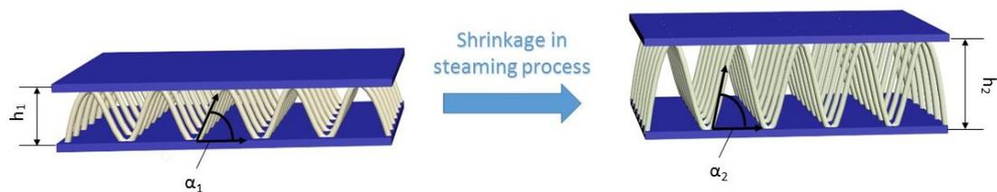
Figure 3.5 Shrinkage process of a spacer fabric in steaming stage.
