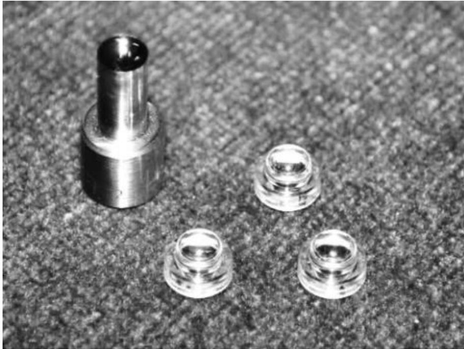
Figure 2.2 Mold insert and the injection-molded camera lenses for mobile phones
