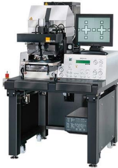
Fig. 3.2 Suss MA6 Mask Aligner: Light source of 350 W UV light at 365 nm; Resolution <math>< 0.8 \mu\text{m}</math>; Alignment accuracy <math>< \pm 0.5 \mu\text{m}</math>; Substrate up to 4-inch round wafer.
