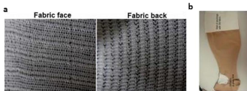
**Figure 2.24:** Stocking made of SMPU. (a) Fabric structure. (b) SMP fabric attached to commercial stocking [163].
