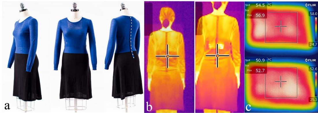
Figure 4.26. (a) Thermal garment with heating area near the waist area; (b) Infrared image of thermal garment when heated; The left thermal garment taking into consideration air flow (left) vs. garment without taking into consideration air flow; (c) it is shown that the garment considering the air flow (up) achieves more precise temperature than the garment without considering that (down) because it provides more power to offset the heat loss;
