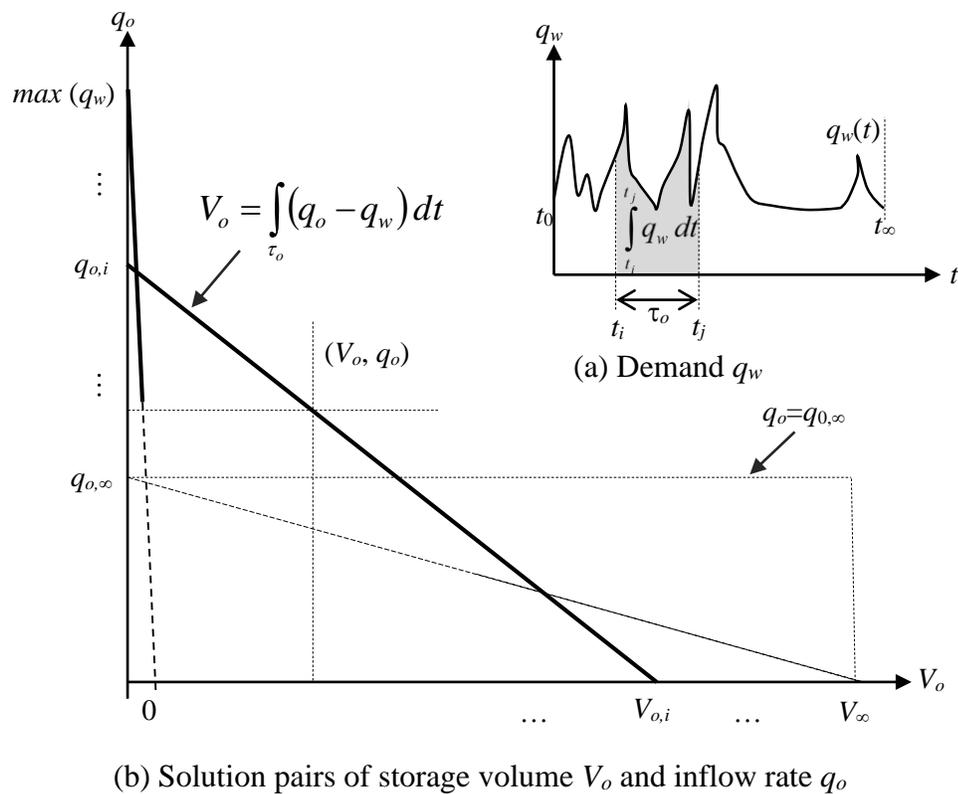
**Figure 3.3 Mass balance at a water storage tank**
