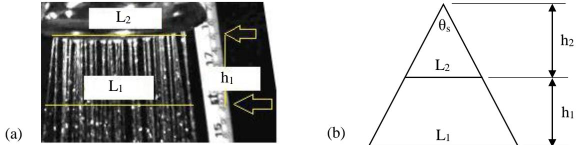
**Figure 3.11 Spray spread angle**
