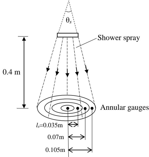
**Figure 3.12 Spray spread angle and water distribution patterns**
