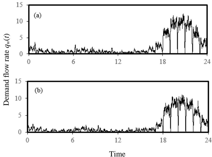
**Figure 5.1 Example demand flow rates for 600 conventional showerheads: (a) maximum daily consumption ( $202.1 \text{ m}^3\text{d}^{-1}$ ); (b) minimum daily consumption ( $180.0 \text{ m}^3\text{d}^{-1}$ )**
