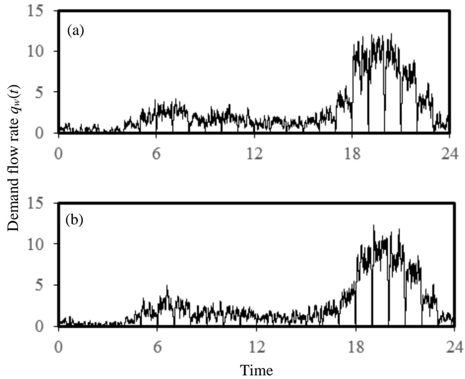
**Figure 5.4 Example demand flow rates for 600 kitchen sinks: (a) maximum daily consumption ( $226.9 \text{ m}^3\text{d}^{-1}$ ); (b) minimum daily consumption ( $208.0 \text{ m}^3\text{d}^{-1}$ )**
