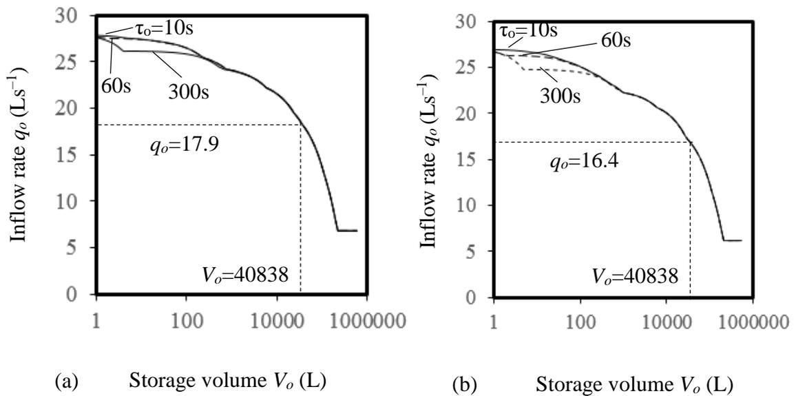
**Figure 5.8 Solutions of inflow rate and storage volume for Case A: (a) for the maximum demand time series in Figure 5.6(a); (b) for the minimum demand time series in Figure 5.6(b)**
