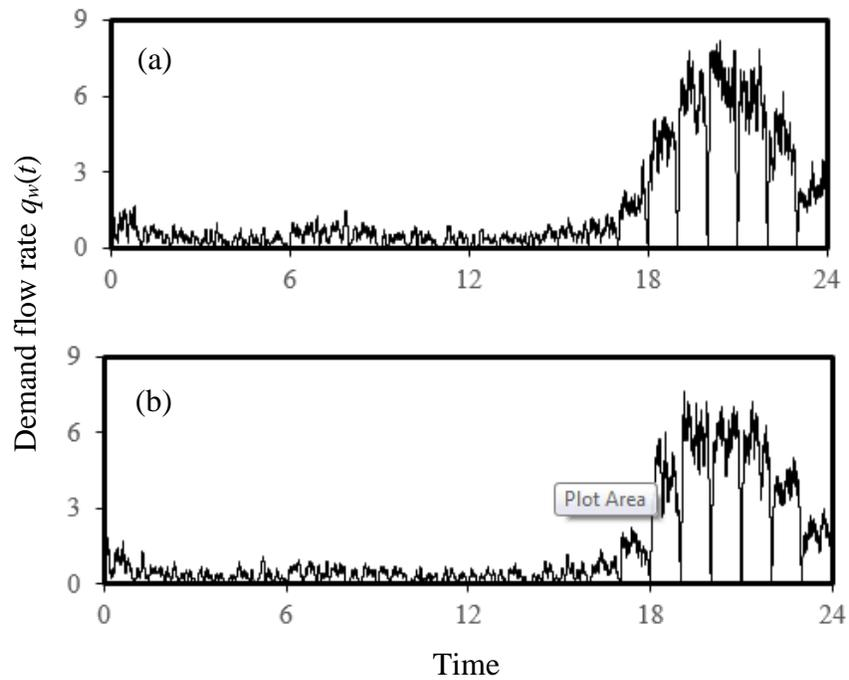
**Figure 5.2 Example demand flow rates for 600 low flow showerheads, i.e. WELS rated Grade 1 showerheads: (a) maximum daily consumption ( $132.8 \text{ m}^3\text{d}^{-1}$ ); (b) minimum daily consumption ( $119.5 \text{ m}^3\text{d}^{-1}$ )**
