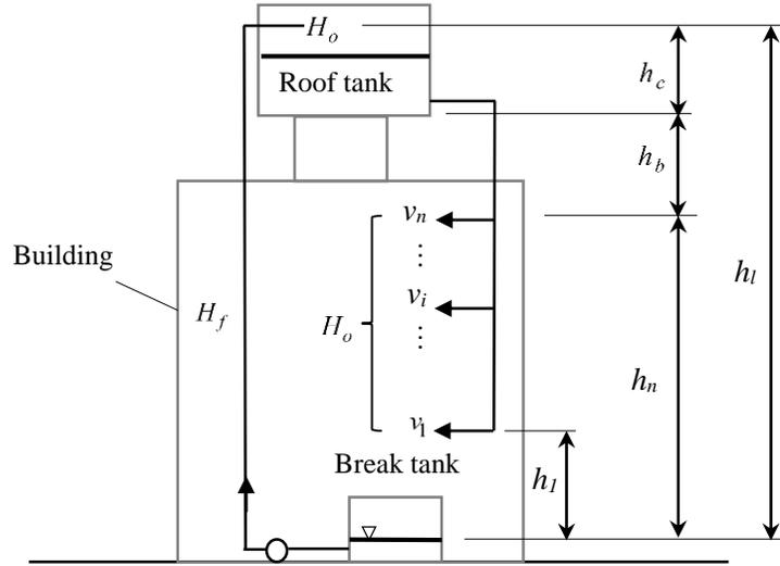
**Figure 3.5 A high-rise roof tank water supply system**
