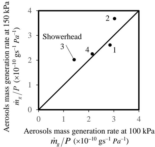
**Figure 6.5 Ratio of aerosol mass generation rate to water supply pressure at showerhead**
