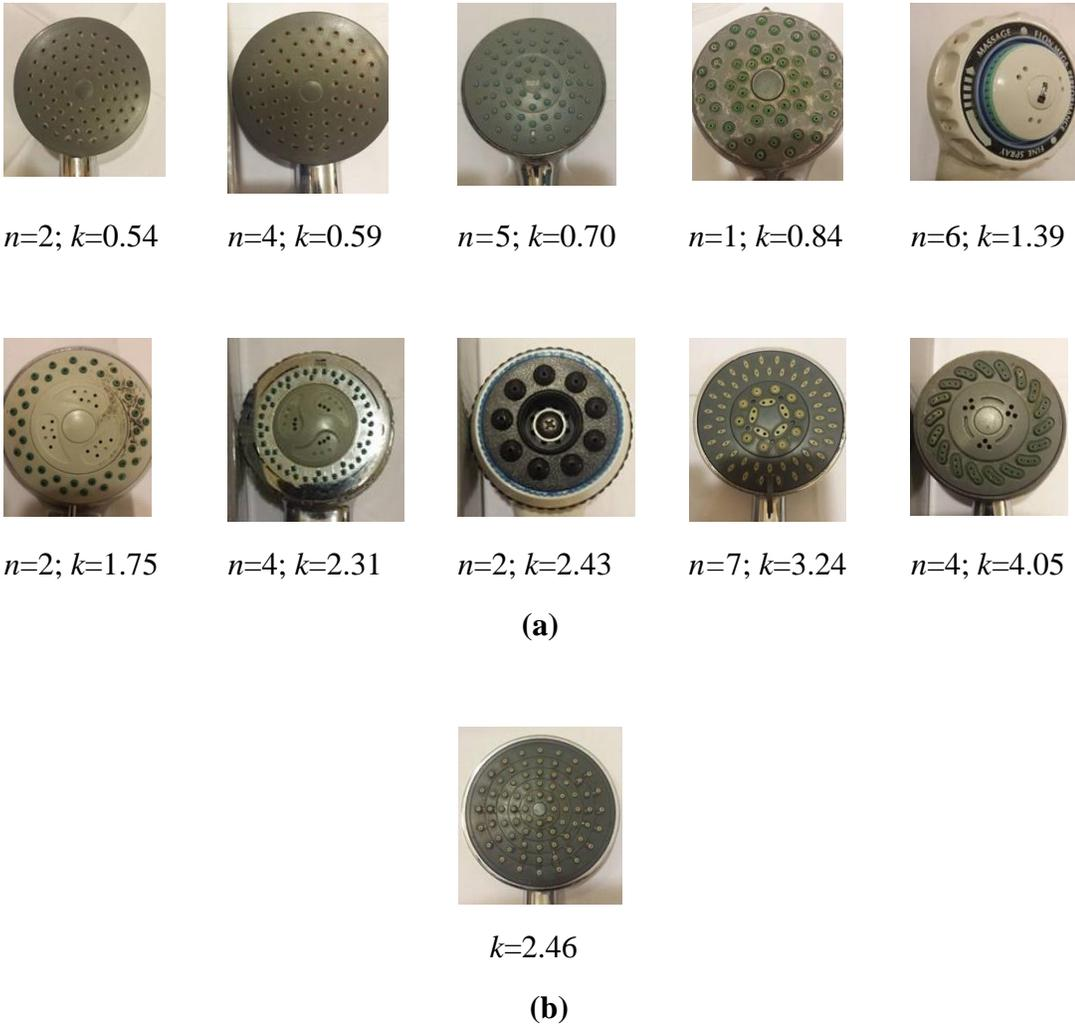
**Figure 4.1 Showerheads under investigation: (a) showerheads already installed in 10 residential washrooms in Hong Kong; (b) a Water Efficiency Labelling Scheme (WELS) rated Grade 2 showerhead**
