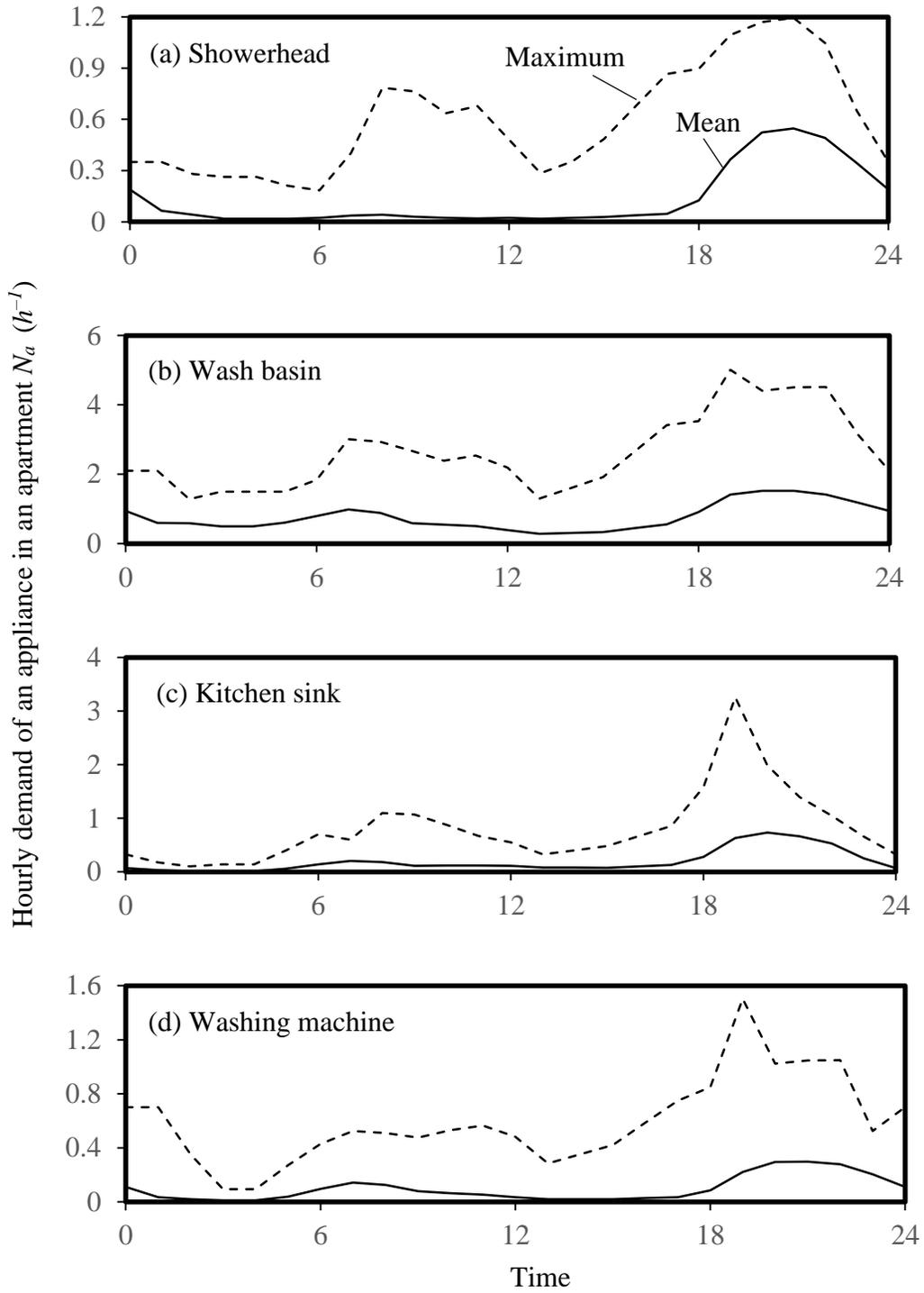
**Figure 2.8 Hourly demand of each type of appliances in an apartment: (a) showerhead; (b) wash basin; (c) kitchen sink; (d) washing machine**
