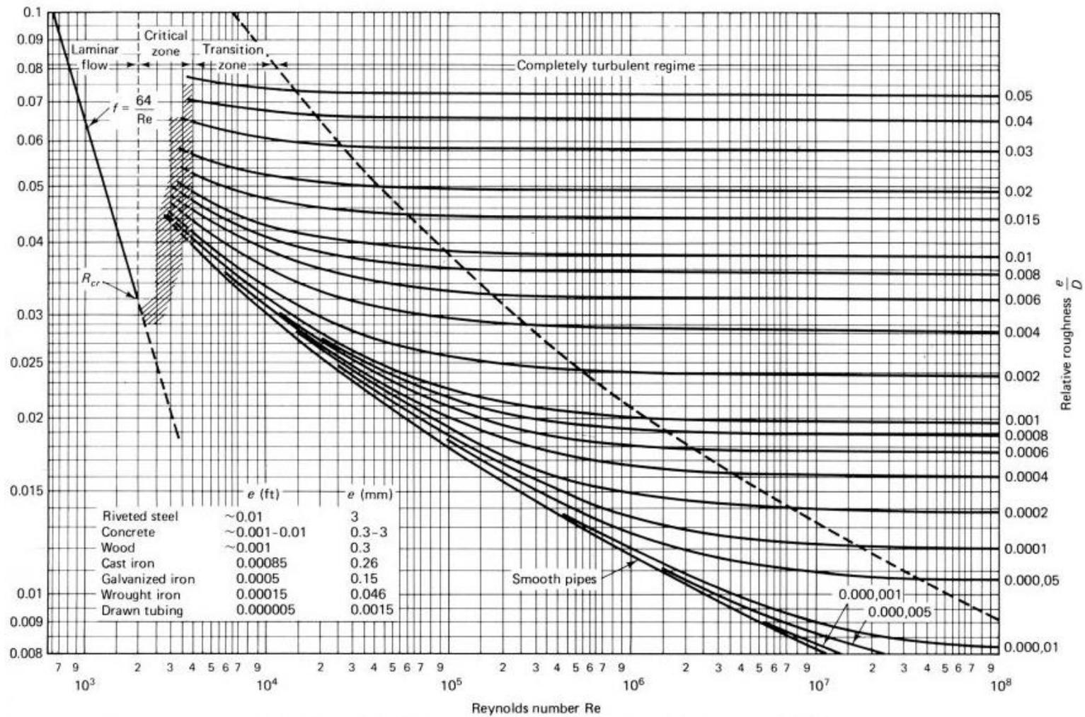
Figure 5.11 Moody diagram (Moody 1944) for selection of d'Arcy friction factor
