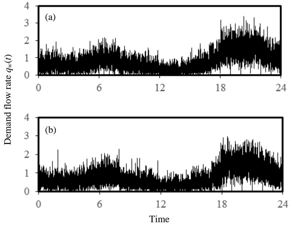
**Figure 5.3 Example demand flow rates for 600 wash basins: (a) maximum daily consumption ( $68.0 \text{ m}^3\text{d}^{-1}$ ); (b) minimum daily consumption ( $64.6 \text{ m}^3\text{d}^{-1}$ )**
