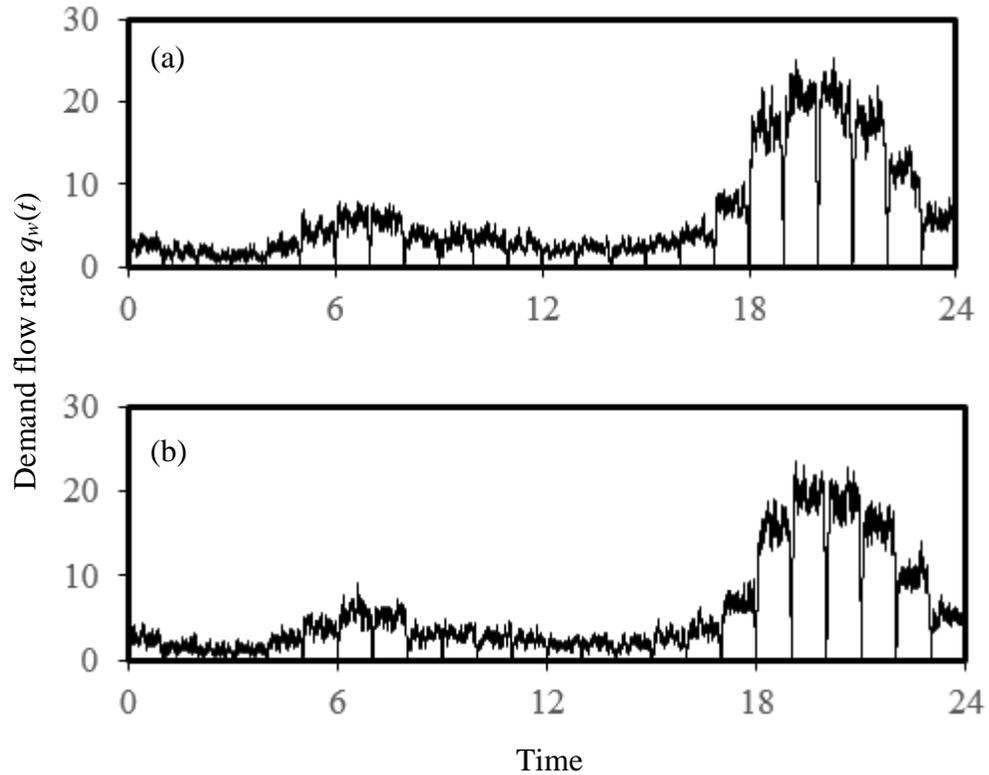
**Figure 5.7 Total demand flow rates for Case B (showerheads are low flow ones, i.e. WELS rated Grade 1 showerheads, while other types of appliances are conventional ones): (a) maximum daily consumption ( $520.7 \text{ m}^3\text{d}^{-1}$ ); (b) minimum daily consumption ( $474.4 \text{ m}^3\text{d}^{-1}$ )**
