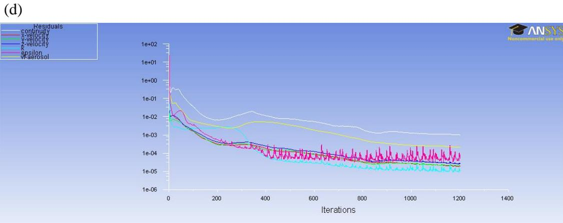
**Figure 6.3 Residuals of numerical calculation for validation: (a) Fan rotational velocity = 1000 rpm; (b) Fan rotational velocity = 2000 rpm; (c) Fan rotational velocity = 3000 rpm; (d) Fan rotational velocity = 4000 rpm**
