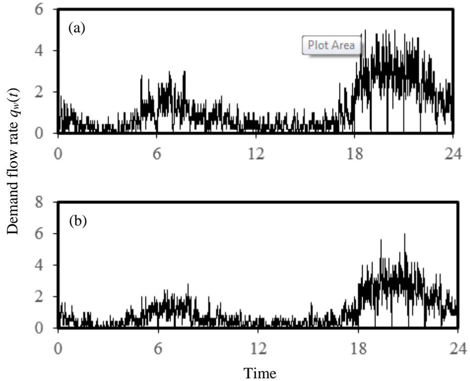
**Figure 5.5 Example demand flow rates for 600 washing machines: (a) maximum daily consumption ( $93.1 \text{ m}^3\text{d}^{-1}$ ); (b) minimum daily consumption ( $82.4 \text{ m}^3\text{d}^{-1}$ )**
