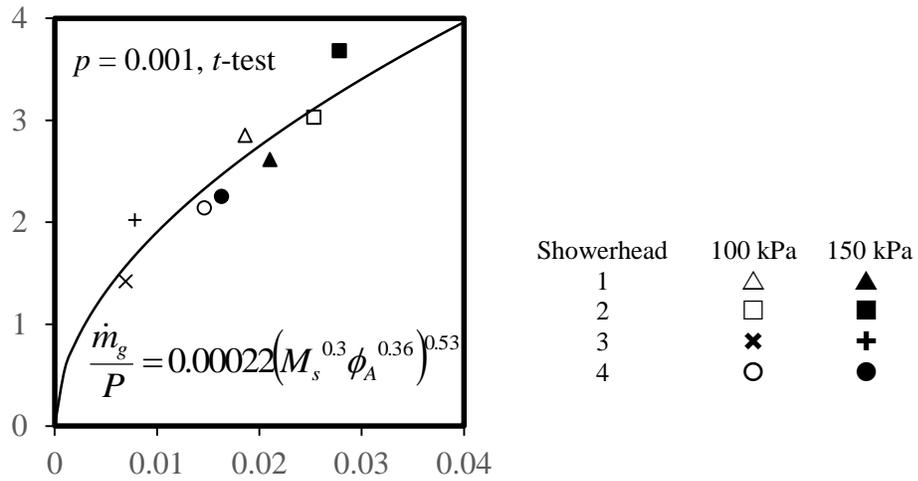
x-axis:  $M_s^{0.3} \phi_A^{0.36}$ ; y-axis: Aerosols mass generation rate  $\dot{m}_g/P$  ( $\times 10^{-10}$   $\text{gs}^{-1} \text{Pa}^{-1}$ )
