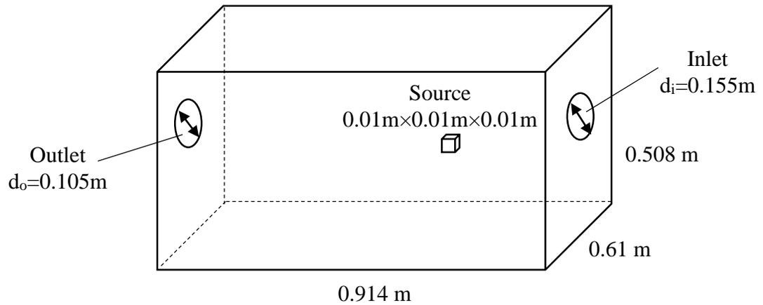
**Figure 3.7 Geometric model set-up for CFD simulations**
