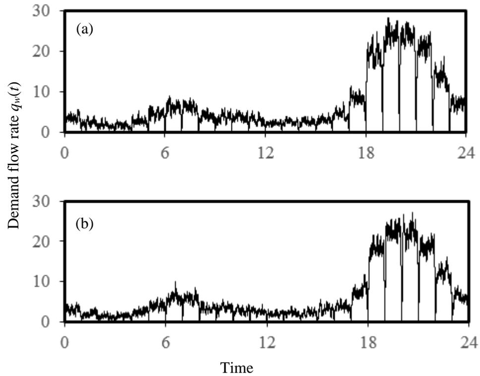
**Figure 5.6 Total demand flow rates for Case A (all appliances are conventional ones): (a) maximum daily consumption ( $590.0 \text{ m}^3\text{d}^{-1}$ ); (b) minimum daily consumption ( $534.8 \text{ m}^3\text{d}^{-1}$ )**
