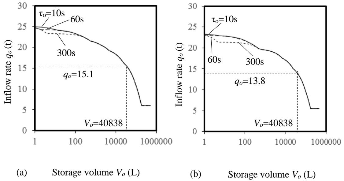
**Figure 5.9 Solutions of inflow rate and storage volume for Case B: (a) for the maximum demand time series in Figure 5.7(a); (b) for the minimum demand time series in Figure 5.7(b)**
