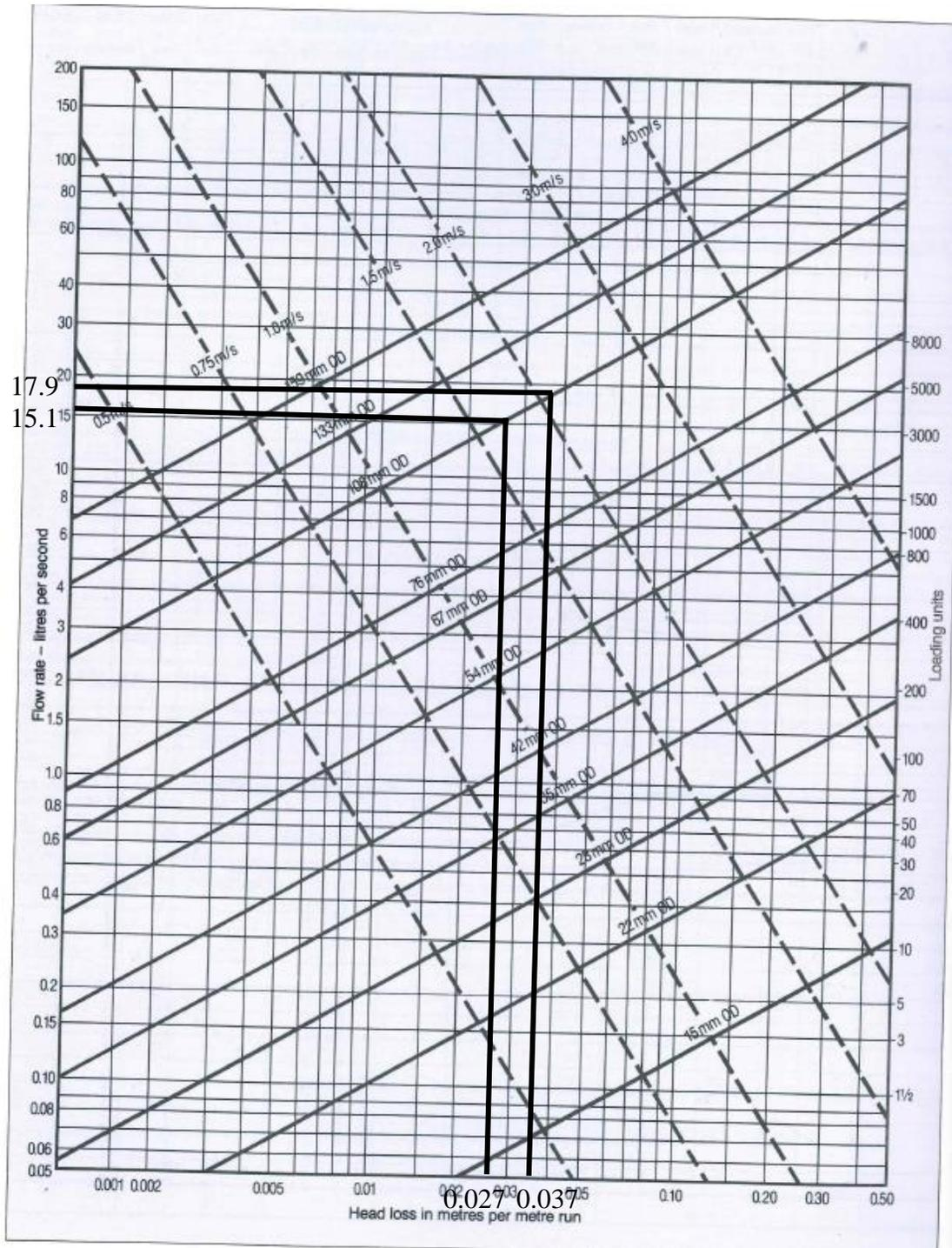
**Figure 5.10 Pipe sizing chart – copper and stainless steel (The Institute of Plumbing 2002)**
