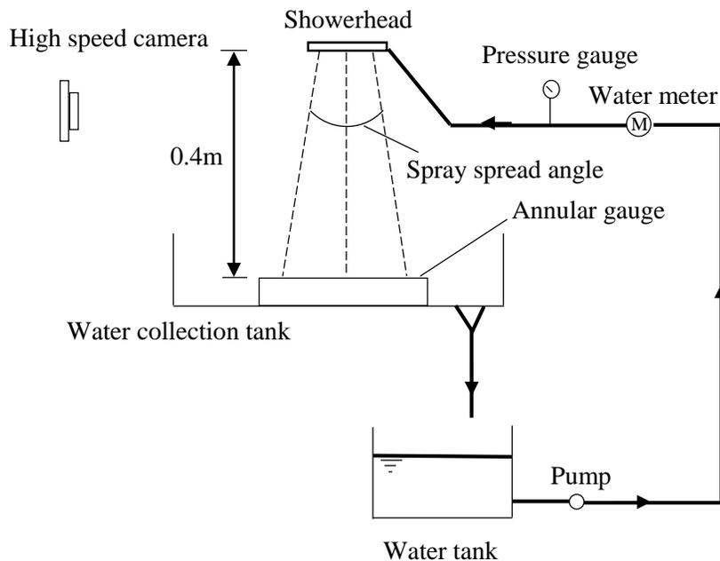
**Figure 3.9 Experimental set-up for measurement of shower spray attributes**
