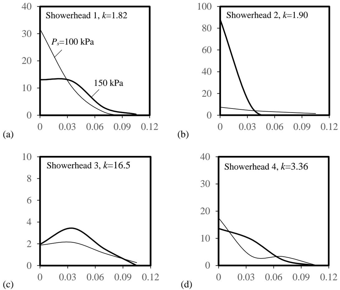
x-axis: Distance from showerhead  $l_s$  (m); y-axis: Mass flux density  $u_{s,l}$  ( $\text{kg s}^{-1} \text{m}^{-2}$ )
