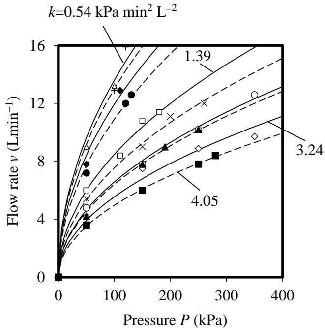
**Figure 4.2 Showerhead resistance factors  $k$  for the 10 surveyed showerheads**
