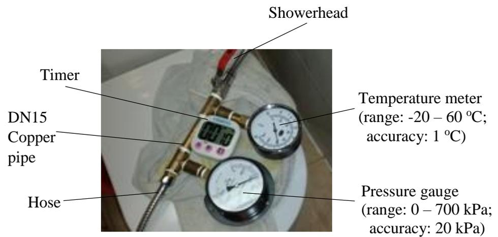
**Figure 3.1 Laboratory-made measurement apparatus**
