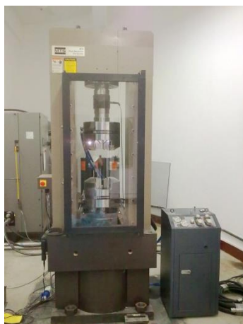
Fig. 2-3 MTS815.02 testing system
