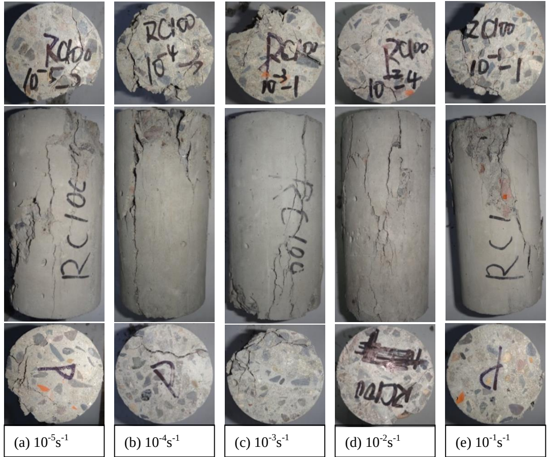
Fig. 3-39 Failure patterns of RAC100 at different strain rates
