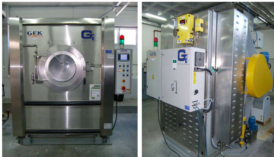
Figure 3.2. G2 ozone machine from Jeanologia [50]
