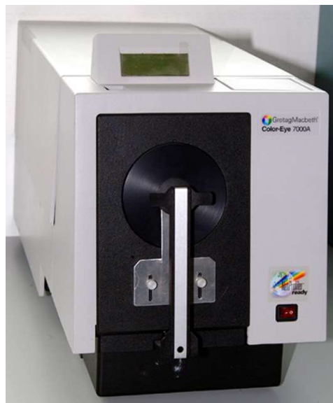
Figure 2.17. Spectrophotometer ColorEye 7000A from GretagMacbeth
