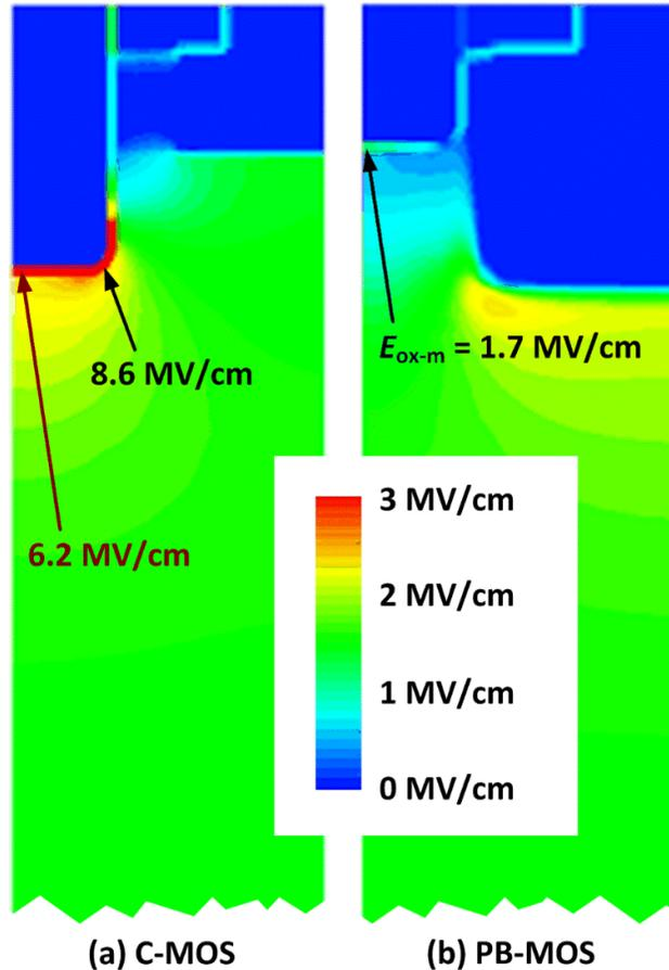
Figure 5-7 OFF-state electric field contours of (a) the C-MOS and (b) the PB-MOS at  $V_{GS} = -5$  V and  $V_{DS} = 1200$  V.
