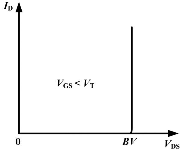
Figure 3-7  $BV$  characteristics of power devices
