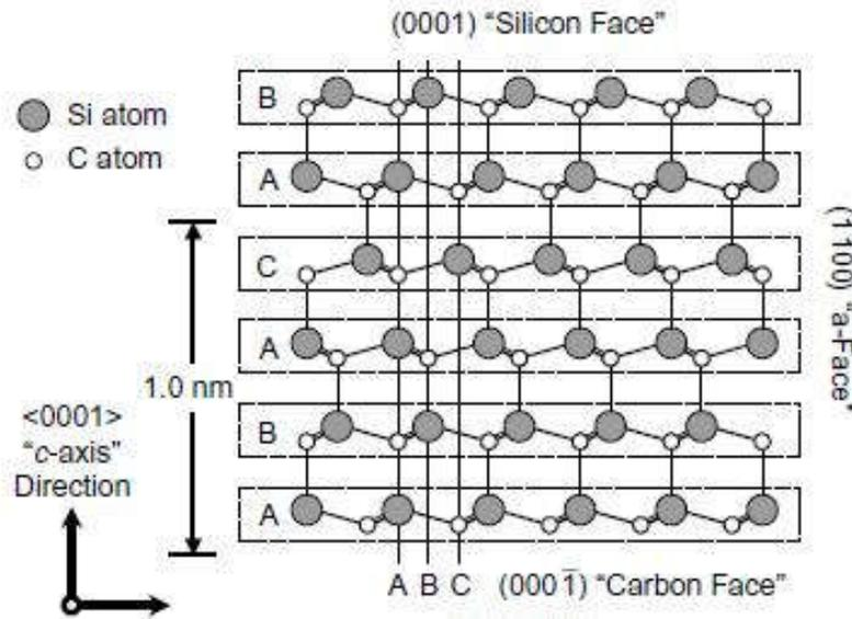
Figure 2-2 Schematic illustration of Si-C bond in a hexagonal SiC polytype.
