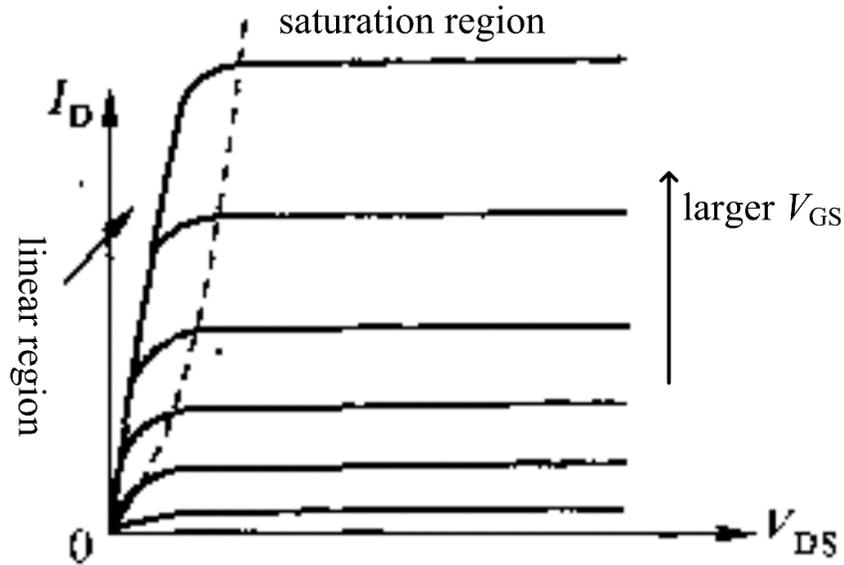
Figure 3-6 Output characteristics of a typical N-channel MOSFET
