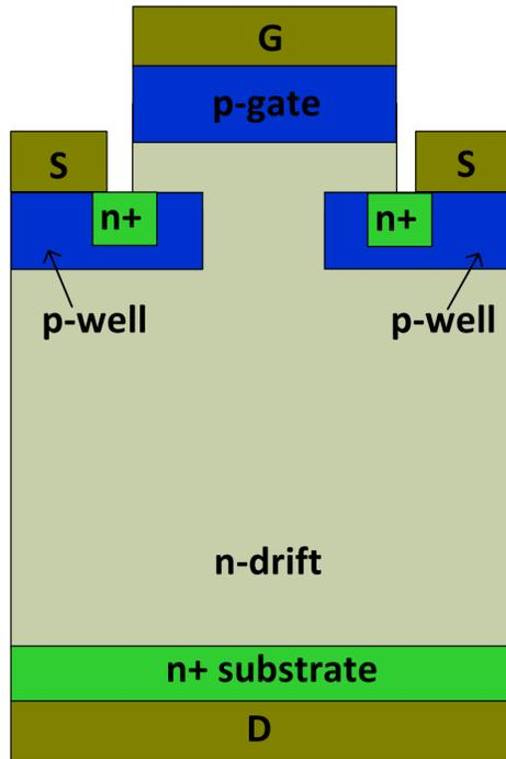
Figure 2-22 Schematic cross-sectional structure of another novel JFET structure.
