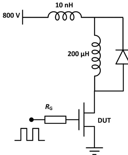
Figure 5-10 Circuit used for the switching tests.
