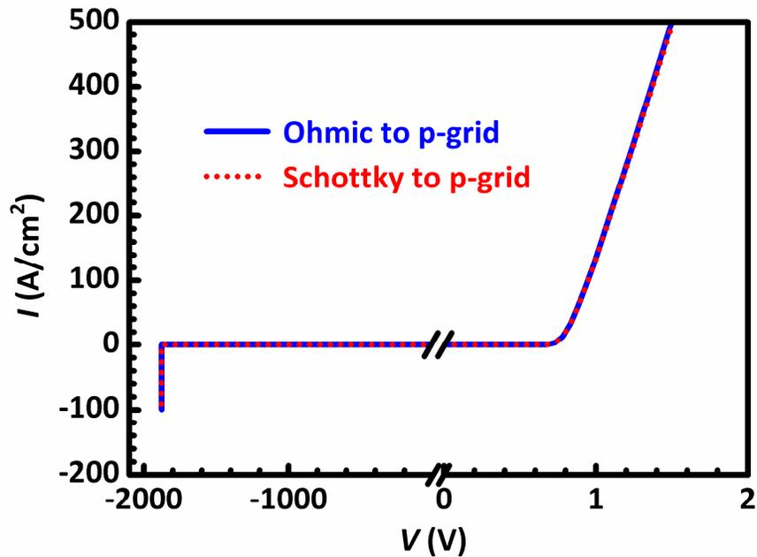
Figure 6-3 Static  $I$ - $V$  characteristics of the SiC JBSs.
