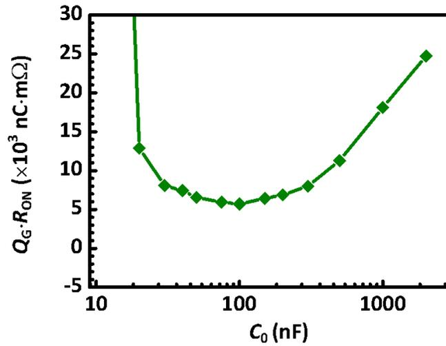
Figure 4-11 The influence of  $C_0$  upon  $Q_G \cdot R_{ON}$ .
