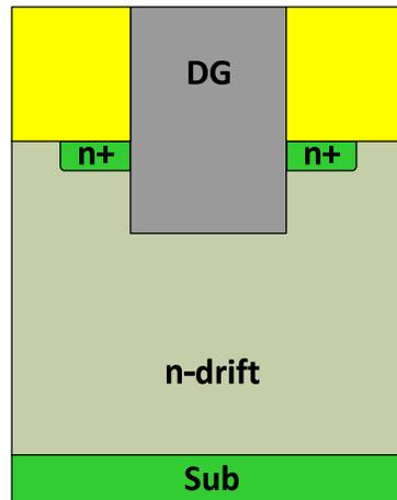
(d) dummy gate by deposition and etch back
