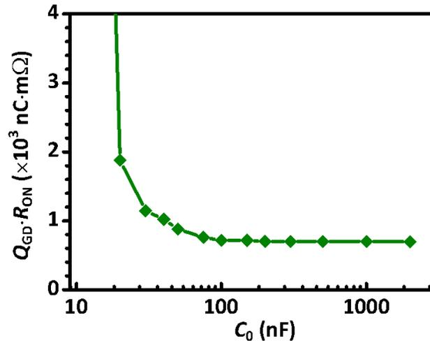
Figure 4-13 The influence of  $C_0$  upon  $Q_{GD} \cdot R_{ON}$ .
