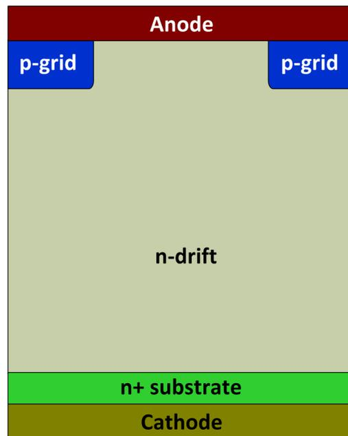
Figure 2-18 Schematic cross-sectional structure of a typical JBS.
