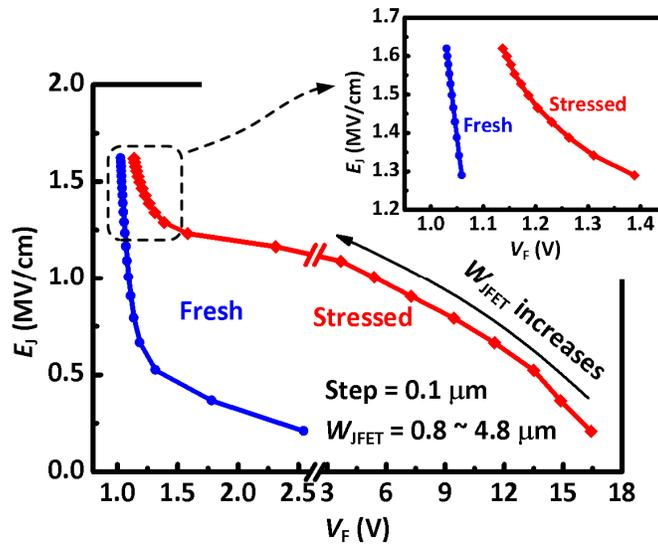
Figure 6-12 The trade-off between junction field  $E_J$  and the forward voltage  $V_F$ . The distance between p-grids  $W_{JFET}$  is varied.
