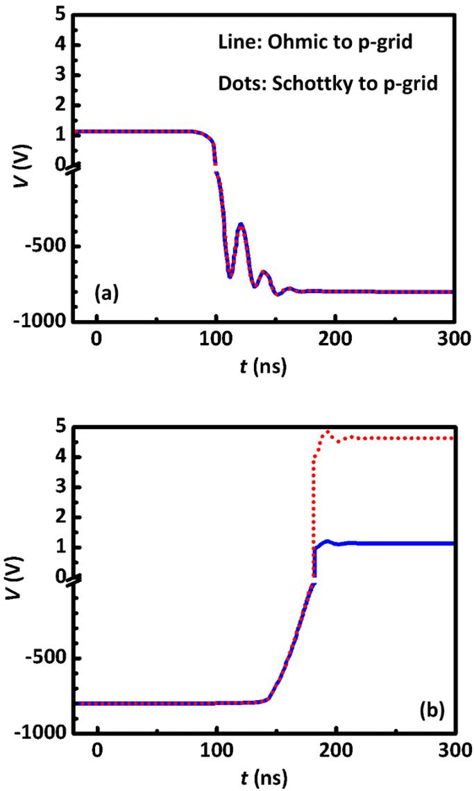
Figure 6-7 The voltage of JBS at (a) the turn-off transient of the SiC JBS by switching on the MOSFET, (b) the turn-on transient of the SiC JBS by switching off the MOSFET.
