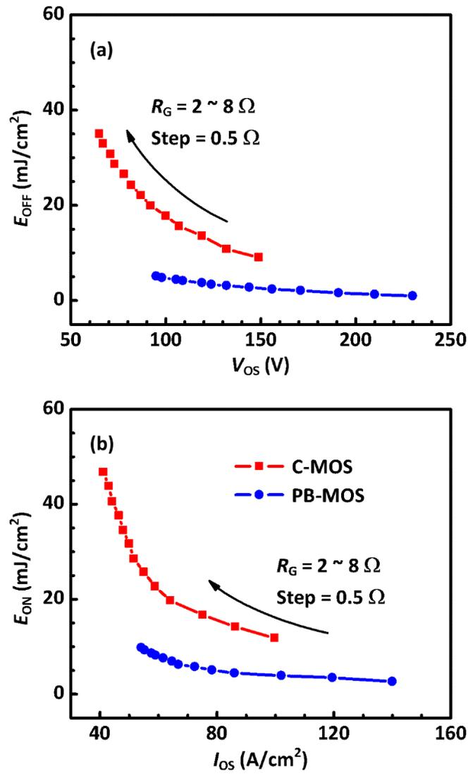
Figure 5-12 (a) The trade-off curve between the voltage overshoot ( $V_{OS}$ ) and the turn-off energy loss ( $E_{OFF}$ ) of the studied MOSFETs, and (b) the trade-off curve between the current overshoot ( $I_{OS}$ ) and the turn-on energy loss ( $E_{ON}$ ), as  $R_G$  is varied.
