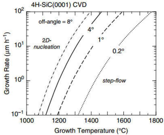
Figure 2-10 The influence of off-axis angles on HTCVD growth of 4H-SiC (0001) at different temperatures.
