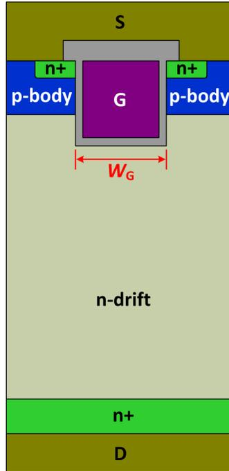
Figure 5-2 Schematic cross-sectional structure of the conventional trench MOSFET (C-MOS). The width of the gate trench is  $W_G$ .
