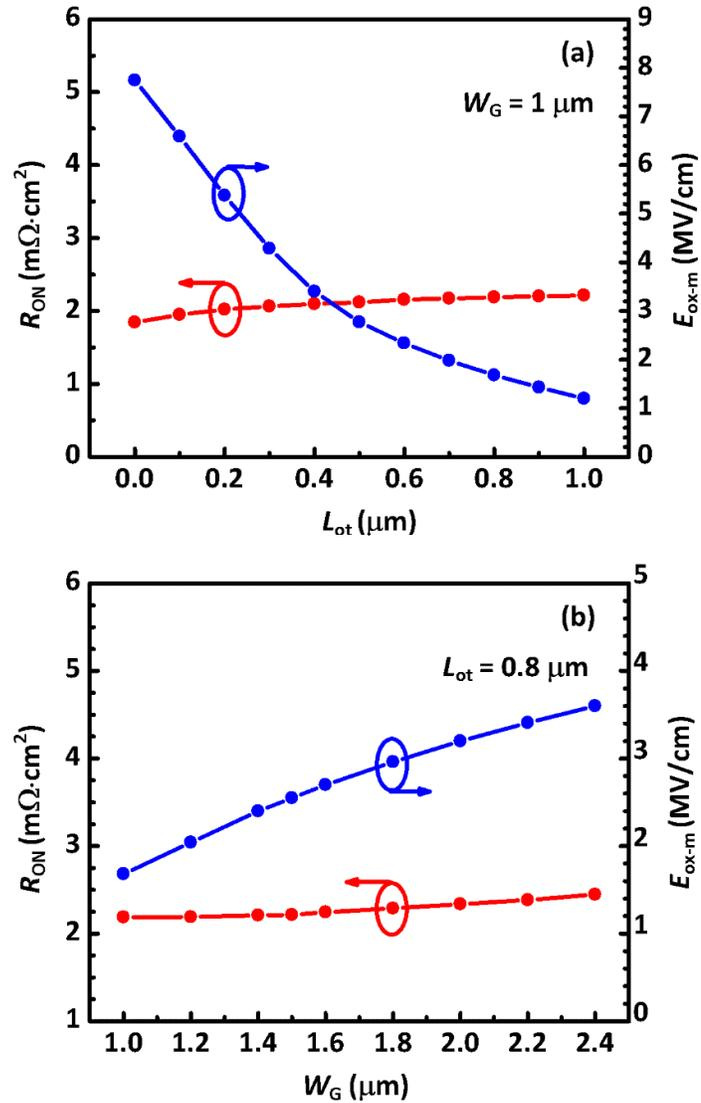
Figure 5-5 The influence of (a)  $L_{ot}$  and (b)  $W_G$  upon  $R_{ON}$  and  $E_{ox-m}$  in the PB-MOS.  $E_{ox-m}$  is defined as the maximum oxide field at  $V_{GS} = -5$  V and  $V_{DS} = 1200$  V.  $W_G = 1$   $\mu$ m and  $L_{ot} = 0.8$   $\mu$ m are chosen for the PB-MOS for comparisons with the C-MOS in the rest part of the study.
