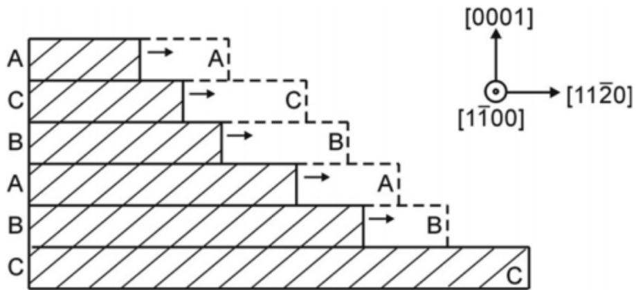
Figure 2-9 Schematic illustration of single crystal type growth of step-controlled epitaxy.
