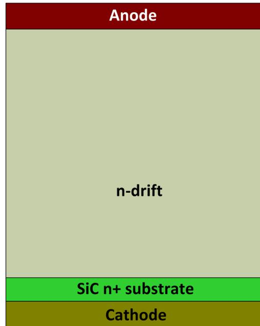
Figure 2-16 Schematic cross-sectional structure of a typical SBD.
