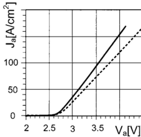
Figure 2-15 Forward  $I$ - $V$  characteristic before (solid) and after (dashed) continuous converter operation [80].
