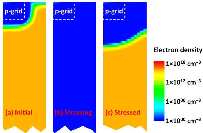
Figure 6-8 The electron distribution in the SiC JBS with a Schottky contact to the p-grid. (a) The initial state with the device zero biased. (b) The state with an 800-V reverse bias stress. (c) The state immediately following the stressing period, with the device zero biased. The time used to turn the device from the stressing state in (b) to the zero-biasing state in (c) is 1  $\mu\text{s}$ .
