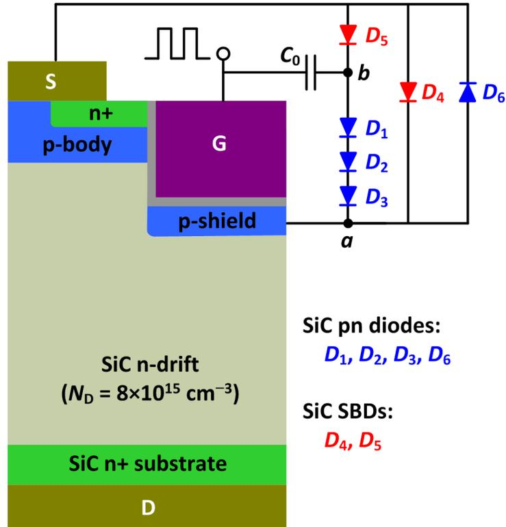
Figure 4-2 Schematic structure of the proposed SBS-MOS. In this study, SiC pn junction diodes are used for  $D_1$ ,  $D_2$ ,  $D_3$ , and  $D_6$ , while SiC SBDs are used for  $D_4$  and  $D_5$ .  $C_0$  is 100 nF, except when other values are specified.
