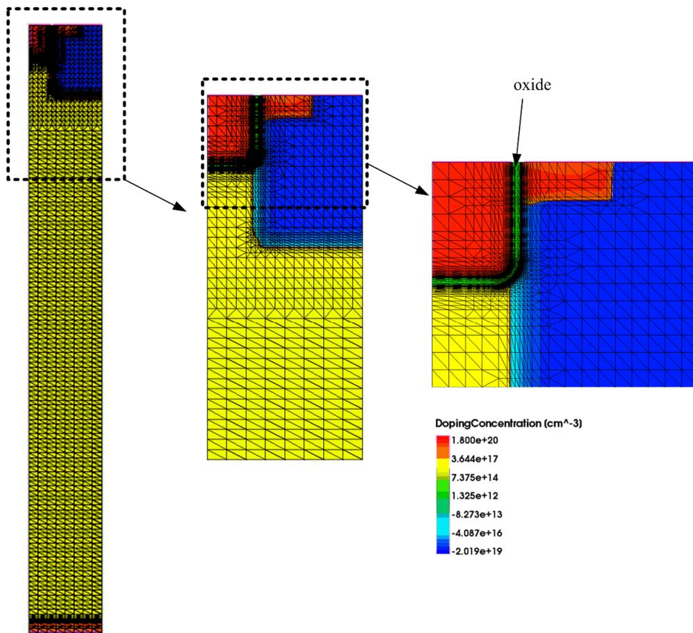
Figure 3-2 Mesh design in a SiC MOSFET.
