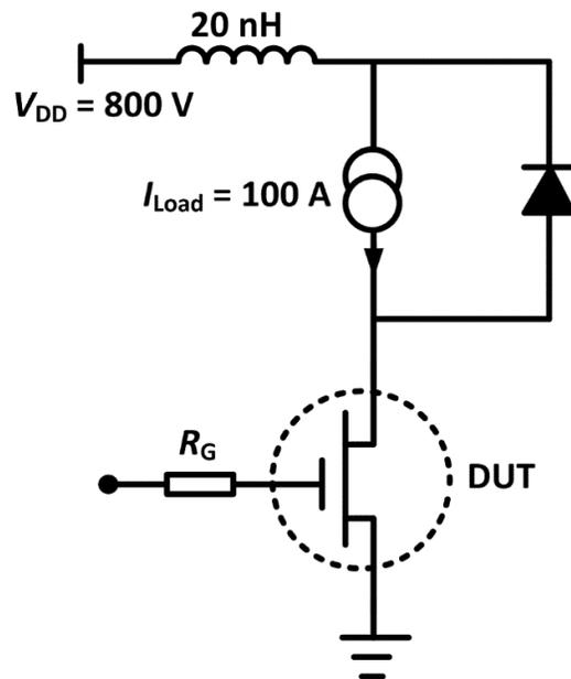
Figure 4-4 Test circuit for switching characteristics of the devices under study. A supply voltage of 800 V and a load current of 100 A are used. The area for the device under test is 1 cm<sup>2</sup>. A SiC junction barrier Schottky diode is used to provide a freewheeling path.
