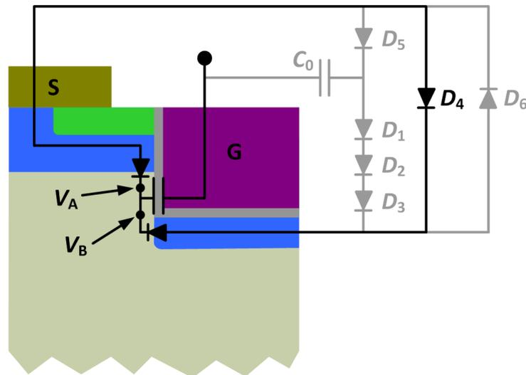
Figure 4-8 Illustration of the discharging current path in the last stage of turn-off transient for the SBS-MOS.
