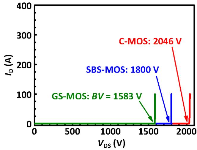
Figure 4-18 OFF-state breakdown characteristics of the studied devices.
