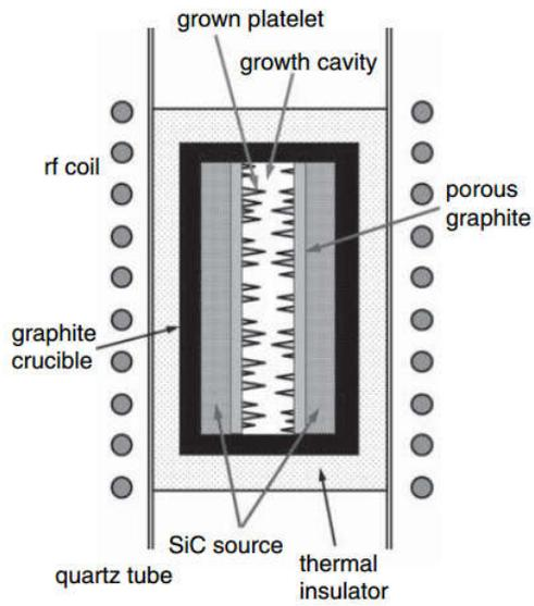
Figure 2-5 A schematic illustration of SiC bulk growth with Lely method.
