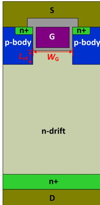
Figure 5-3 Schematic cross-sectional structure of the proposed protruded p-bodies trench MOSFET (PB-MOS). The width of the gate trench is  $W_G$ , and the p-bodies protrude beyond the gate trench by  $L_{ot}$ .
