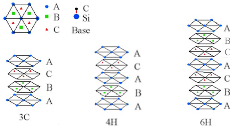
Figure 2-1 The stacking sequence of 3C, 4H and 6H polytypes of SiC.
