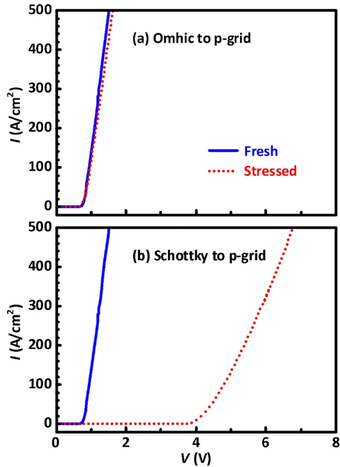
Figure 6-11 The static  $I$ - $V$  characteristics of (a) the SiC JBS with an Ohmic contact to the p-grid, and (b) that with a Schottky contact to the p-grid.
