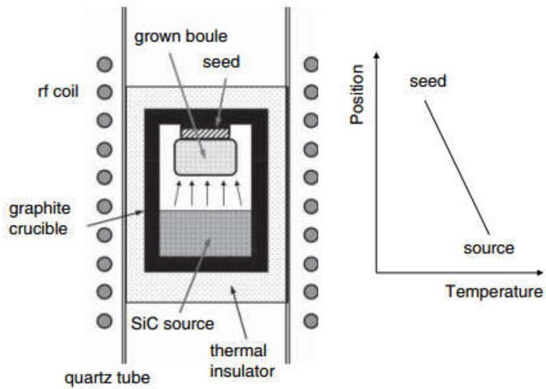
Figure 2-6 Schematic illustration of SiC bulk growth with the modified Lely method and approximate temperature profile.
