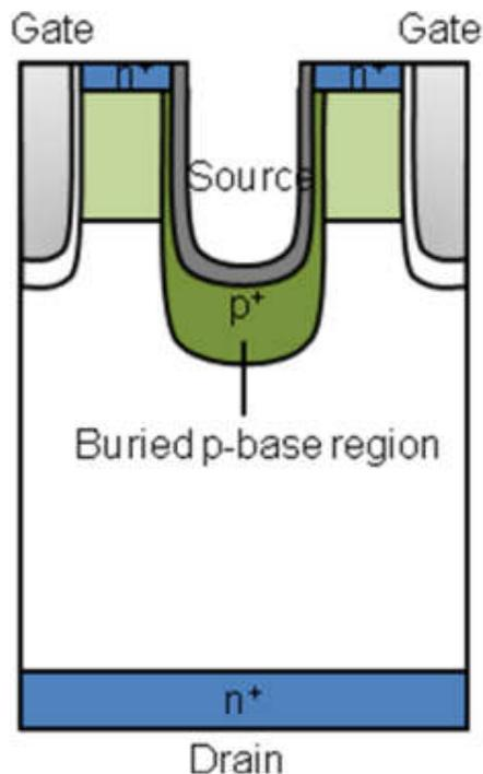
Figure 5-1 The cross-sectional structure of double trench SiC MOSFET.
