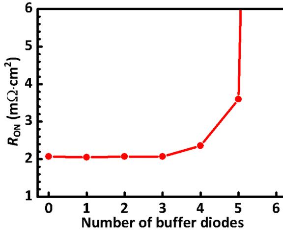
Figure 4-14 The influence of the number of buffer diodes upon  $R_{ON}$ .
