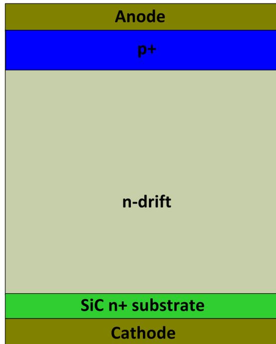
Figure 2-14 Schematic cross-sectional structure of a typical PiN diode.
