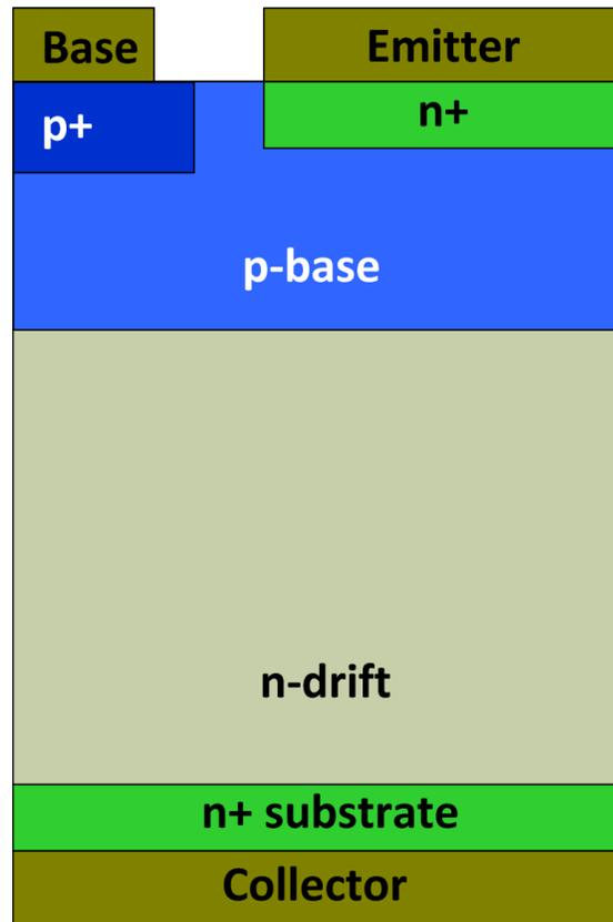
Figure 2-19 Schematic cross-sectional structure of a typical structure of SiC BJT.
