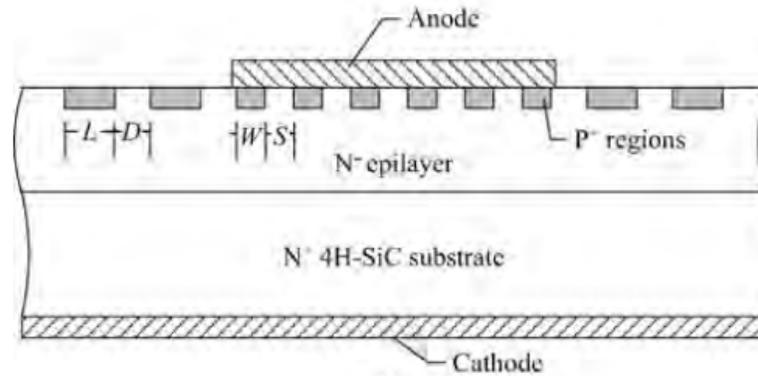
Figure 6-1 SiC Schottky diode with a Schottky electrode instead of Ohmic electrode as the Anode electrode [69].
