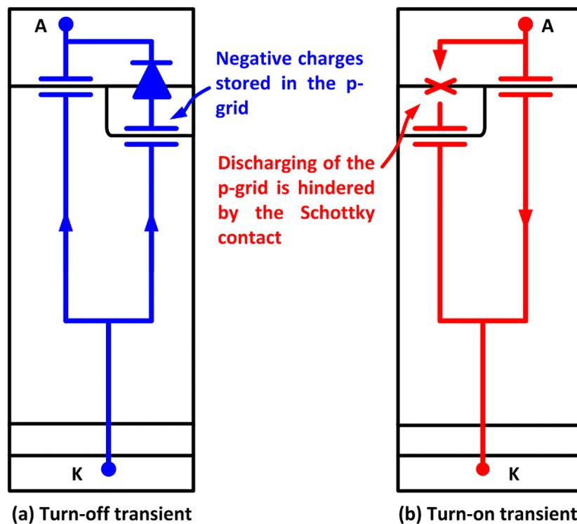
Figure 6-10 Illustration of the charge storing mechanism of the SiC JBS with Schottky contact to p-grid.
