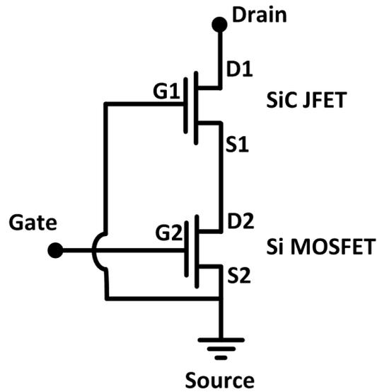
Figure 2-24 A cascode configuration of SiC JFET and Si MOSFET for power applications.
