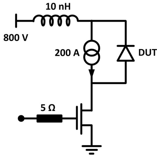
Figure 6-5 The test circuit to test the switching characteristics of the SiC JBS. A SiC MOSFET is used as the switch. The driving signal is switched between  $-5$  V and  $15$  V to set the MOSFET to OFF- and ON-state, respectively.
