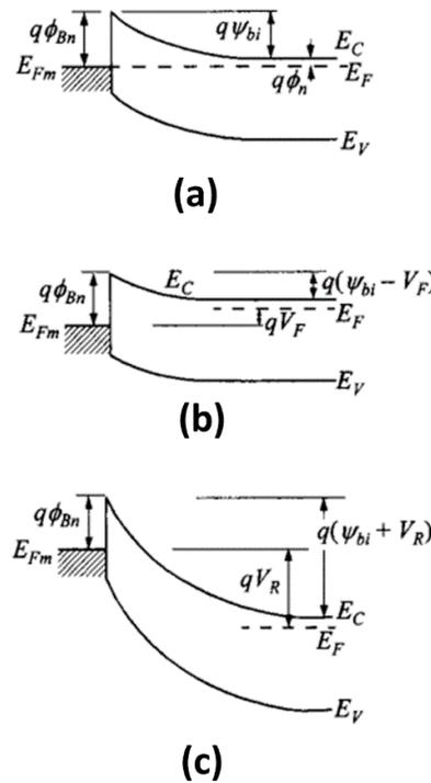
Figure 2-17 Energy band diagrams of metal on n-type under (a) zero bias, (b) forward bias, and (c) reverse bias.
