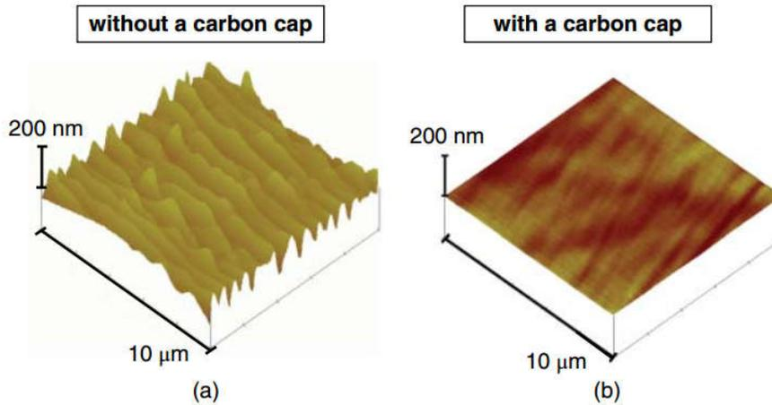
Figure 2-13 AFM images of SiC surfaces after annealing at 1800 °C (a) without a carbon cap, (b) with a carbon cap.
