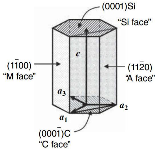
Figure 2-3 Definition of several major faces in the hexagonal crystallographic notation of SiC crystal.
