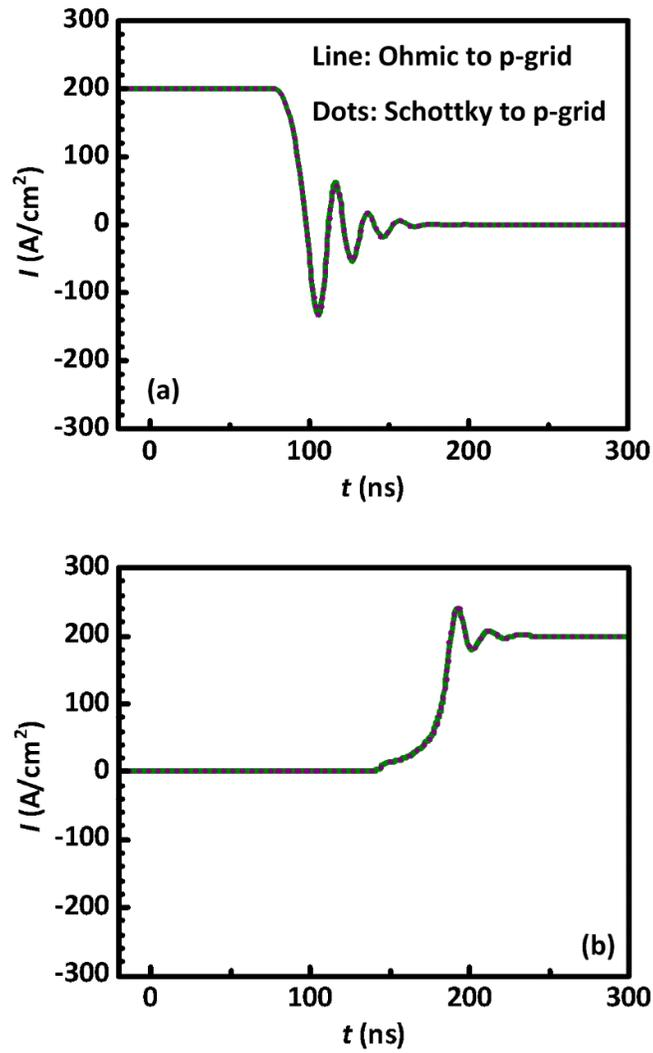
Figure 6-6 The current of JBS at (a) the turn-off transient of the SiC JBS by switching on the MOSFET, (b) the turn-on transient of the SiC JBS by switching off the MOSFET.
