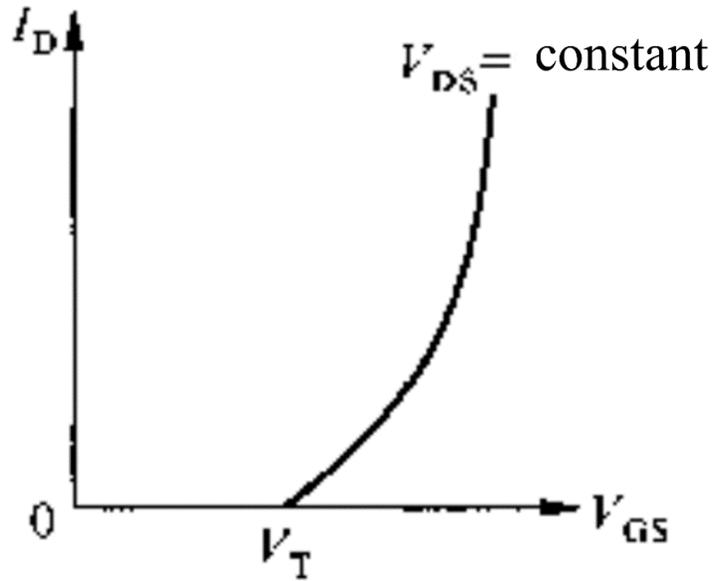
Figure 3-5 Transfer characteristics of an N-channel MOSFET.
