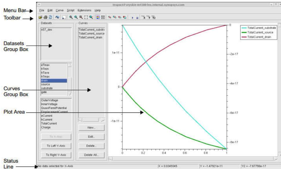
Figure 3-4 The main window of Inspect.
