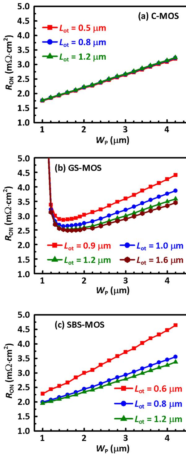
Figure 4-16 Influences of  $W_p$  on  $R_{ON}$  of (a) C-MOS, (b) GS-MOS and (c) SBS-MOS.
