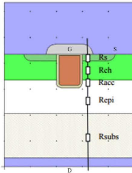
Figure 3-8 Detailed components in  $R_{ON}$  of a trench MOSFET.
