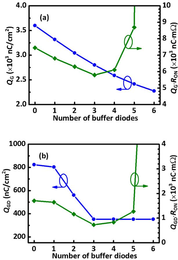
Figure 4-15 The influence of the number of buffer diodes upon (a)  $Q_G$  and  $Q_G \cdot R_{ON}$ , and (b)  $Q_{GD}$  and  $Q_{GD} \cdot R_{ON}$ . The buffer diodes are those between node a and b. As in Figure 4-1(c), three buffer diodes  $D_1$ - $D_3$  are illustrated.
