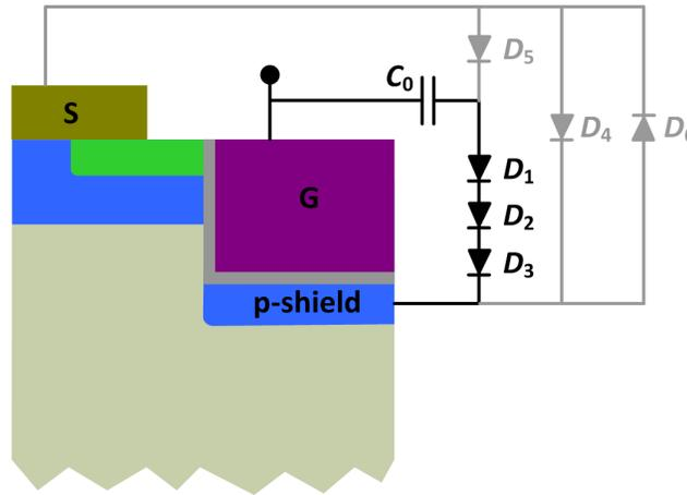
Figure 4-6 Illustration of the charging current path in the first stage of turn-on transient for the SBS-MOS.
