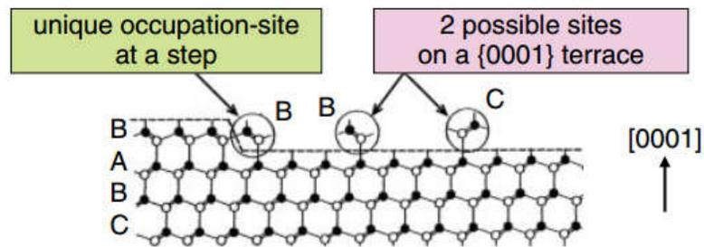
Figure 2-8 Schematic illustration of bond configuration on-axis and at a step in SiC growth.
