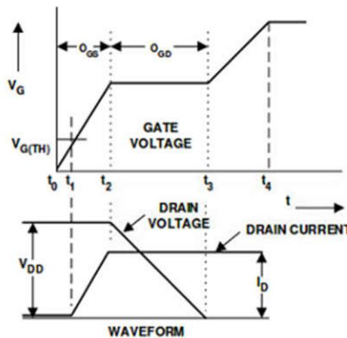
Figure 3-10 Waveforms of  $V_G$ ,  $I_D$ , and  $V_{DD}$  at turn-on process of MOSFET
