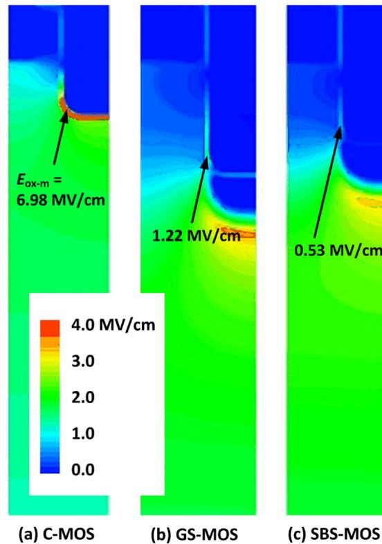
Figure 4-19 Electric field contours at  $V_{\text{DS}} = 1200$  V in the half cell of (a) C-MOS, (b) GS-MOS and (c) SBS-MOS.
