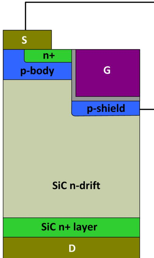
Figure 2-26 Trench SiC MOS with grounded p-shield (GS-MOS).
