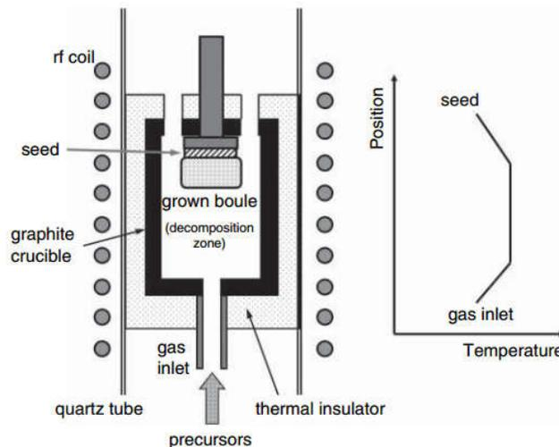
Figure 2-7 Schematic illustration of HTCVD and approximate temperature profile.
