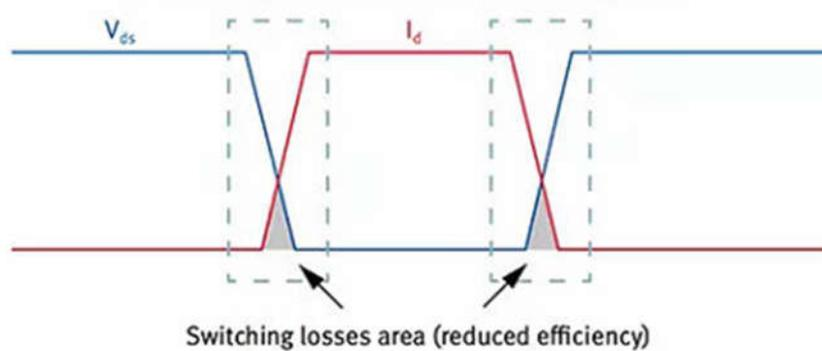
Figure 3-9 Drain current and drain-to-source voltage waveforms of the switching of a MOSFET.
