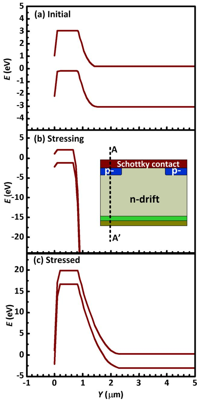
Figure 6-9 Simulated energy band along AA' in the inset in (b) under the three states of Figure 6-8 in the SiC JBS with Schottky contact to p-grid. The interface between the Schottky contact and the semiconductor is set as 0  $\mu\text{m}$ .
