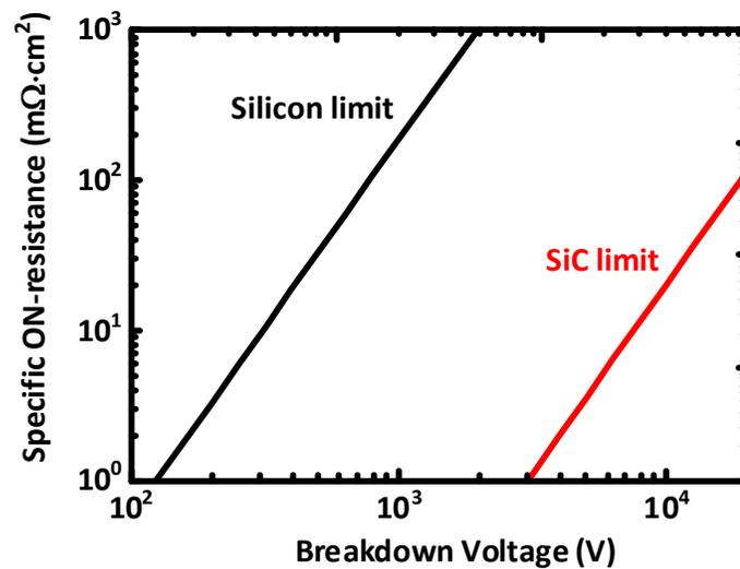
Figure 1-2 Material limits for unipolar power devices
