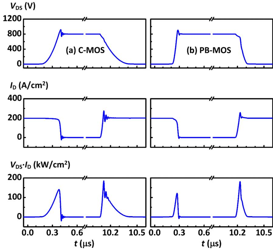
Figure 5-11 Switching waveforms of (a) the C-MOS and (b) the PB-MOS. The circuit in Figure 5-10 is used for the switching test, with  $R_G = 3 \Omega$  for the C-MOS and  $7 \Omega$  for the PB-MOS.
