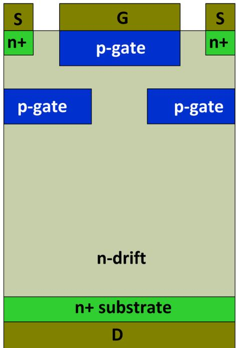
Figure 2-21 Schematic cross-sectional structure of an improved JFET structure.
