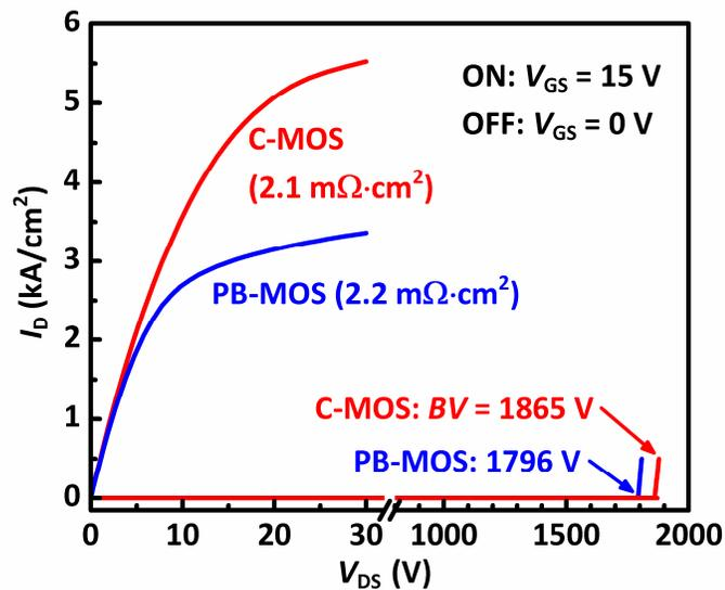
Figure 5-6 The  $I$ - $V$  characteristics of the C-MOS and the PB-MOS.
