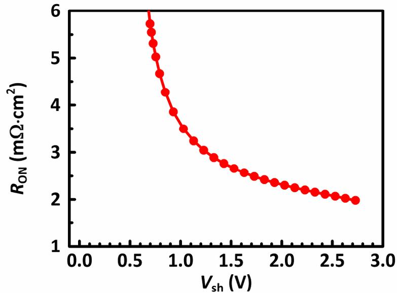
Figure 4-3 Influences of the voltage of the p-shield  $V_{sh}$  upon  $R_{ON}$  of a SiC trench MOSFET with a p-shield.
