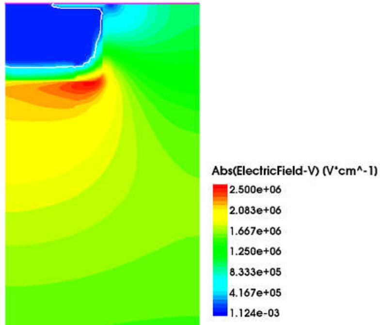
Figure 6-4 Electric field at 1200 V of the studied SiC JBS.
