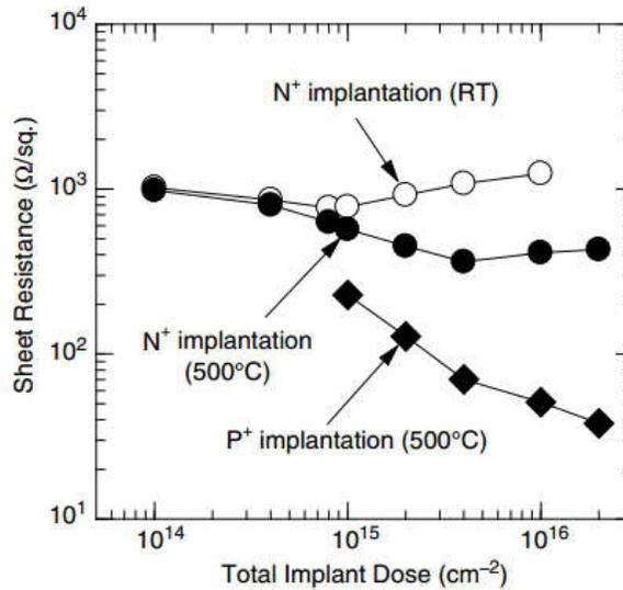
Figure 2-12 Sheet resistance vs. total implant dose for N<sup>+</sup> and P<sup>+</sup>-implanted 4H-SiC under room temperature and 500 °C.
