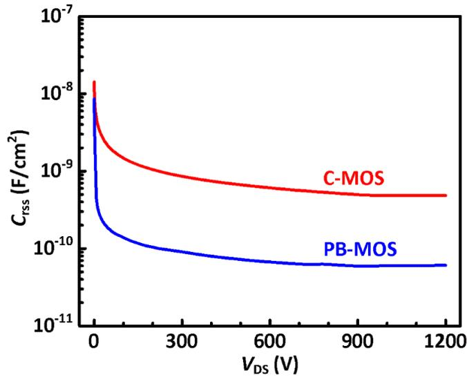
Figure 5-8 Reverse transfer capacitance ( $C_{\text{rss}}$ ) of the C-MOS and the PB-MOS with  $V_{\text{GS}} = 0$  V.
