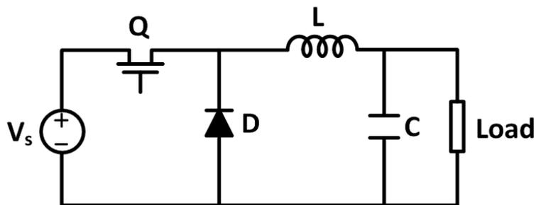
Figure 1-1 The circuit diagram of a buck converter.
