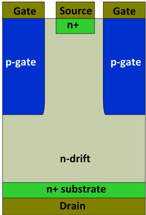
Figure 2-20 Schematic cross-sectional structure of a typical JFET.
