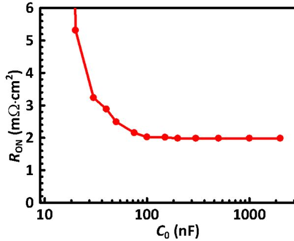
Figure 4-9 The influences of  $C_0$  upon (a)  $R_{ON}$ , (b)  $Q_G$  and  $Q_G \cdot R_{ON}$ , and (c)  $Q_{GD}$  and  $Q_{GD} \cdot R_{ON}$ .
