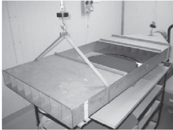
Figure 2.1 Guarded hot plate with a circular sample (Laing et al., 2007)
