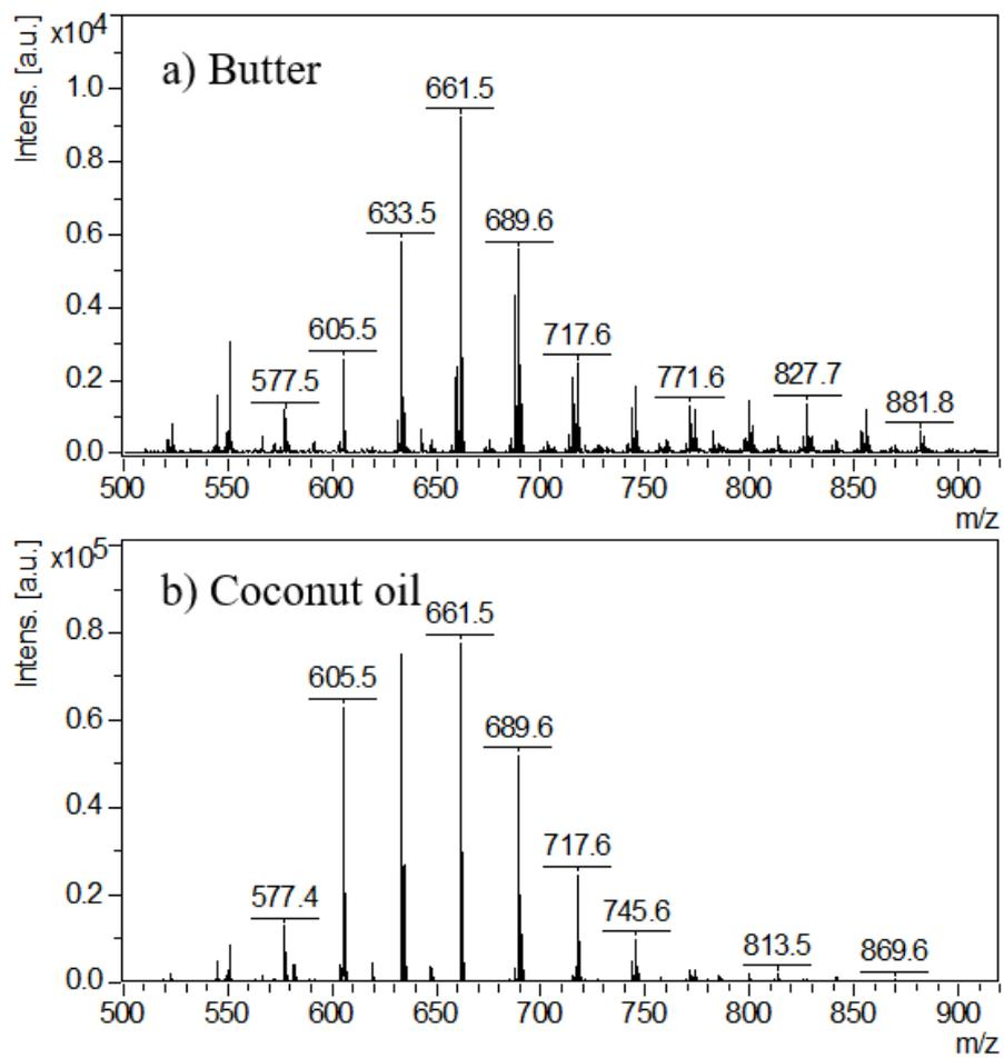
**Figure 4-13.** The mass spectra for the TAG regions of (a) butter and (b) coconut oil.
