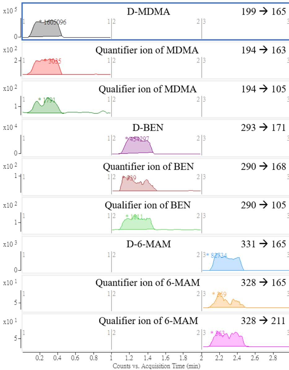
**Figure 3-15.** MRM signals for the detection of MDMA, BEN and 6-MAM in Medichem Basis-line U sample using SPME-ESI-MS.
