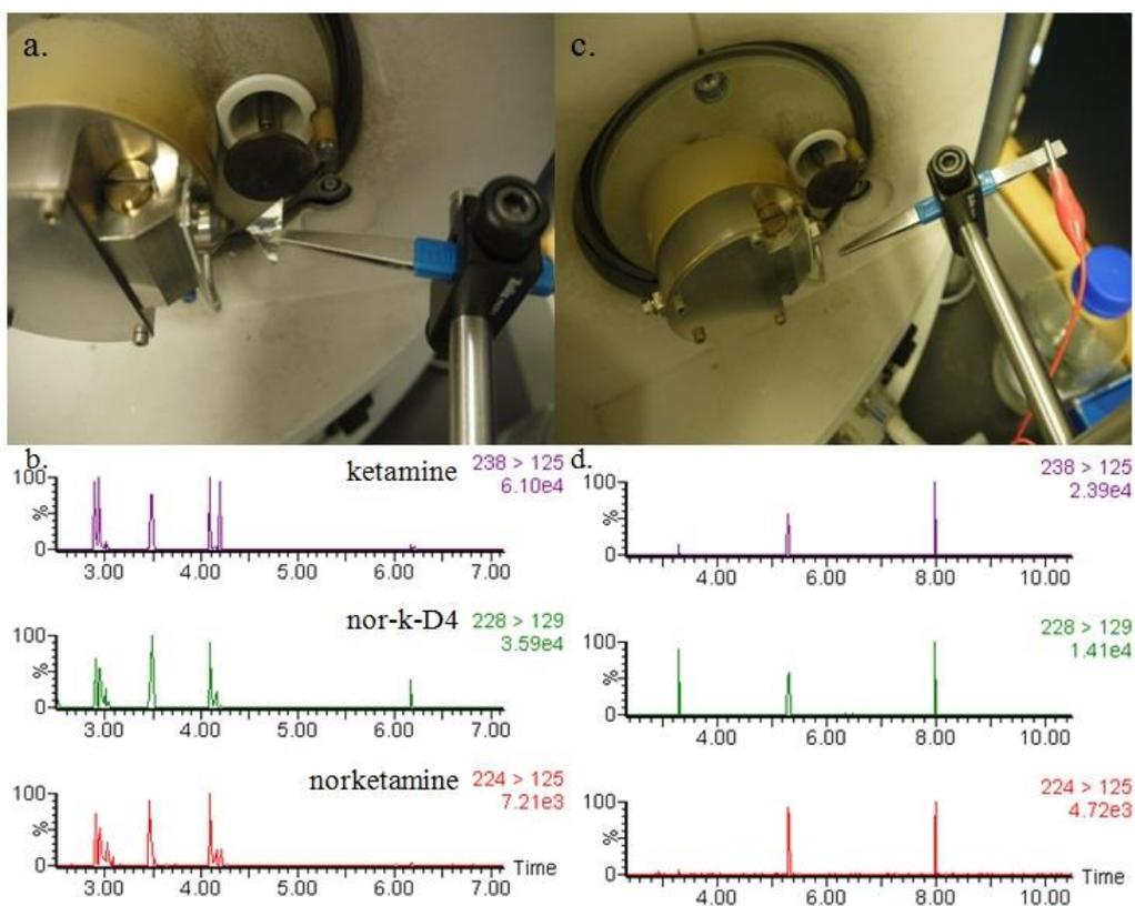
**Figure 2-4.** (a) and (c) Electro spray ionization using aluminum foil and stainless-steel needle, respectively; (b) and (d) chromatogram showing the ion signal generated by aluminum foils and stainless-steel needles, respectively.
