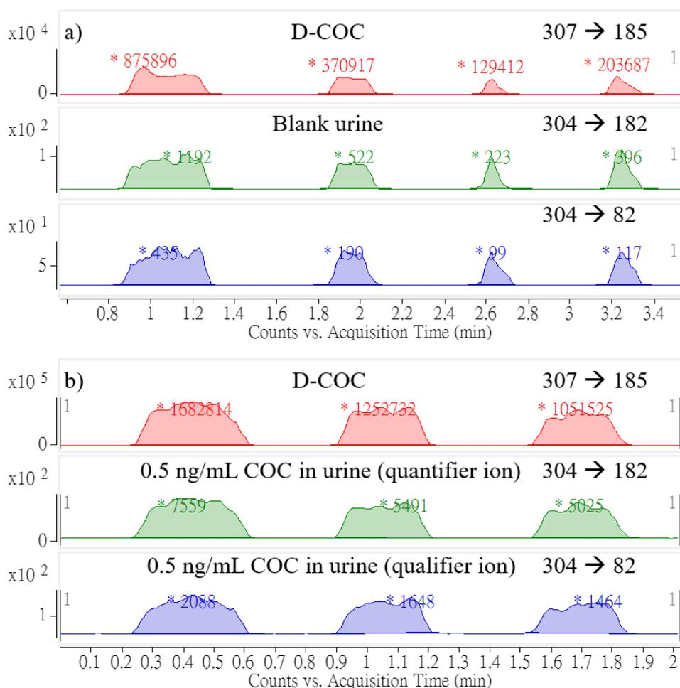
**Figure 3-14.** MRM results for the detection of cocaine of (a) blank urine and (b) 0.5 ng/mL of cocaine in urine using SPME-ESI-MS.
