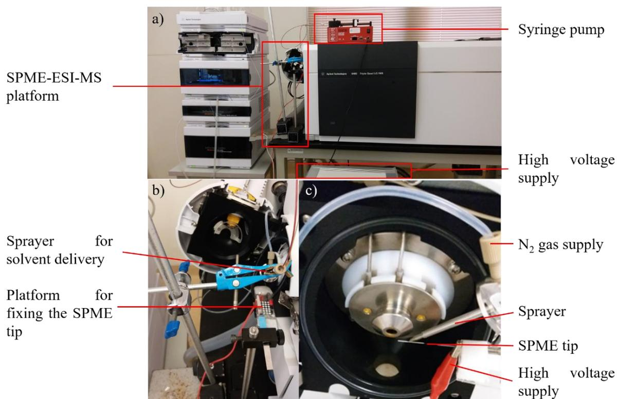
**Figure 3-1.** (a) The setup of SPME-ESI-MS on an Agilent 6460 triple quadrupole mass spectrometer. (b) Close-up of the platform placed in front of the mass spectrometer for SPME-ESI-MS analysis and (c) Close-up of a SPME tip mounted onto the platform for SPME-ESI-MS analysis.
