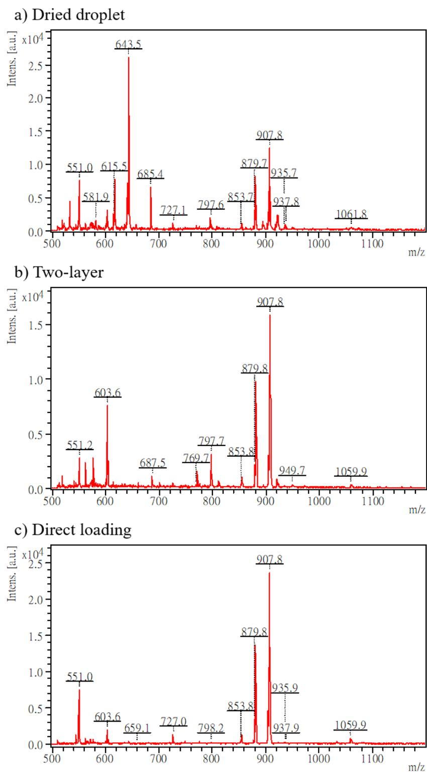
**Figure 4-2.** MALDI-MS spectra of an olive oil sample obtained by (a) dried-droplet method, (b) two-layer method and (c) direct sample loading method
