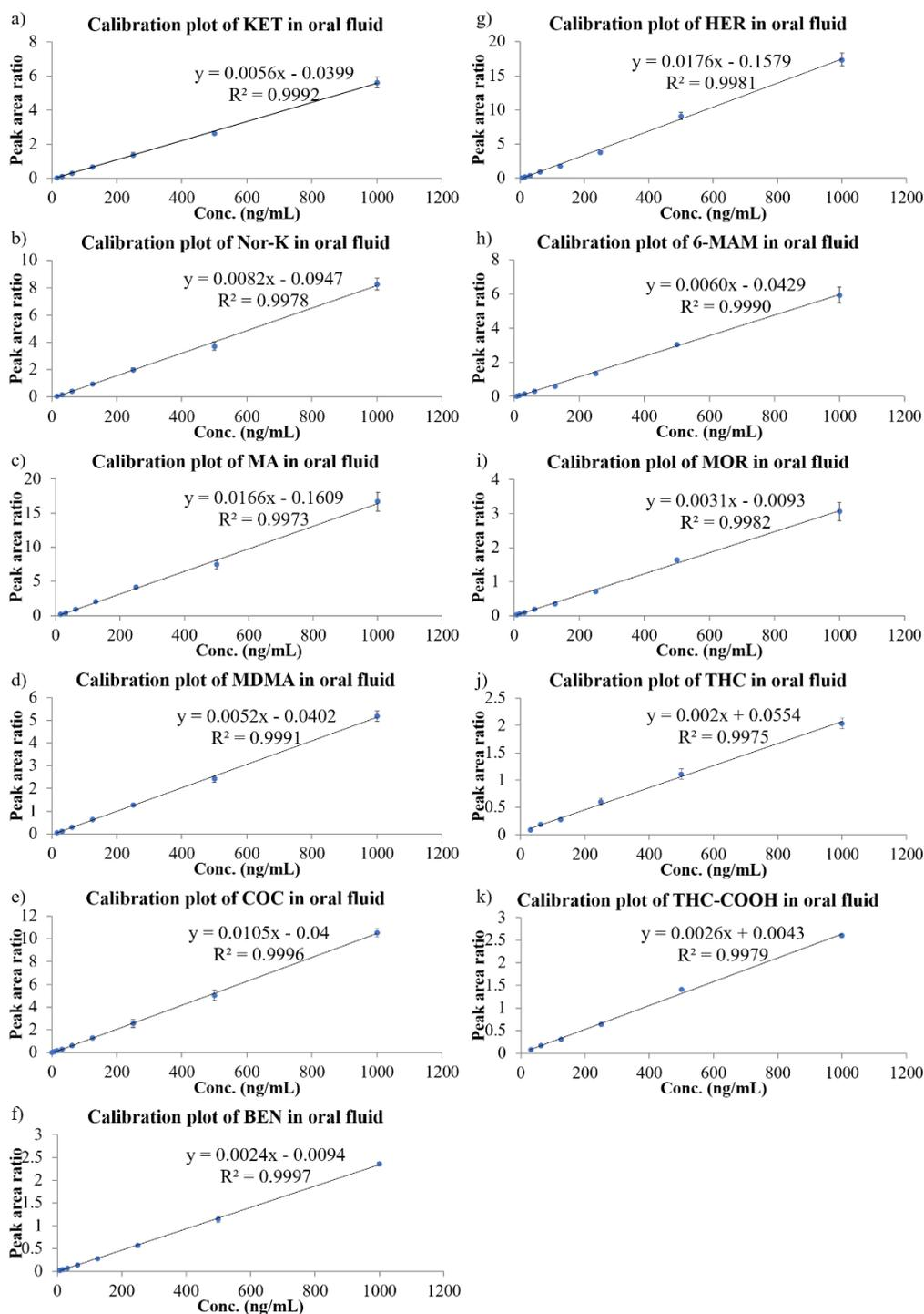
**Figure 3-13.** Calibration plots for the quantitation of (a) ketamine, (b) nor-ketamine, (c) methamphetamine, (d) MDMA, (e) cocaine, (f) benzoylecgonine, (g) heroin, (f) 6-monoacetylmorphine, (i) morphine, (j) THC and (k) THC-COOH in oral fluid.
