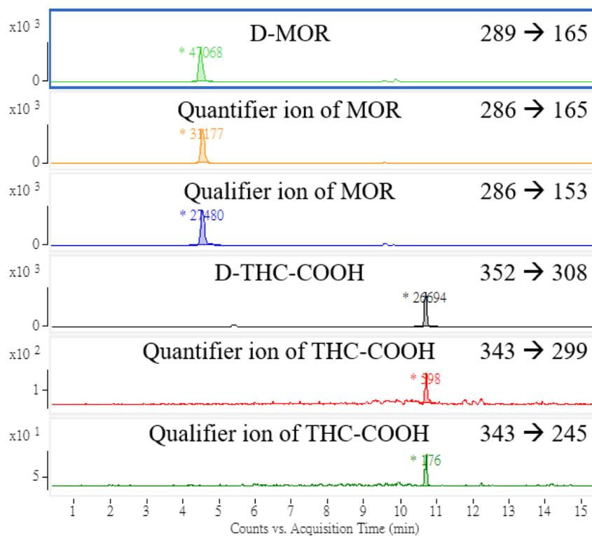
**Figure 3-18.** The LC-MRM results for the detection and quantitation of MOR and THC-COOH in Medichem WDT confirm U +25% sample using C18 SPME tip for the extraction. Negative ionization mode was used for the analysis of THC-COOH.
