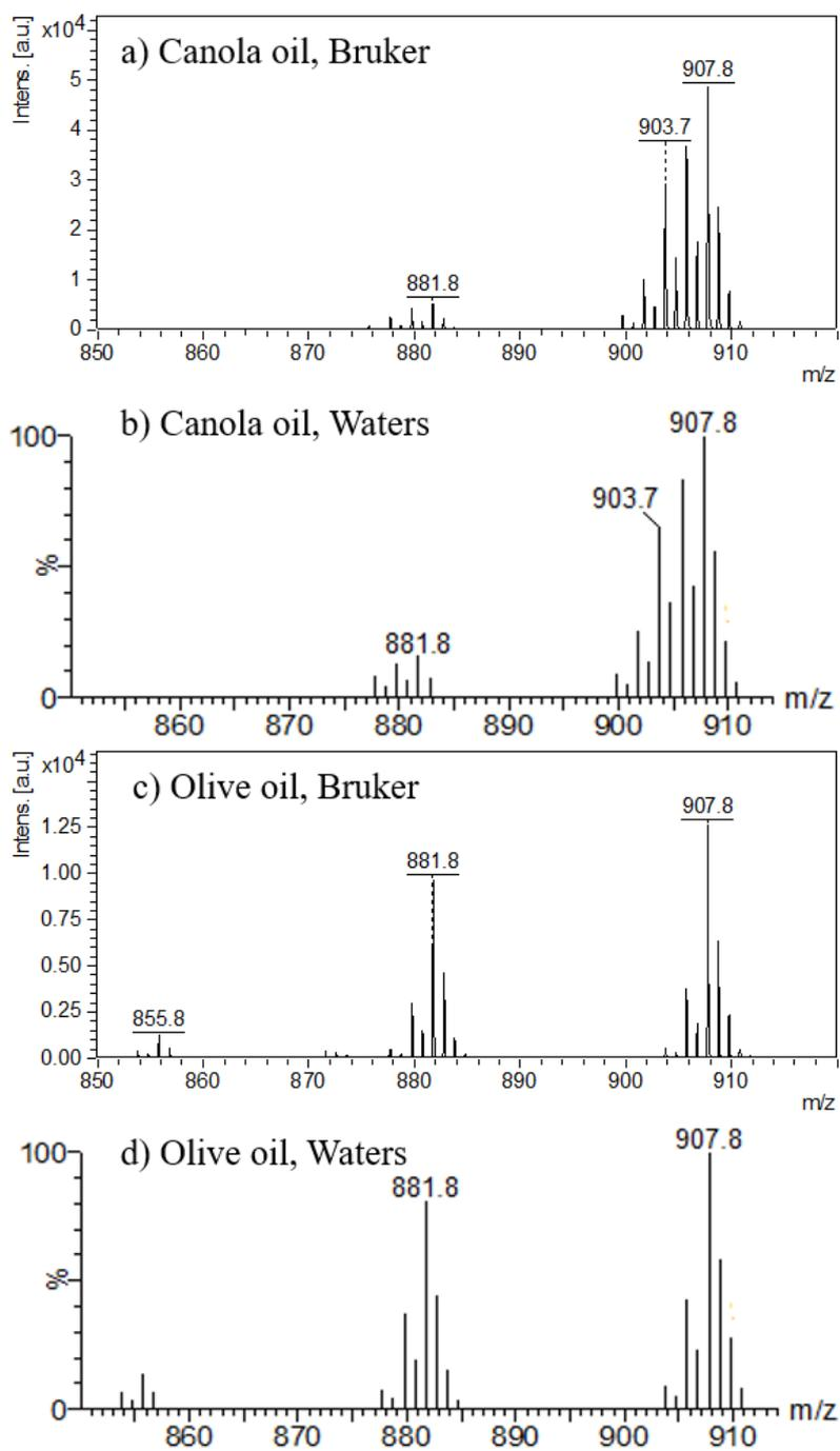
**Figure 4-6.** The mass spectra obtained of (a) a canola oil and (c) an olive oil using Bruker's MALDI-MS and the mass spectra obtained of the same (b) canola oil and (d) olive oil using Waters' MALDI-MS.
