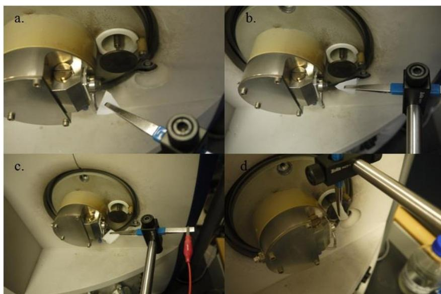
**Figure 2-3.** (a) and (b) Electrospray ionization using cotton-polyester mixture; (c) and (d) electrospray ionization using sponge.
