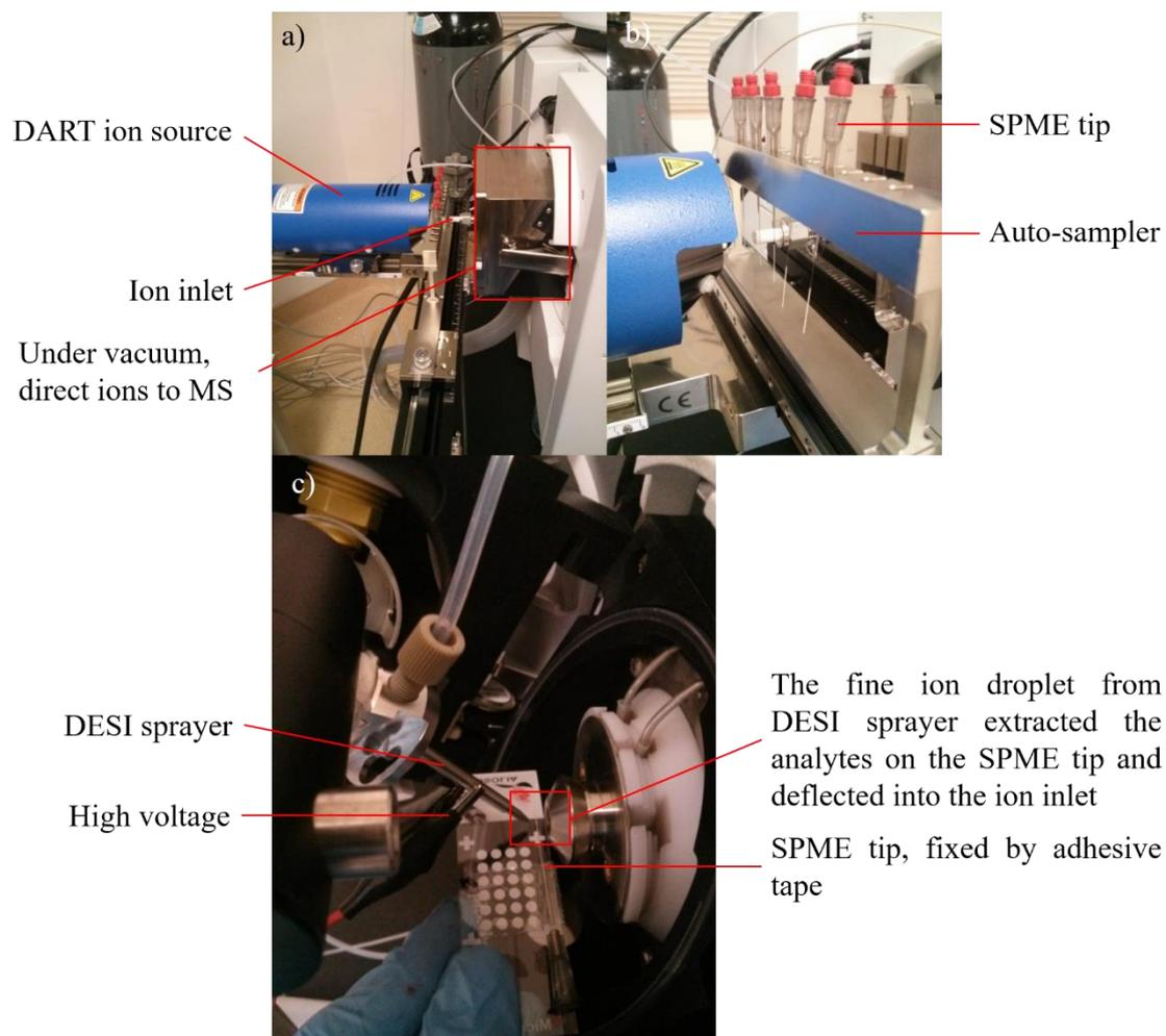
**Figure 3-2.** Experimental setup of direct coupling of SPME with mass spectrometry using (a, b) DART and (c) DESI.
