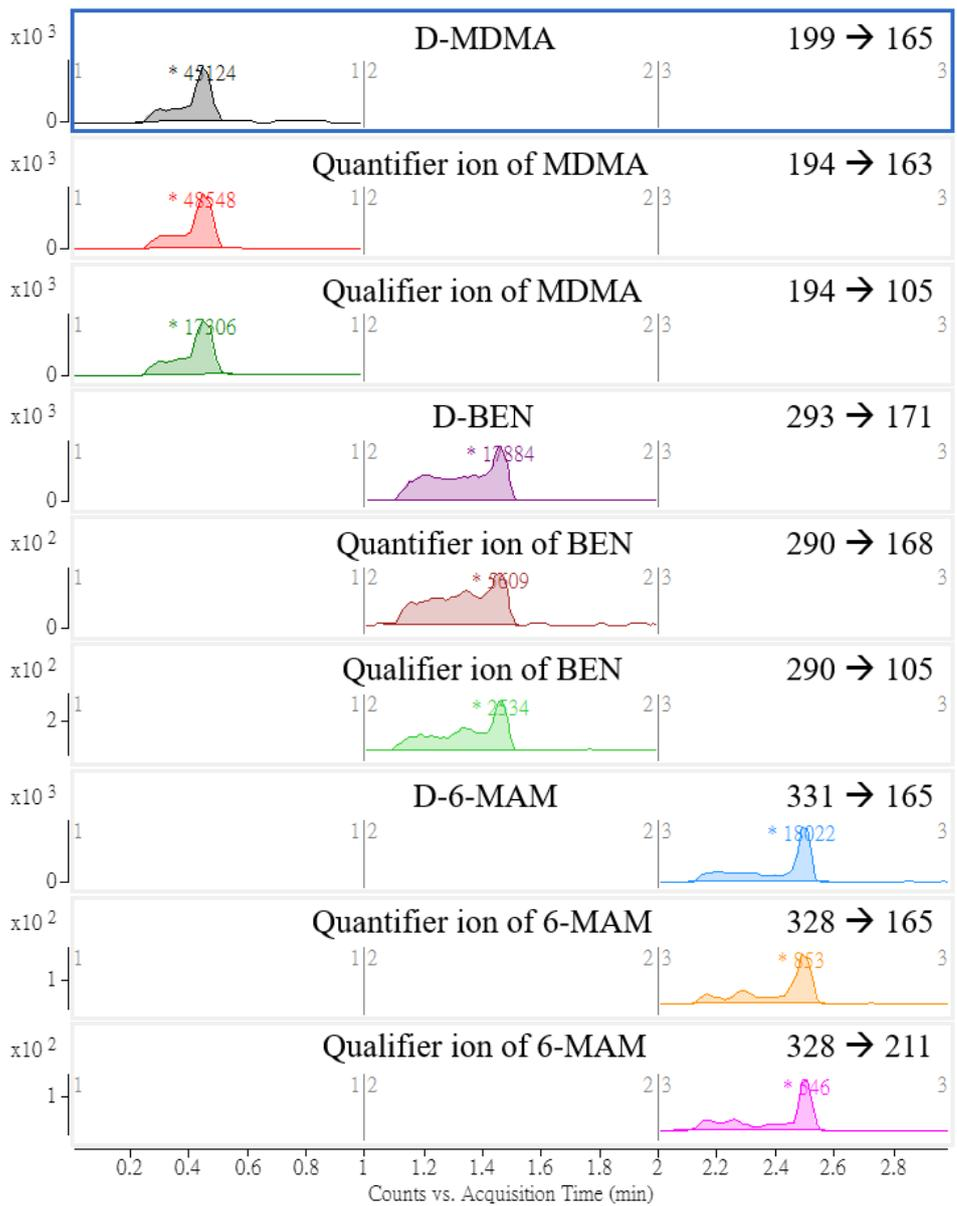
**Figure 3-16.** MRM signals for the detection of MDMA, BEN and 6-MAM in Medichem WDT confirm U +25% sample using SPME-ESI-MS.
