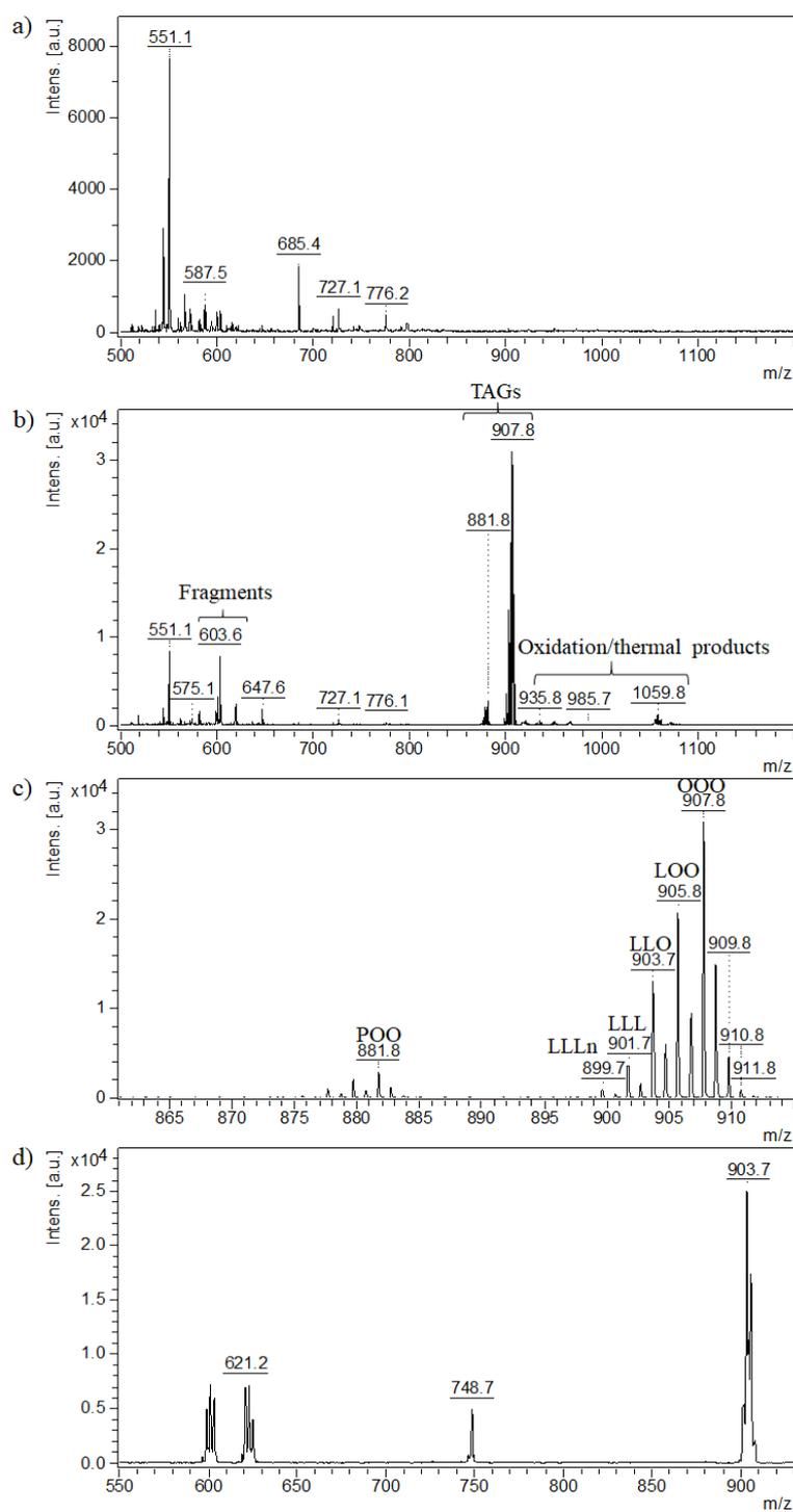
**Figure 4-7.** (a) Mass spectrum of blank DHB matrix. (b & c) Typical mass spectra of a canola oil sample and zoom in view of TAG region. TAGs were detected as Na<sup>+</sup> adducts in the spectrum. (d) MS/MS spectrum of peak *m/z* 903.7.
