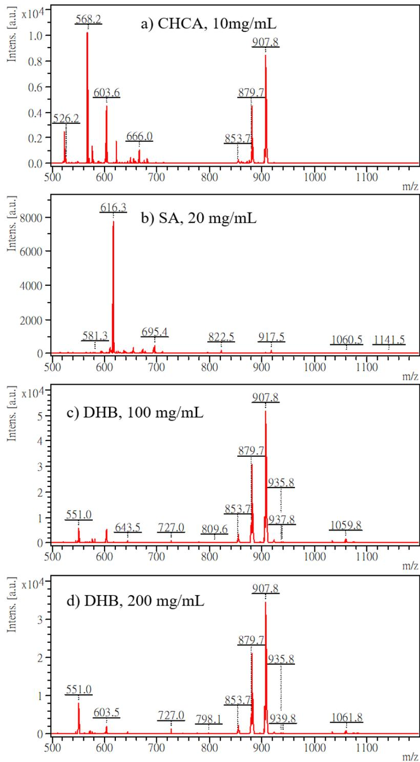
**Figure 4-3.** MALDI-MS spectra of an olive oil sample obtained using (a) 10 mg/mL CHCA, (b) 20 mg/mL SA, (c) 100 mg/mL DHB and (d) 200 mg/mL DHB as matrix.
