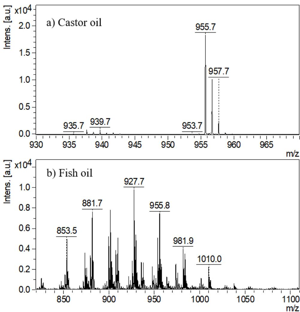
**Figure 4-12.** The mass spectra for the TAG regions of (a) castor oil and (b) fish oil.
