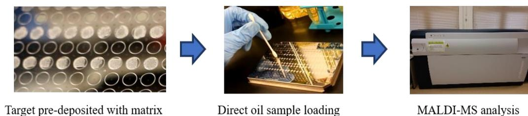
**Figure 4-1.** Direct loading of edible oil sample on the MALDI sample plate.
