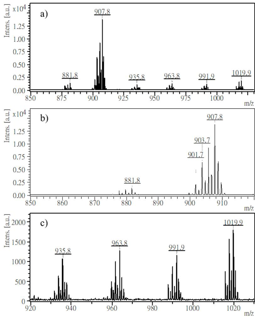
**Figure 4-18.** The mass spectra for the TAG regions of (a) rapeseed oil and the zone in view of (b) mass region  $m/z$  850 –  $m/z$  920 and (c) mass region  $m/z$  920 –  $m/z$  1030.
