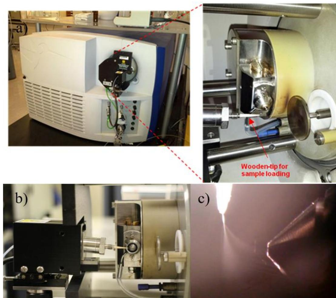
**Figure 2-1.** (a)The photos of WT-ESI-MS setup on a Micromass Quattro Ultima triple quadrupole mass spectrometer. (b) A close-up of a wooden tip mounted into nano-ESI source for WT-ESI-MS analysis. (c) Electrospray of sample solution applied onto wooden tip.
