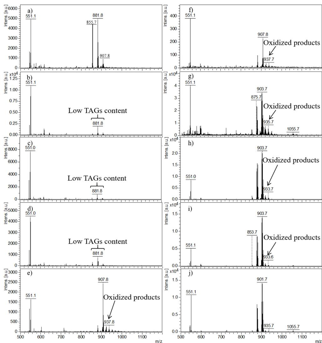
**Figure 4-25.** The mass spectra of gutter oil samples (a) s469, (b) s470, (c) s471, (d) s472, (e) s473 and (f) s474, and the mass spectra of (g) soybean oil heated for 20 hr, (h) soybean oil cooked with food for 20 hr, (i) soybean oil cooked with food for 16 hr, and (j) soybean oil cooked with food for 8 hr.
