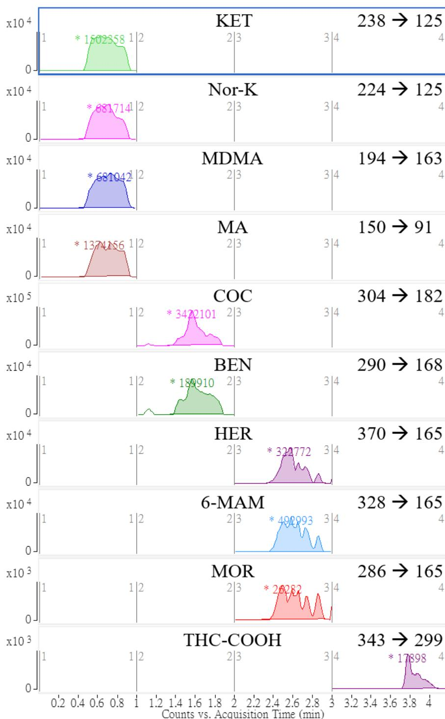
**Figure 3-19.** The MRM results for the detection of a mixture of 900 ng/mL targeted analytes using SPME-ESI-MS. Only the quantifier ion channels were shown.
