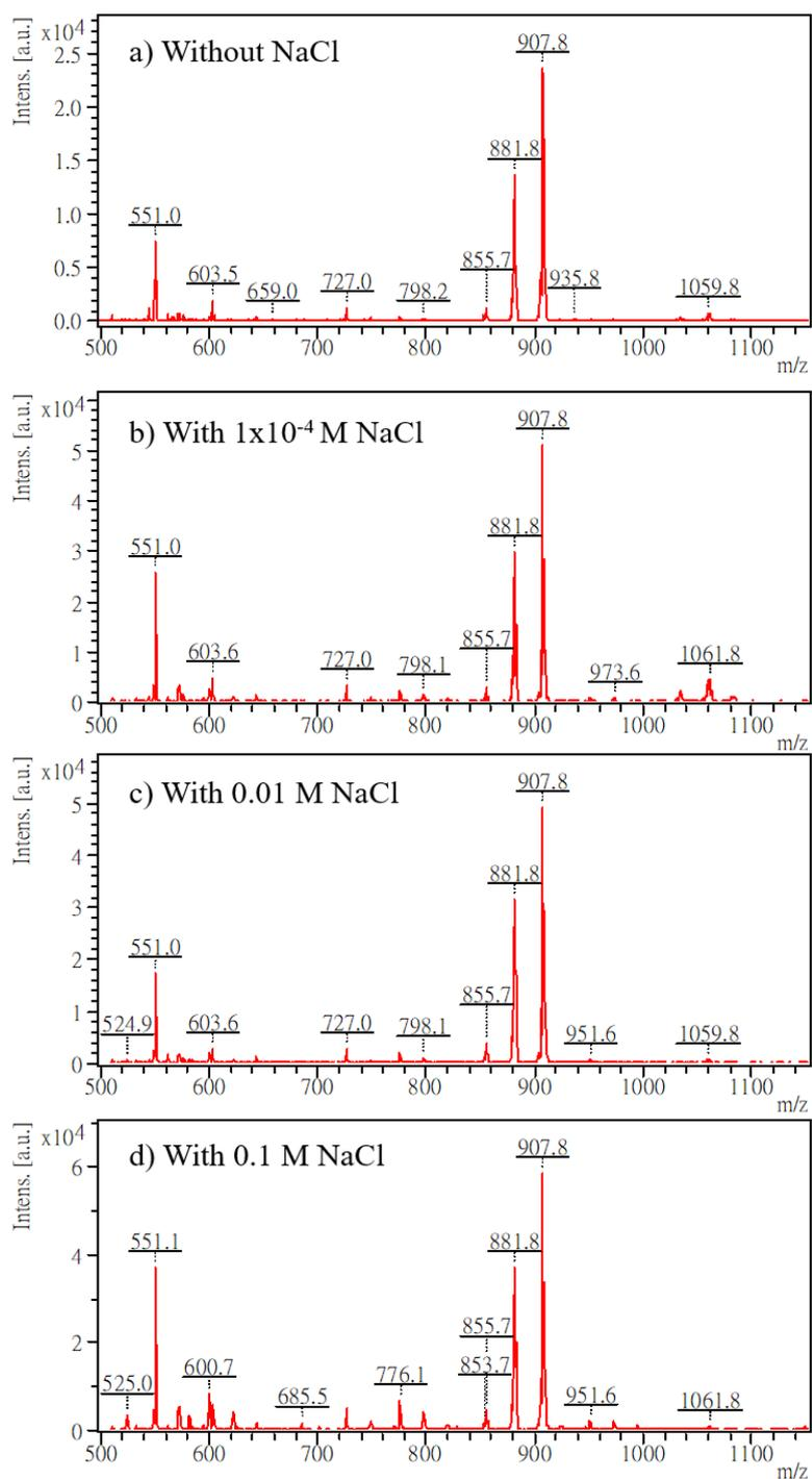
**Figure 4-4.** MALDI-MS spectra of an olive oil sample obtained with the addition of (a) 0 M, (b)  $1 \times 10^{-4}$  M, (c) 0.01 M and (d) 0.1 M sodium chloride solution into the matrix solution (final concentration).
