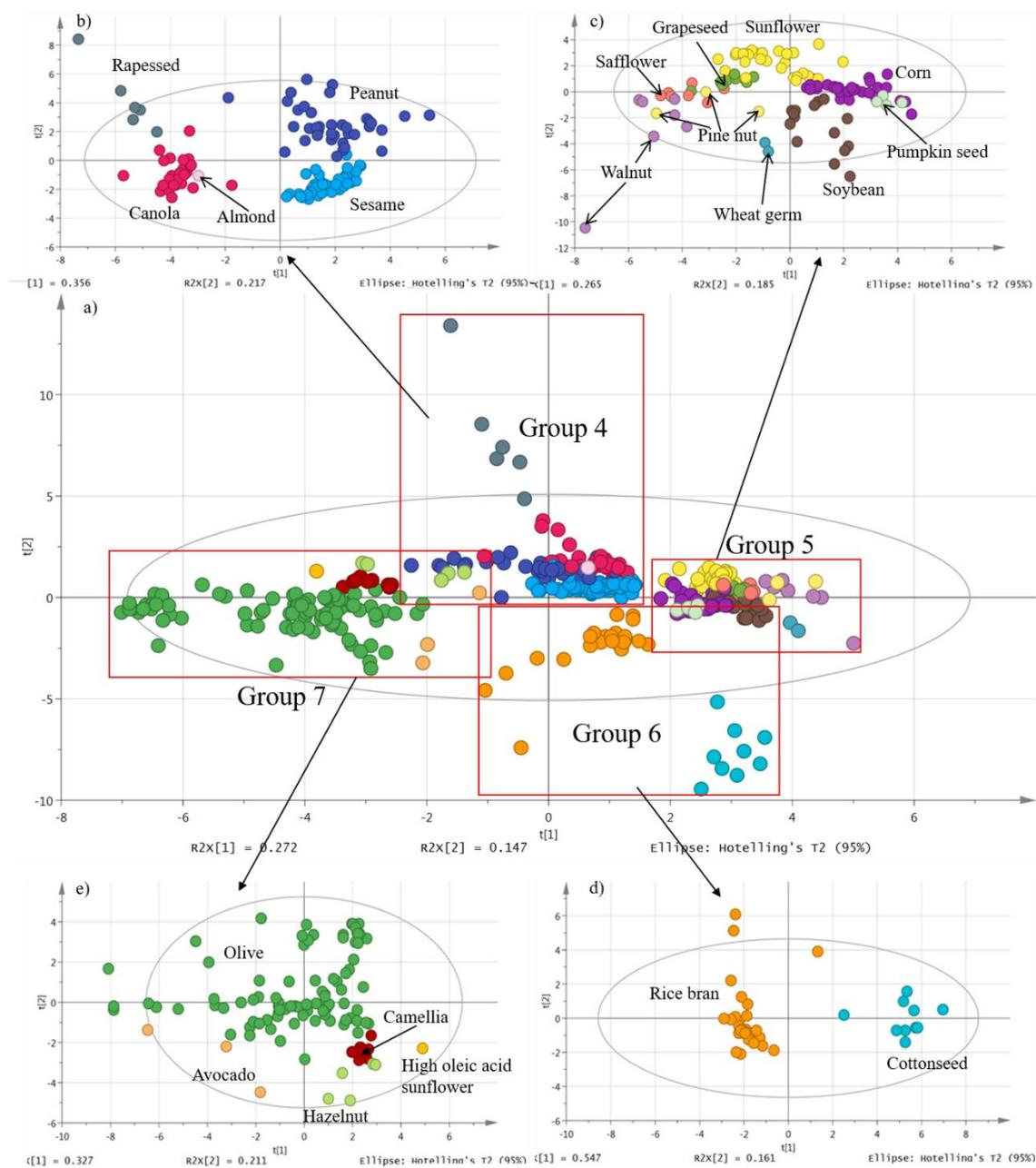
**Figure 4-21.** (a) PCA score plot for different edible oils based on their MALDI-MS results after removing groups 1, 2 and 3 as well as castor oil and fish oil. The first principal accounted for 27% of variance and second principal accounted for 15% of variance. (b-e) PCA score plots for (b) group 4, (c) group 5, (d) group 6 and (e) group 7. The first principal accounted for 36%, 27%, 55% and 33% of variance and second principal accounted for 22%, 19%, 16% and 21% of variance, respectively.
