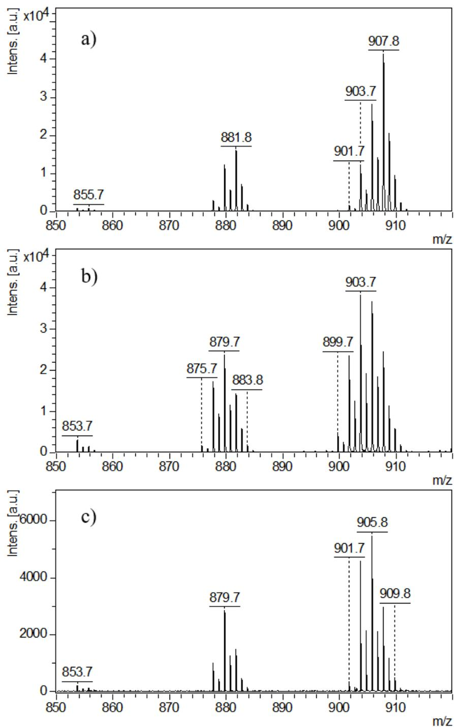
**Figure 4-9.** (a-c) The TAG region with different spectral patterns of three peanut oil samples collected from different brands.
