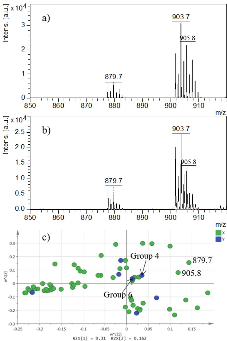
**Figure 4-22.** Mass spectra for the TAGs regions of (a) a misclassified sunflower oil sample and (b) a typical sunflower oil sample. (c) PLS-DA loading plot for the classification of samples into different groups.
