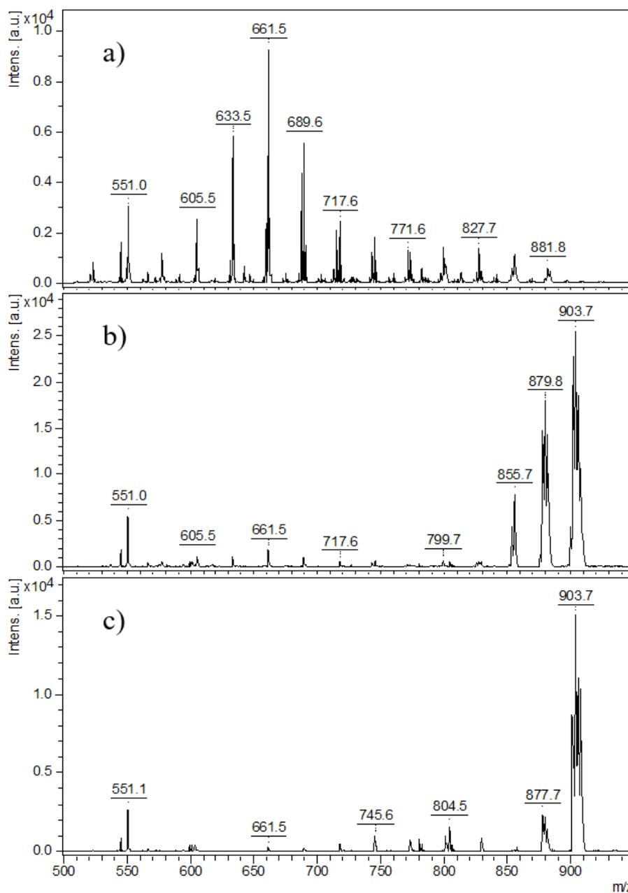
**Figure 4-14.** The MALDI-MS spectra of (a) a butter sample, (b) a margarine sample (mixture of soybean, palm, coconut and rapeseed oils) and (c) another margarine sample (mixture of sunflower oil and other unspecified vegetable oils).
