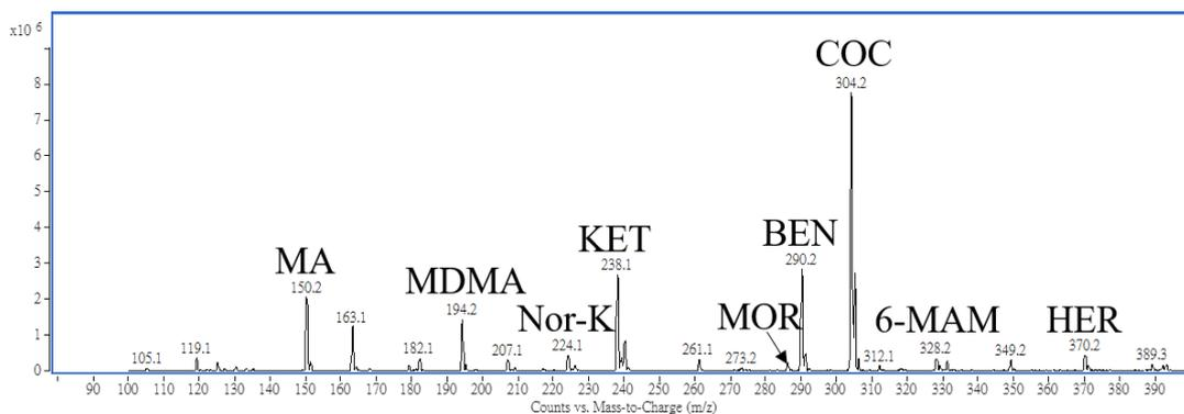
**Figure 3-17.** The mass spectrum for analyzing a mixture of 2000 ng/mL targeted analytes in MeOH using conventional ESI-MS.
