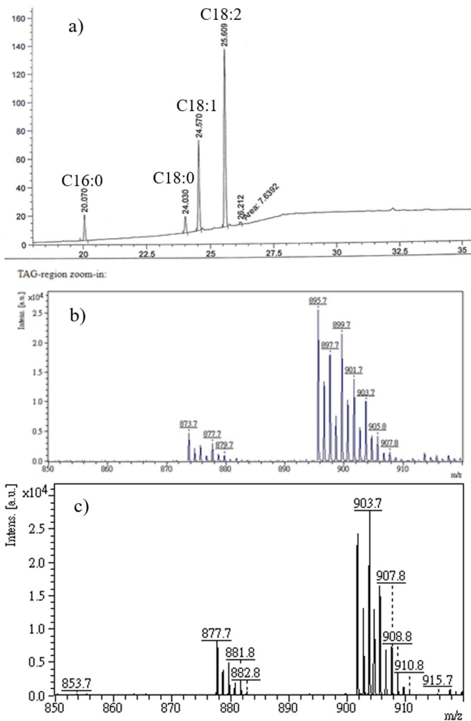
**Figure 4-23.** (a) The GC-FID result of the faked flaxseed oil sample. (b) A reference MALDI-MS spectrum of flaxseed oil recorded in the home-built database and (c) the MALDI-MS spectrum of the faked flaxseed oil sample.
