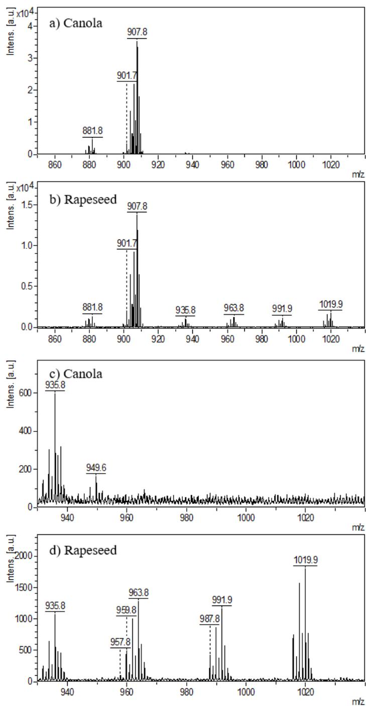
**Figure 4-11.** The full MALDI-MS spectra of (a) a canola oil and (b) a rapeseed oil and the zoom-in view ( $m/z > 930$ ) of (c) the canola oil and (d) the rapeseed oil.
