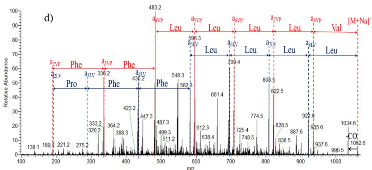
**Figure 4-16.** (a) The full MALDI-MS spectrum and (b) the cyclolinopeptides region MALDI-MS spectrum of a flaxseed oil sample. (c) The mass spectrum of a flaxseed oil sample analyzed using ESI-orbitrap MS. (d) The orbitrap MS/MS spectrum of ion  $m/z$  1062.6 showed two a-ion series of cyclolinopeptide A.
