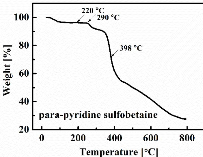
Fig 4.7. TGA analysis of para-pyridine sulfobetaine
