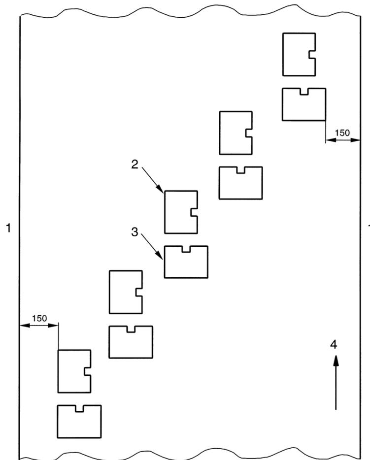
Fig 3.2. Example of pattern for cutting out test specimens from the laboratory sample.
