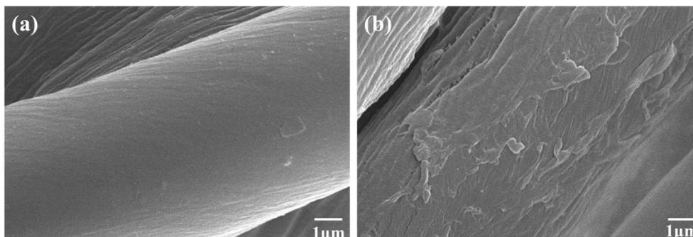
Fig 4.8. SEM images of cotton fiber in cotton fabrics before (a) and after finishing process (b) with para-pyridine sulfobetaine.
