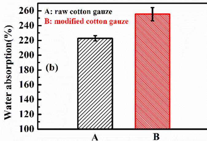
Fig 4.13. Air permeability (a) and water absorption (b) of cotton fabrics.
