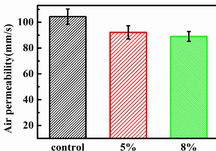
Fig 6.1. Air permeability results of cotton fabrics before (control) and after finishing (5% and 8%)
