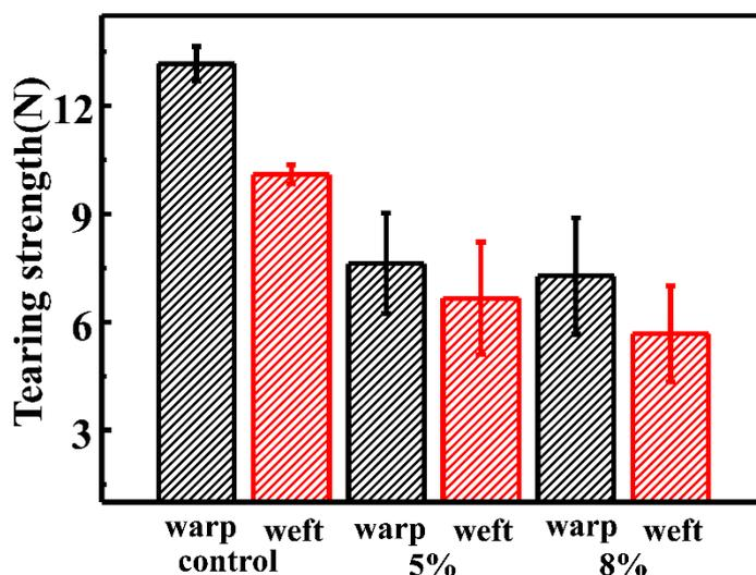
Fig 6.2. Tearing strength results of cotton fabrics before (control) and after finishing (5% and 8%) in warp and weft directions
