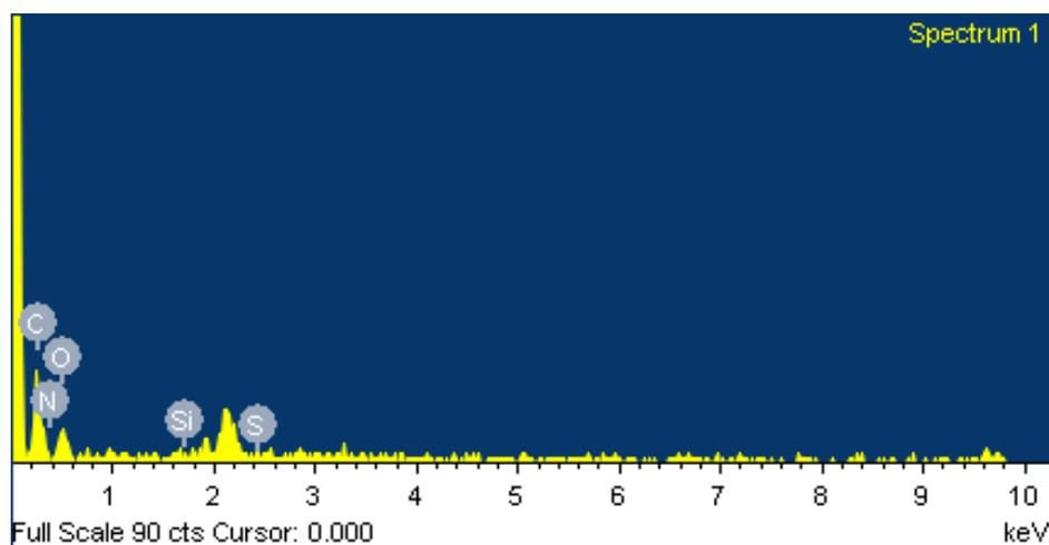
Fig 4.9. EDX result of the modified cotton fabric with para-pyridine sulfobetaine.
