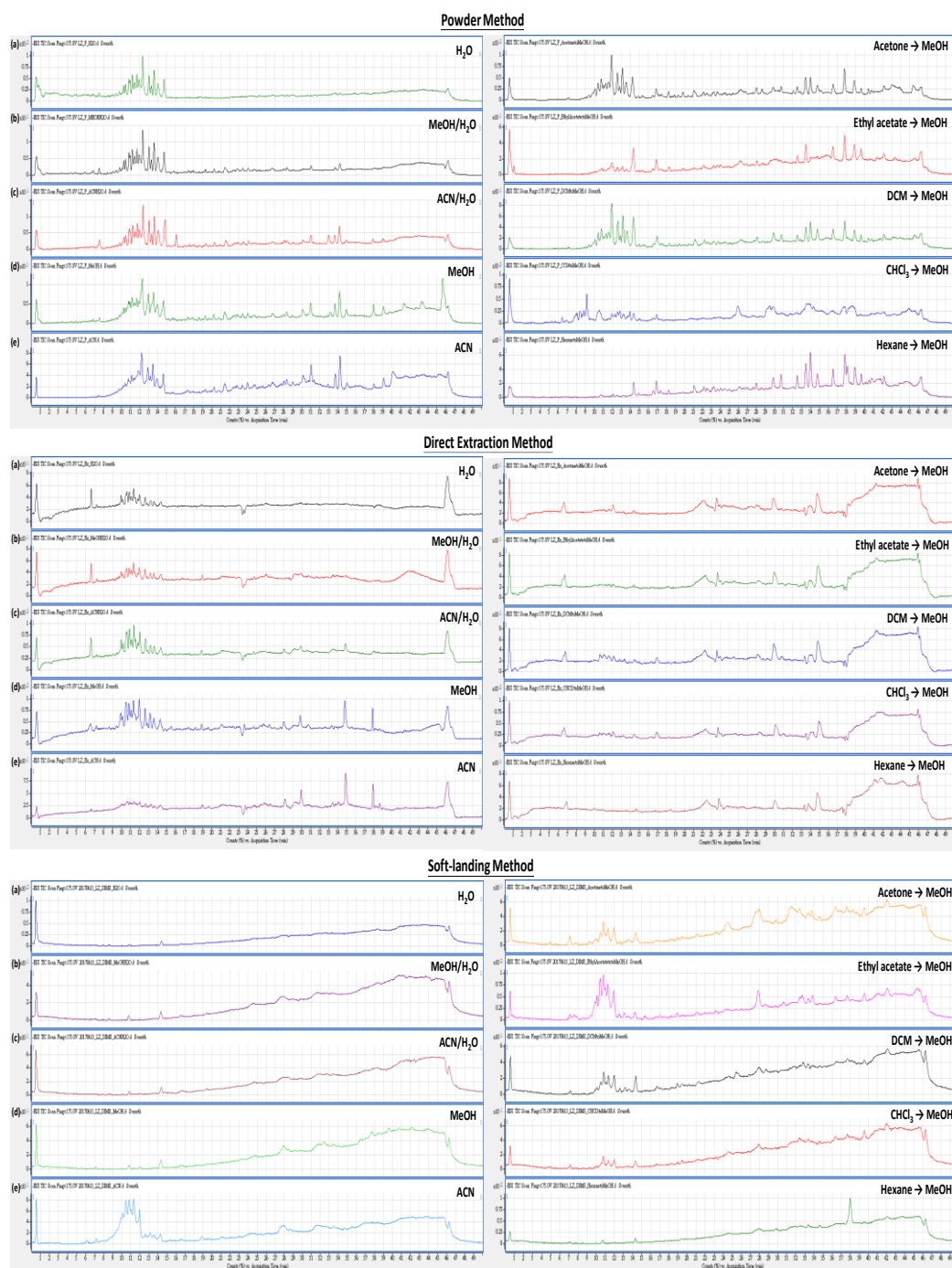
Figure 4.4. Total ion chromatogram (TIC) obtained by UPLC-MS analysis of the Ganoderma lucidum samples collected by the powder extraction method, direct extraction method and soft-landing method with the application of different solvents: (a) water, (b) methanol/water (1/1), (c) acetonitrile/water (1/1), (d) methanol, (e) acetonitrile, (f) acetone, (g) ethyl acetate, (h) dichloromethane, (i) chloroform, and (j) hexane, where (e) to (j) were reconstituted into methanol.
