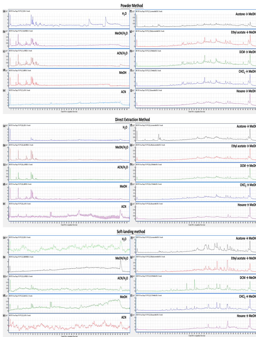
Figure 4.23. Total ion chromatogram (TIC) obtained by UPLC-MS analysis of the Ilex latifolia leaves samples collected by the powder extraction method, direct extraction method and soft-landing method with the application of different solvents: (a) water, (b) methanol/water (1/1), (c) acetonitrile/water (1/1), (d) methanol, (e) acetonitrile, (f) acetone, (g) ethyl acetate, (h) dichloromethane, (i) chloroform, and (j) hexane, where (e) to (j) were reconstituted into methanol.
