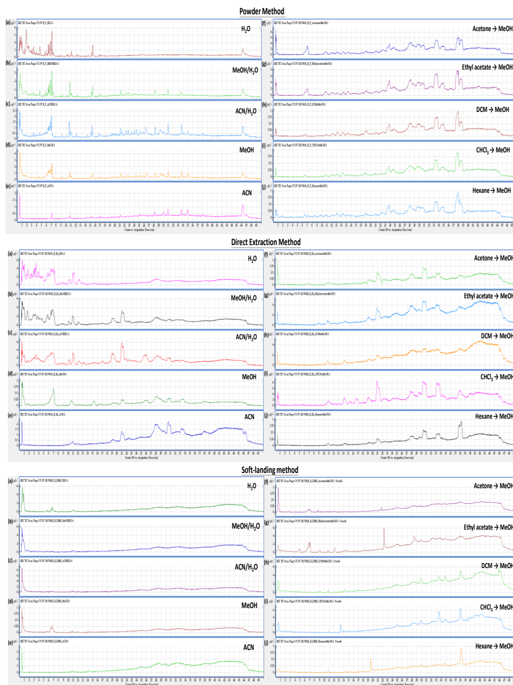
Figure 4.10. Total ion chromatogram (TIC) obtained by UPLC-MS analysis of the Hylocereus undatus samples collected by the powder extraction method, direct extraction method and soft-landing method with the application of different solvents: (a) water, (b) methanol/water (1/1), (c) acetonitrile/water (1/1), (d) methanol, (e) acetonitrile, (f) acetone, (g) ethyl acetate, (h) dichloromethane, (i) chloroform, and (j) hexane, where (e) to (j) were reconstituted into methanol.
