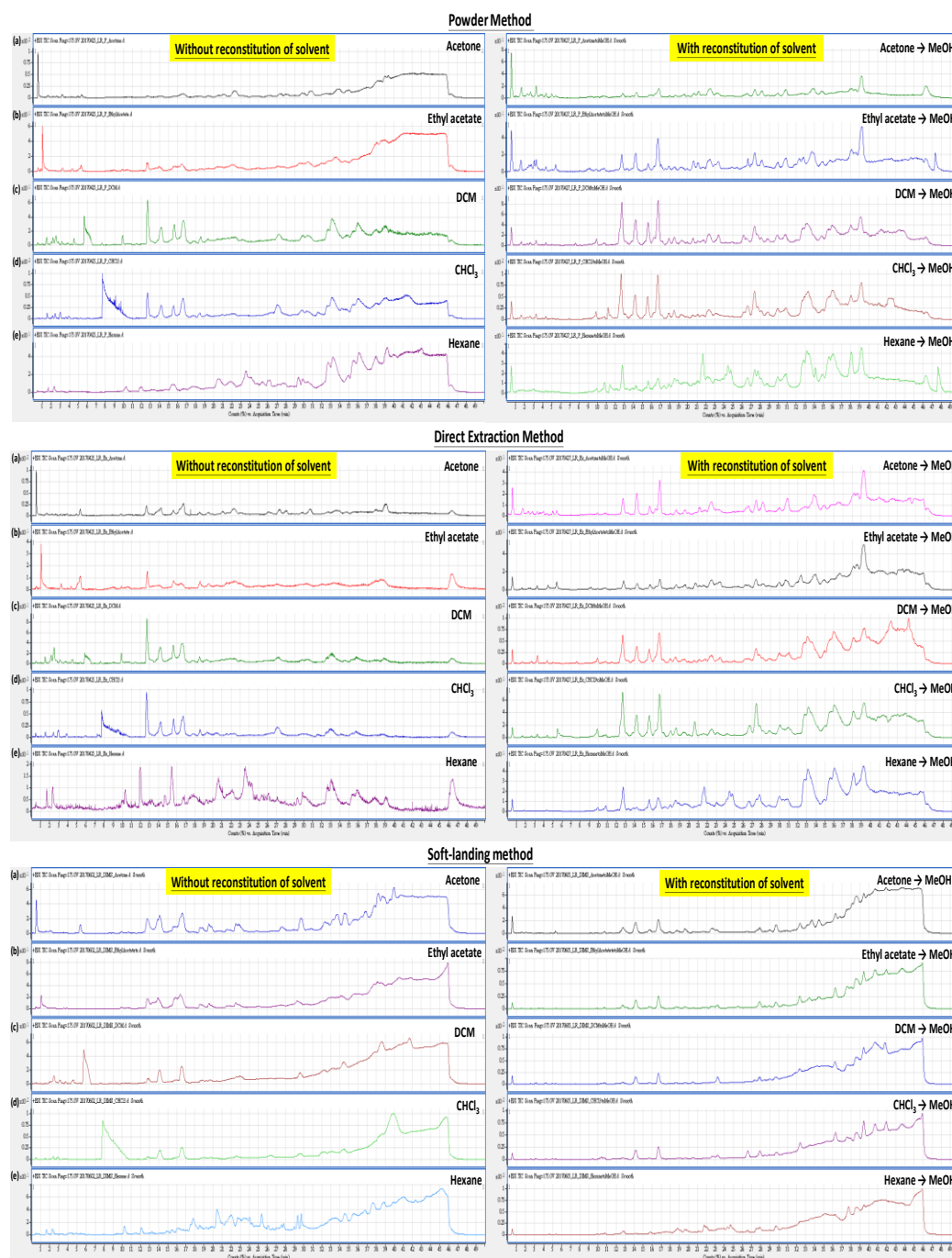
Figure 4.16. Total ion chromatogram (TIC) obtained by UPLC-MS analysis of the Lycoris radiata samples collected by the powder extraction method, direct extraction method and soft-landing method with the application of different solvents: (a) acetone, (b) ethyl acetate, (c) dichloromethane, (d) chloroform, and (e) hexane without (left), or with (right), reconstitution of solvent into methanol.
