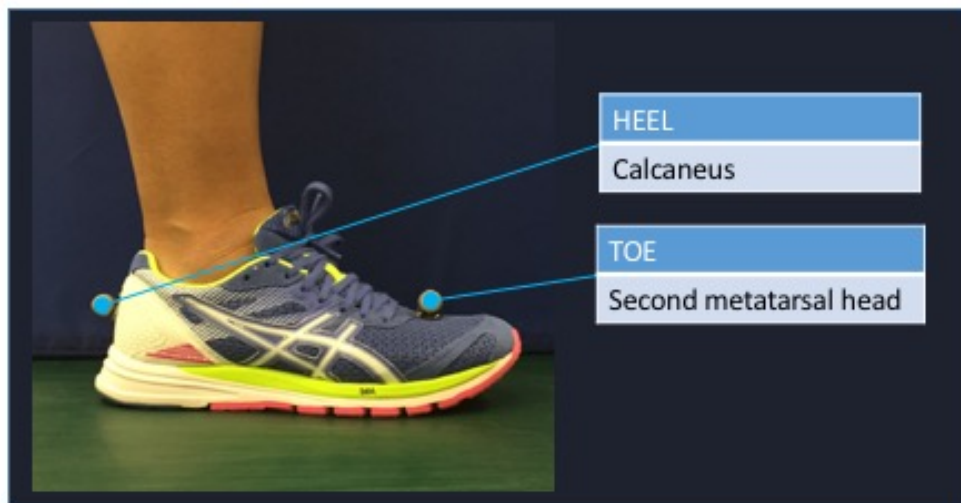
Figure 2.1 Reflective marker positions for HEEL and TOE
