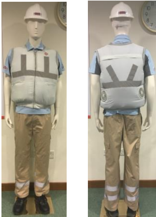
Figure 4.1 The newly designed PCS (two-layer cooling vest) worn over the construction uniform (from left to right: front view, back view)
