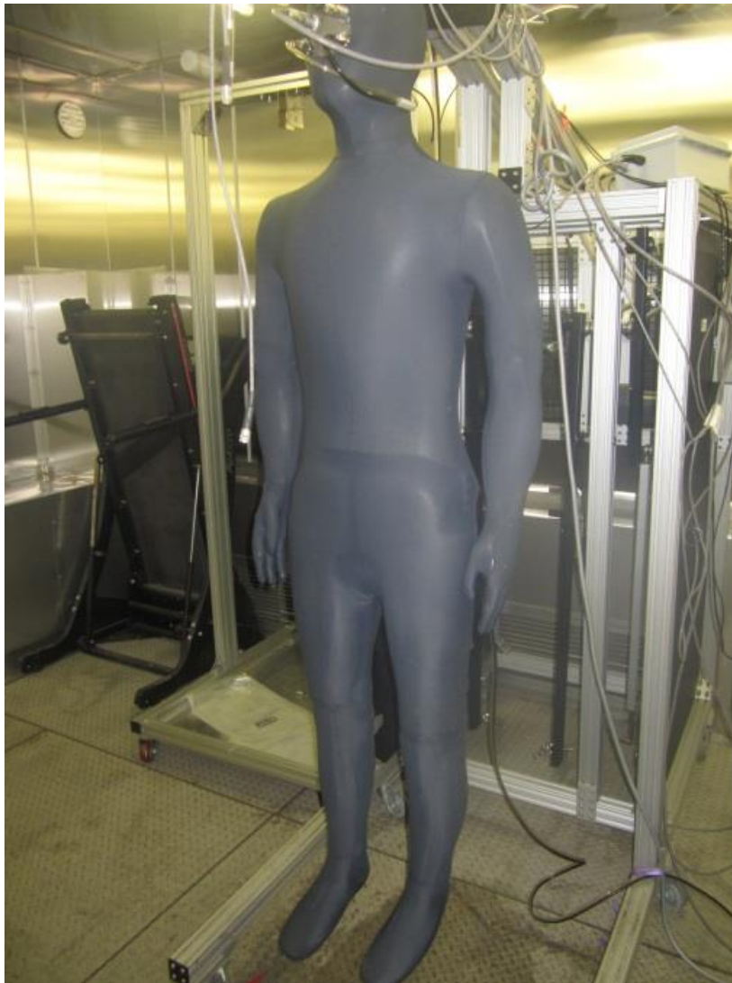
Figure 3.2 The sweating thermal manikin in a climatic chamber
