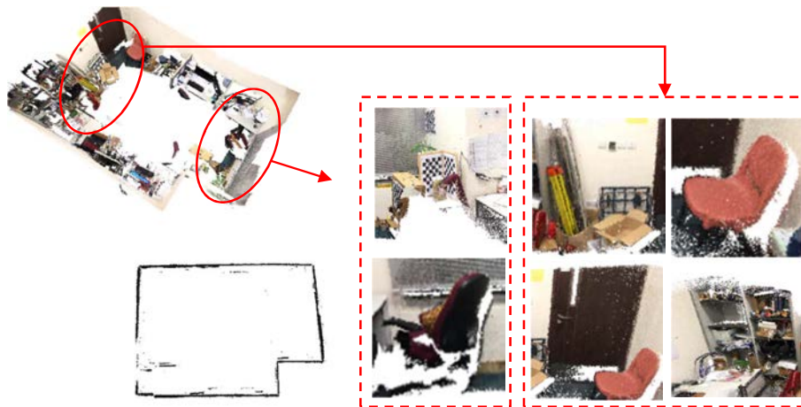
Figure 4.13: 3D model reconstruction of an office using the calibrated data of sensor 1
