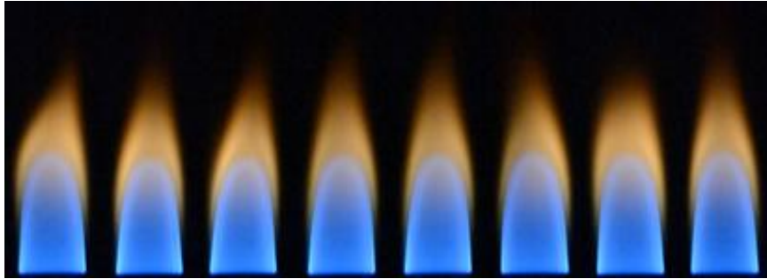
Fig.2.3: Instantaneous images of an IDF with Re_i = 192 and Re_o = 46 .
