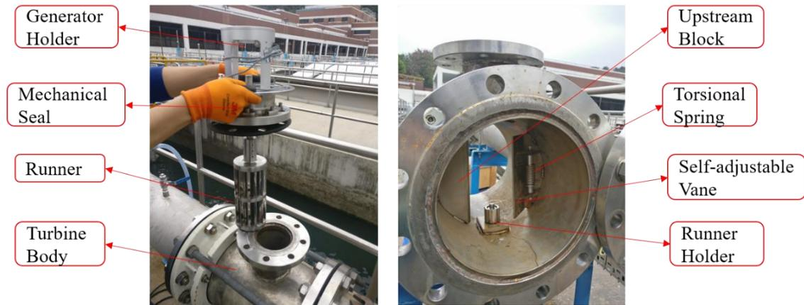
Fig.3.24 The inline cross-flow turbine prototype
