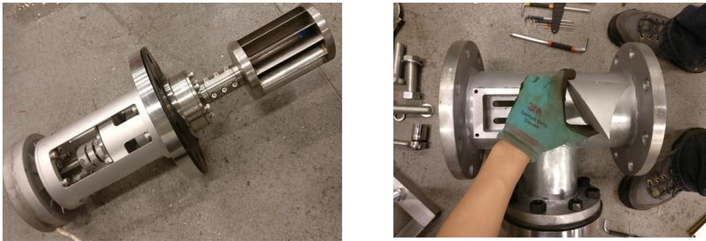
Fig.8.6 Prototype of the bidirectional turbine
