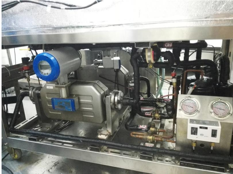
Photo 7 Refrigerant mass flow meters
