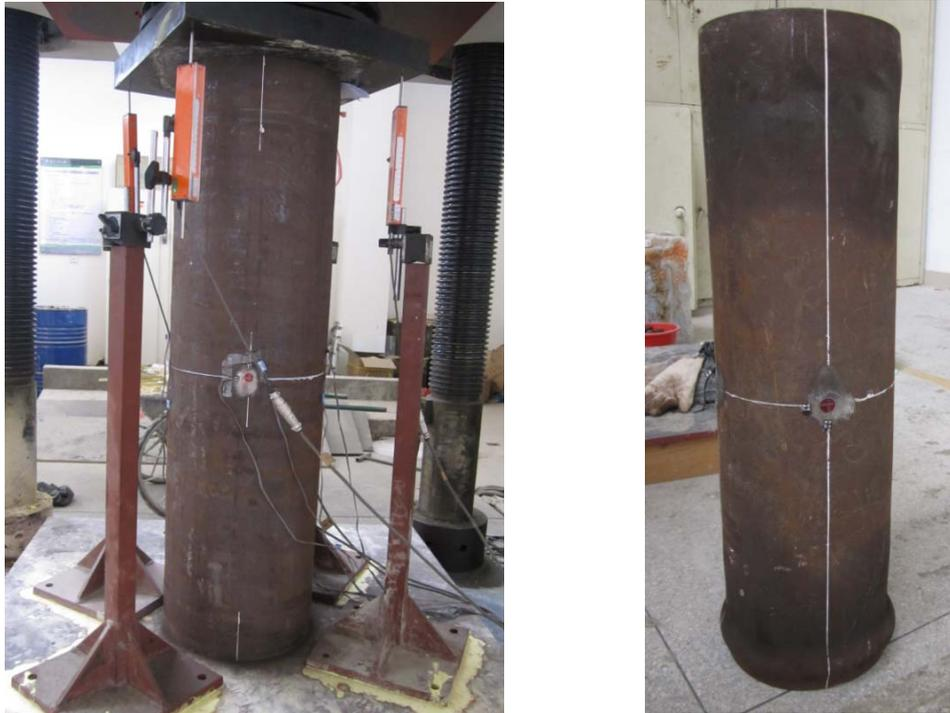
**Figure 6. 2** Test setup and buckling of bare steel tubes under axial compression
