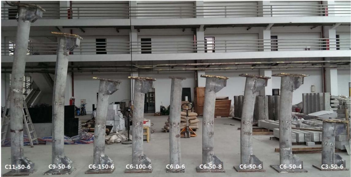
**Figure 8.7** General view of steel tubes after test
