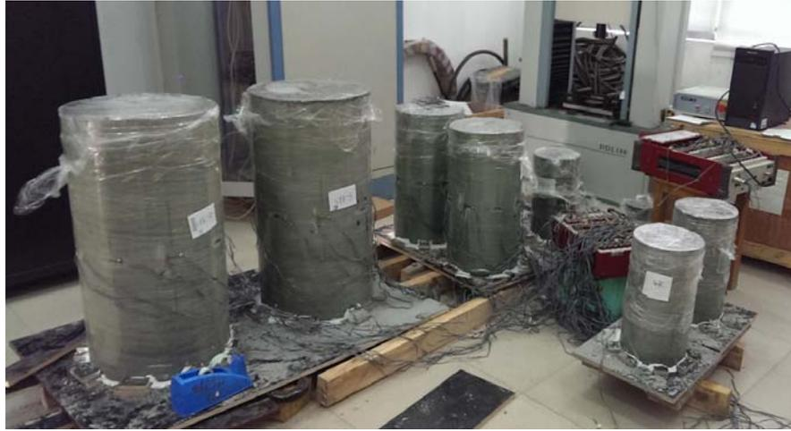
**Figure 4. 4** Strain measurement of specimens filled with SCEC
