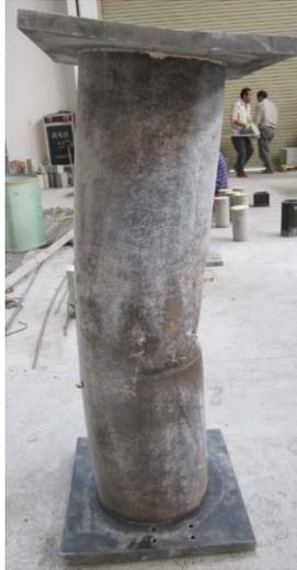
**Figure 7. 7** Buckling of inner steel tube
