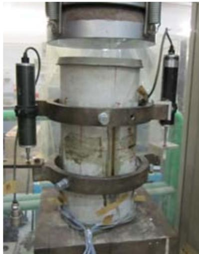
**Figure 4. 2** Control cylinder test
