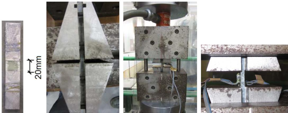
**Figure 3. 4** Strip specimen for compression test and compression test setup
