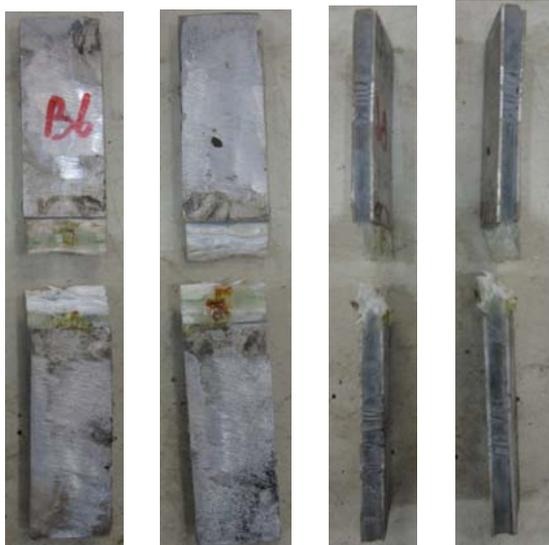
**Figure 3. 6** Failure mode of compression test on FRP strip specimens
