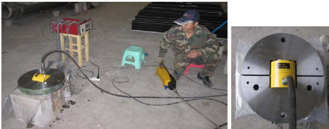
**Figure 3. 7** Setup of split disk tests
