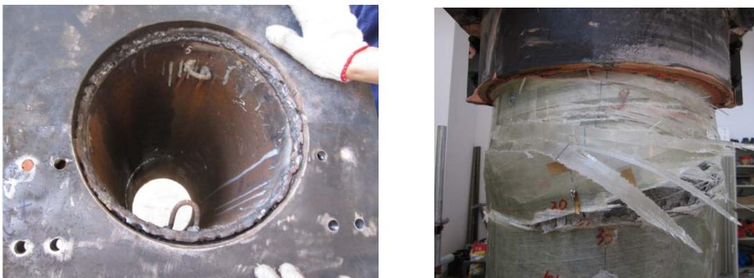
**Figure 7. 3** Local failure of specimen CE325-10-P4N-100 (damaged)
