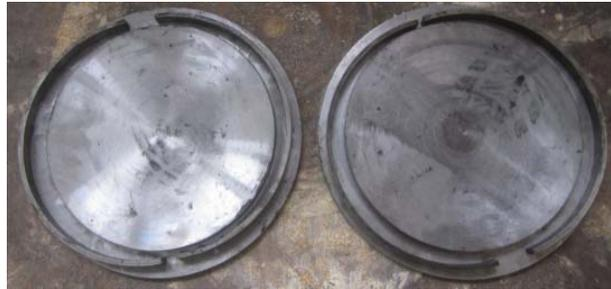
**Figure 3. 13** Loading platens with a groove to fit the ends of tube specimen
