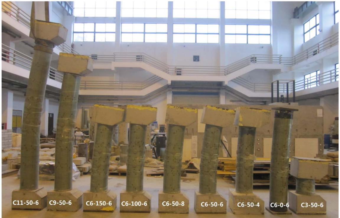
**Figure 8. 5** General view of all slender hybrid DSTCs after tests
