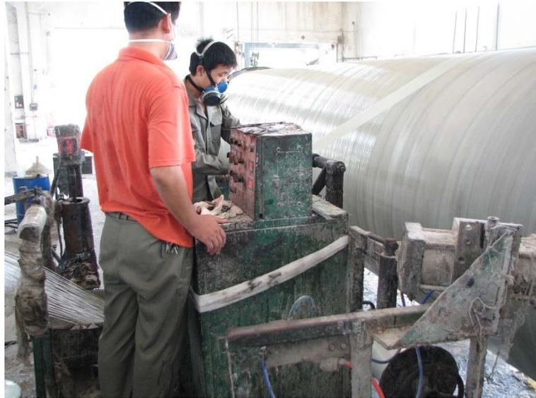
**Figure 2. 1** Filament winding process
