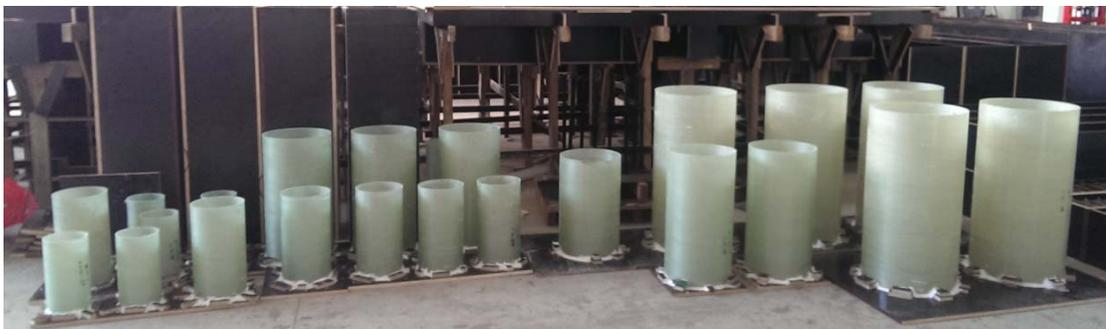
**Figure 4. 3** Preparation of filament-wound GFRP tubes
