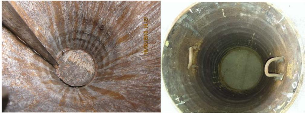
**Figure 6.7** Global buckling of the inner steel tube of hybrid DSTCs
