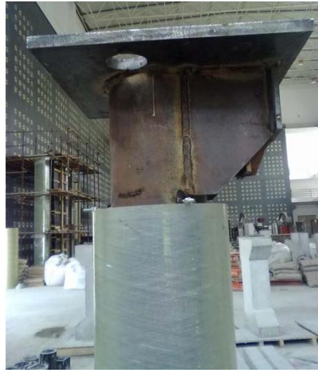
**Figure 8. 2** Construction of the corbel ends of eccentrically-loaded slender DSTCs
