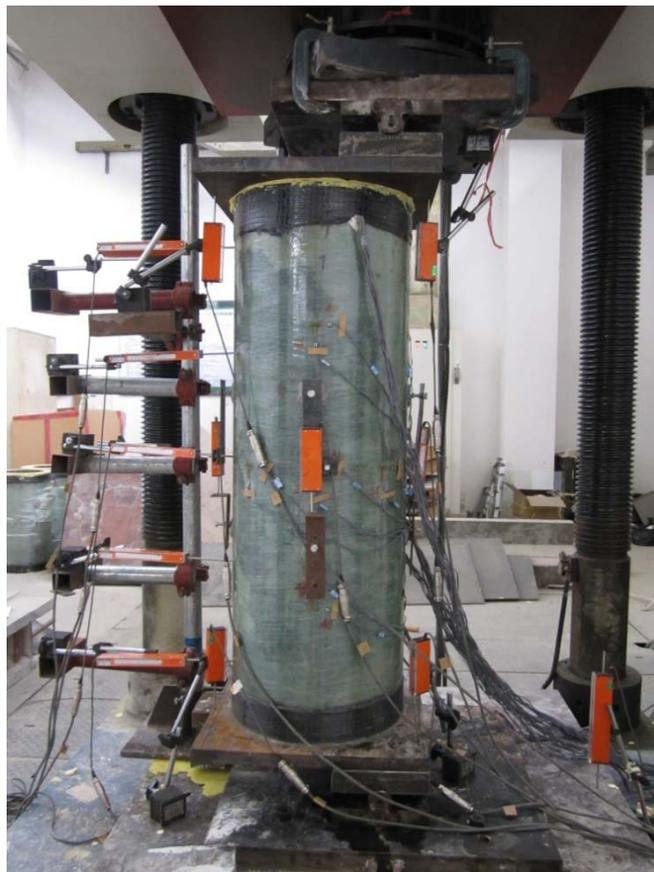
**Figure 7. 5** Setup of eccentric compression tests on DSTCs
