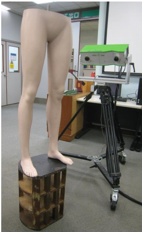
Figure 4-16. The mannequin was scanned by Comet Vario Zoom scanner by Steinbichlar GmbH
