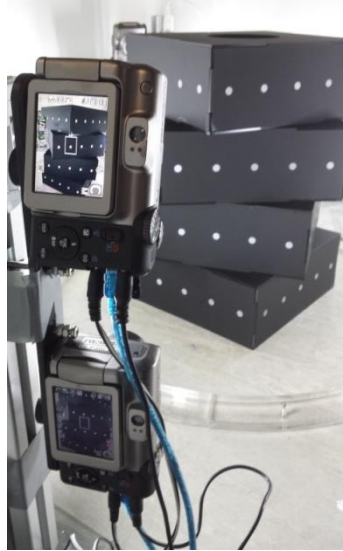
Figure 4-6. Each camera has to take an image on the calibration range during camera calibration
