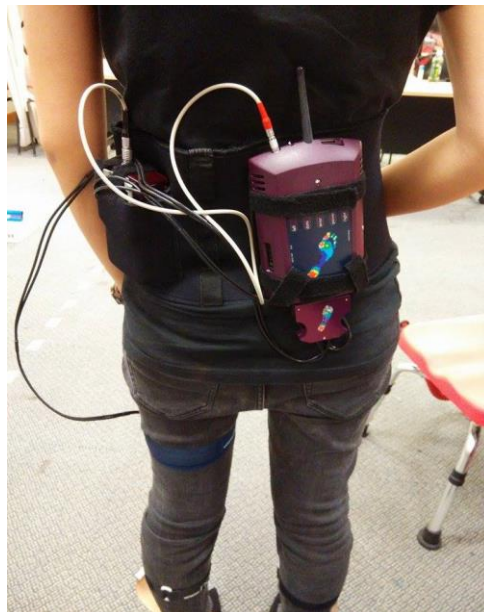
Figure 5-3. Setup of Pedar®-X in-shoe pressure measurement system
