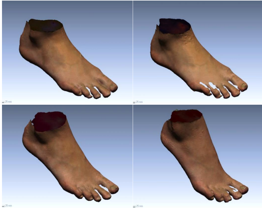
Figure 4-1. Foot scanned images from the Frontier 3D foot laser scanner with foot of subject resting flat on the scanning platform (top left); foot heel resting on support that is 1 cm (top right), 5 cm (bottom left) and 8 cm (bottom right) in height.
