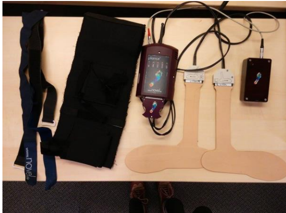
Figure 5-2. Pedar®-X in-shoe pressure measurement system
