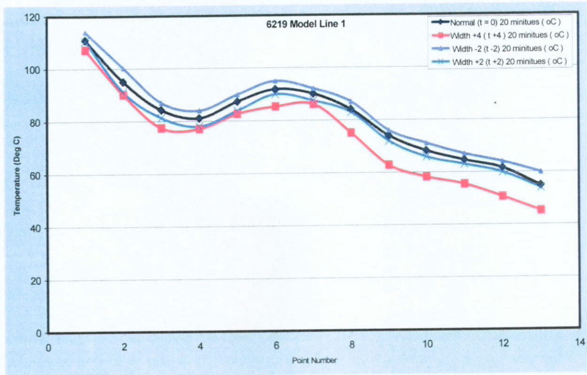
Fig. 98 Experimental Temperature Results of Model 1 (Line 1)
