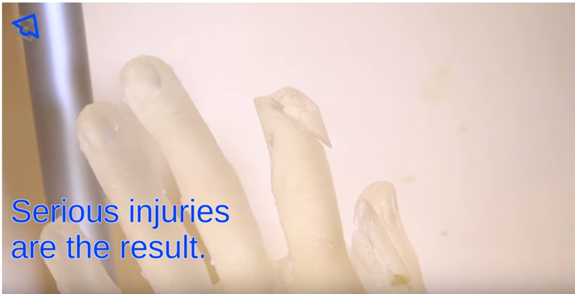
Figure 1.2: Quadcopter propellers cause serious finger injuries [2].
