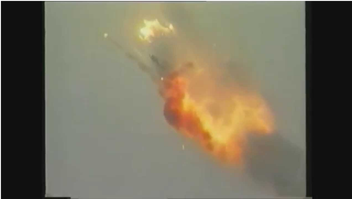
Figure 1.1: Ariane-5 explosion (quoted from [1]), which resulted in US$500 million loss, is due to a bug in the cyber subsystem [84].
