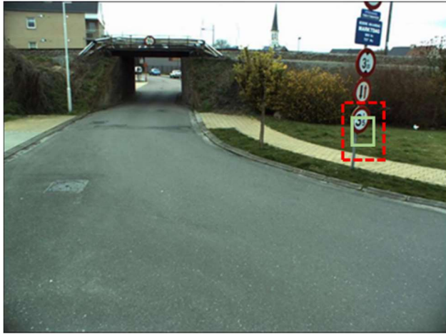
Figure 15. The effect of a badly located road sign: Green: the bounding box predicted by a poor detector. Red: the enlarged region to be fed into a classifier.
