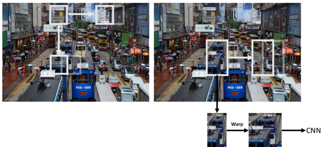
Figure 1. The sliding window approach: Search windows with different scales and aspect ratios are used to explore the entire image.
