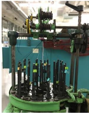
Figure 3.5 The conventional vertical circular braiding machine utilized for manufacturing developed auxetic braided structures.
