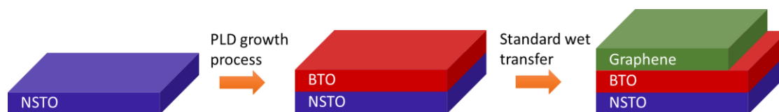
Figure 3. 1 Schematic fabrication process of graphene/BTO/NSTO heterostructure.
