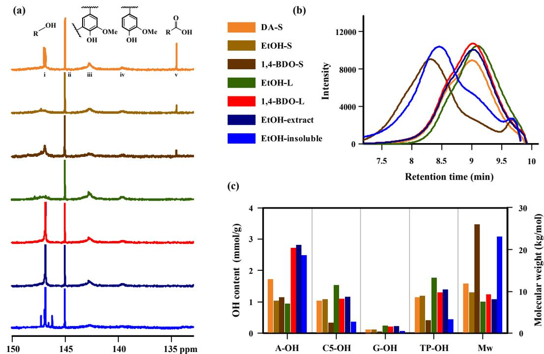
Fig. 6.5 Chemical characteristics pretreated lignin samples after DA (15 mM acid); EtOH; and 1,4-BDO (15 mM acid and 65% organosolv). (a)  $^{31}\text{P}$  NMR spectra; (b) GPC chromatogram; and (c) overall comparisons. S: residue lignin; L: organosolv soluble lignin; EtOH-extract and EtOH-insoluble lignin was harvested from 1,4-BDO-L lignin as detailed in Fig. 6.2 and the text.
