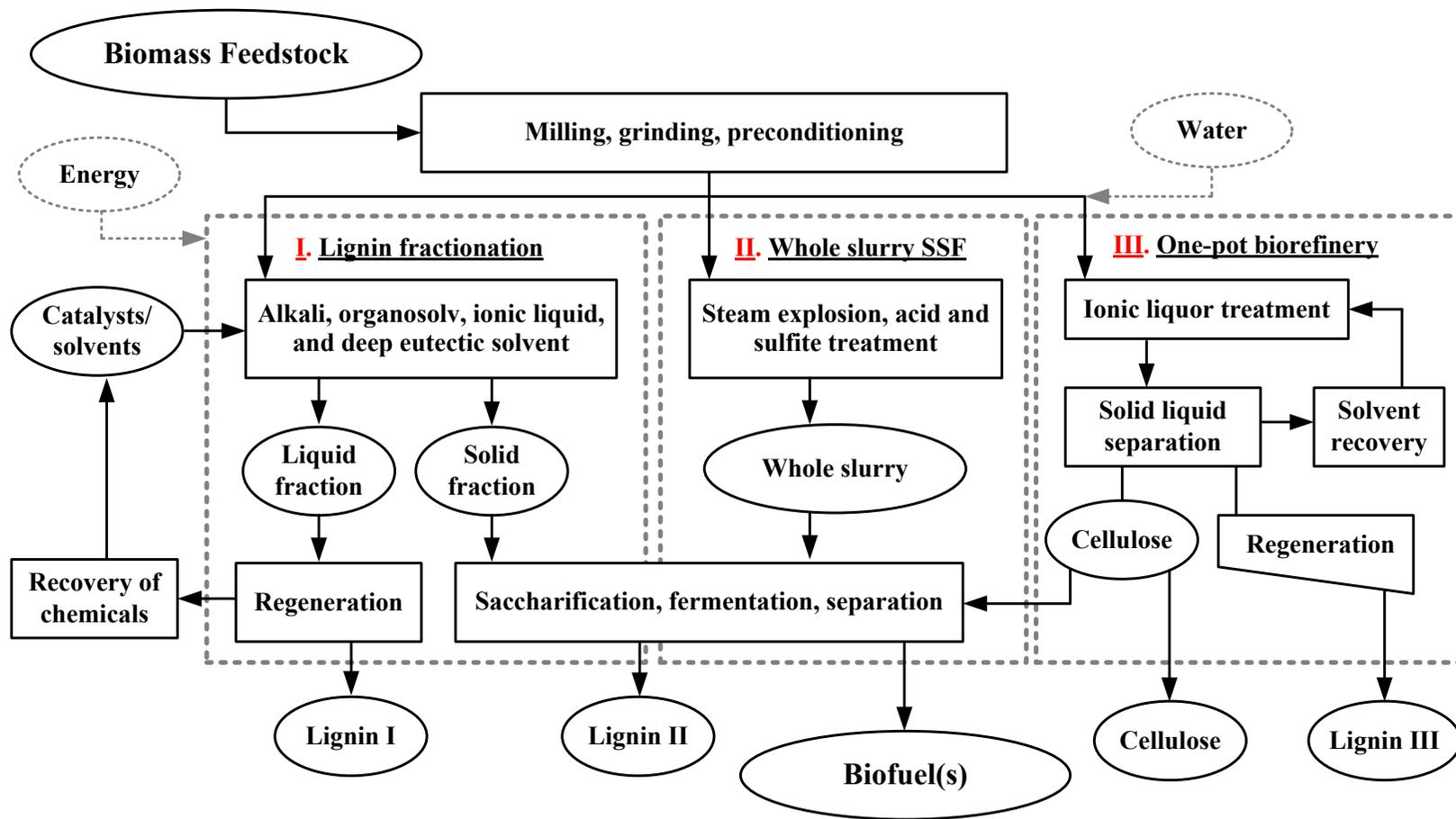
Fig. 2.5 Three biorefinery concepts for complete utilization of lignocellulosic biomass in bioenergy system.
