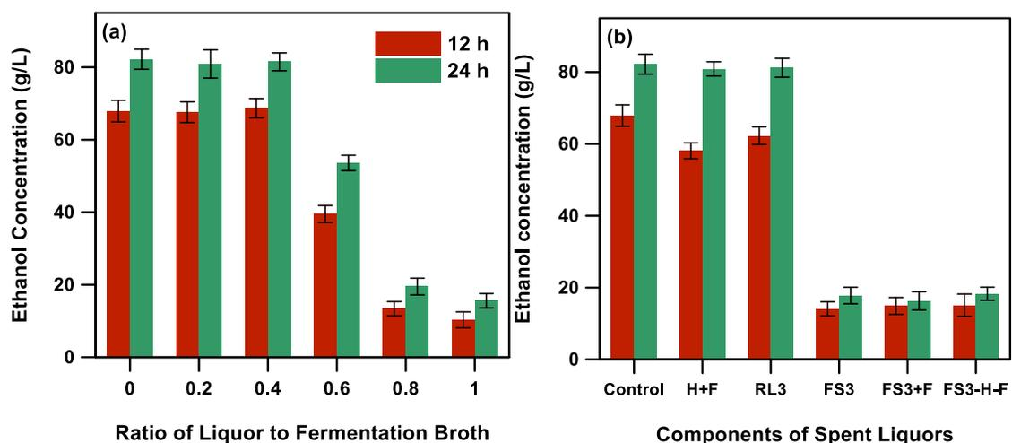
Fig. 5.5 Effects of spent liquor components to fermentation. (a) Concentrated pretreatment spent liquor at different mass ratios, and (b) different spent liquor components were mixed with standard mediums for fermentation. H: HMF; F: Furfural; FS3: <3 kDa filtrate; RL3: >3 kDa retentate; +F: furfural was added into the broth to offset the loss of the concentration process; -H-F: filtrate with no HMF or Furfural.
