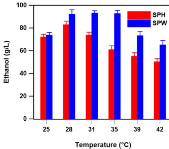
Fig. 5.3 Performance of *S. cerevisiae* in SSF at 25, 28, 32, 35, 38 and 40°C. SPH: sulfite pretreated washed slurry; SPW: sulfite pretreated whole slurry.
