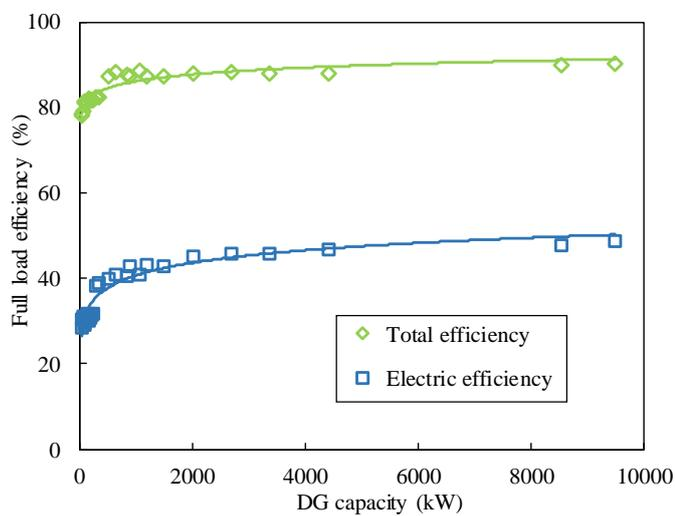
Figure 3.4 DGs full load efficiencies of different capacities
