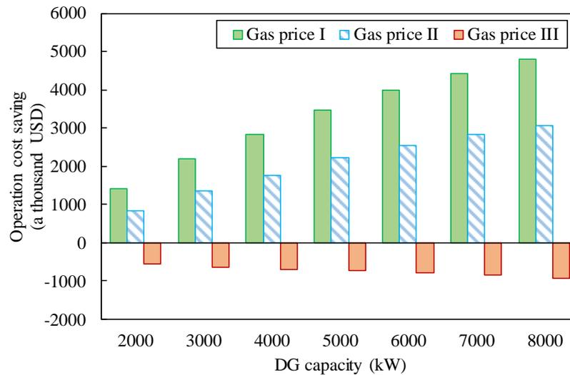
Figure 4.10 The operation cost savings under different gas prices
