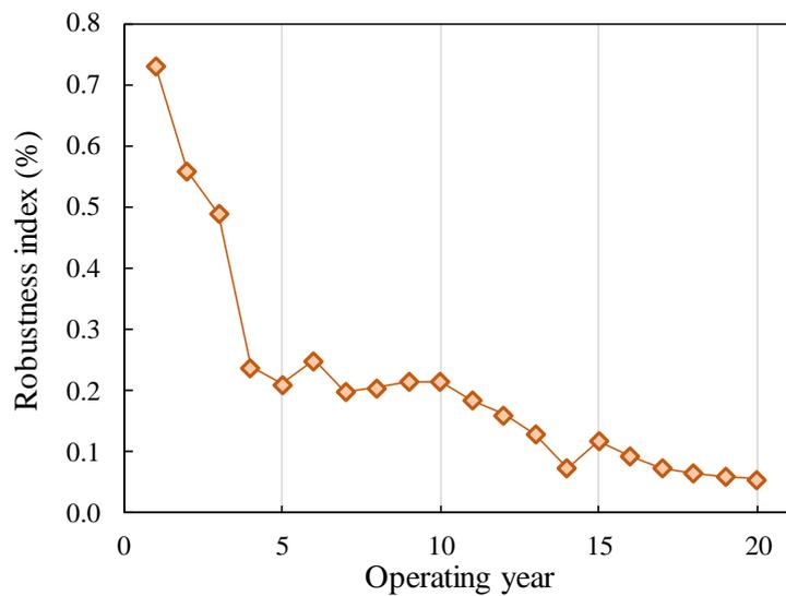
Figure 8.5 Robustness index of DES annual total system energy efficiency vs operating year
