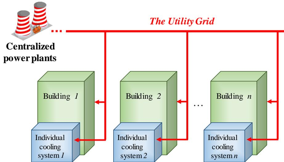
Figure 6.2 District power distribution architecture of the existing centralized energy system
