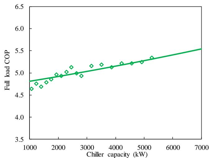
Figure 3.6 Electric chillers full load COP of different capacities
