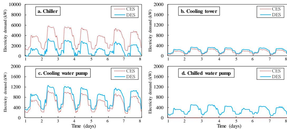
Figure 6.9 Electricity demand of electric chillers, cooling towers, cooling water pumps and chilled water pumps of two energy systems in a typical summer week
