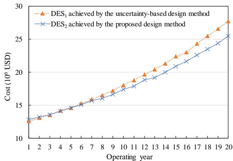
Figure 7.6 Comparison between annual total costs of  $DES$ s achieved by uncertainty-based and proposed optimal design methods
