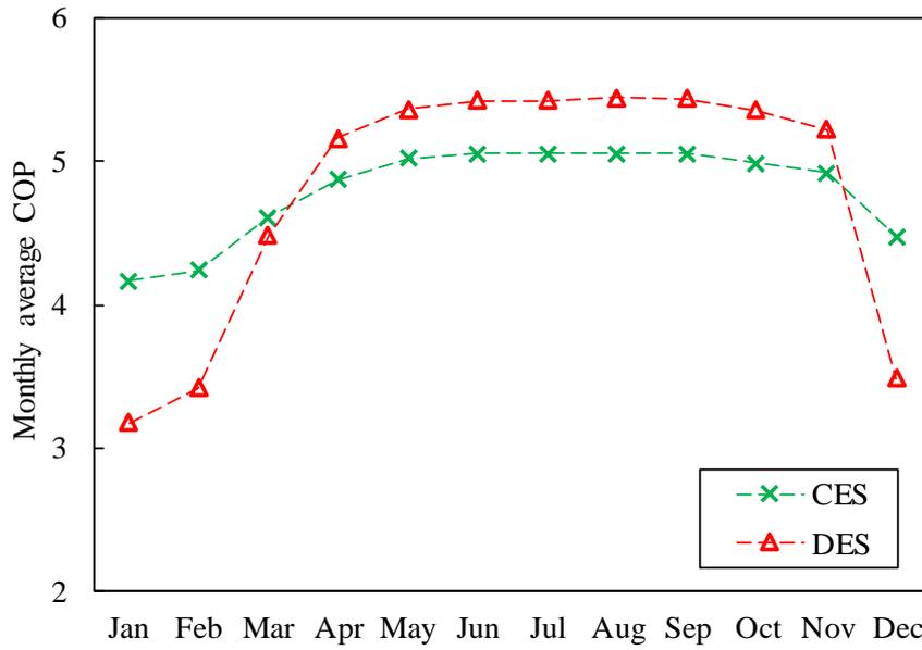
Figure 6.12 Monthly average COP of electric chiller in the DES (*Option 1*) and the CES
