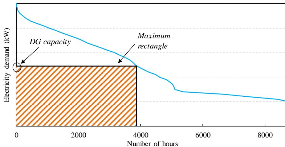
Figure 4.2 Cumulative curve and the application of MRM
