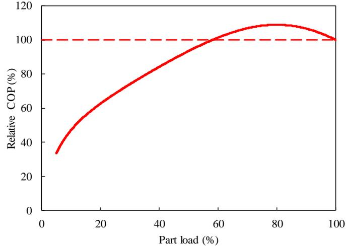
Figure 3.7 The relative COP of electric chiller at part loads
