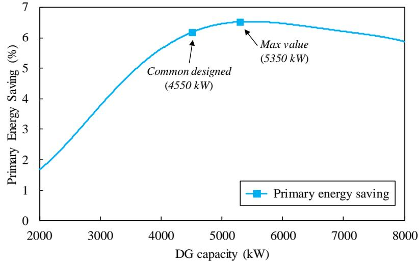
Figure 4.5 Energy performance of DESs of variable DG capacities when selling electricity is not permitted
