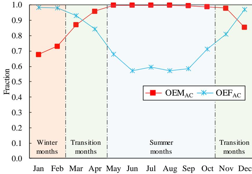
Figure 6.11 Matching indices of absorption chillers in a year
