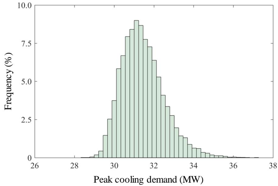
Figure 7.3 Distribution of peak cooling demand in the DES lifetime
