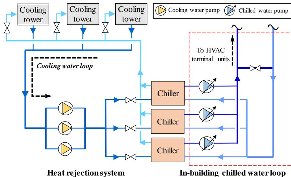
Figure 6.3 Schematic of typical individual cooling systems of buildings in the centralized energy system
