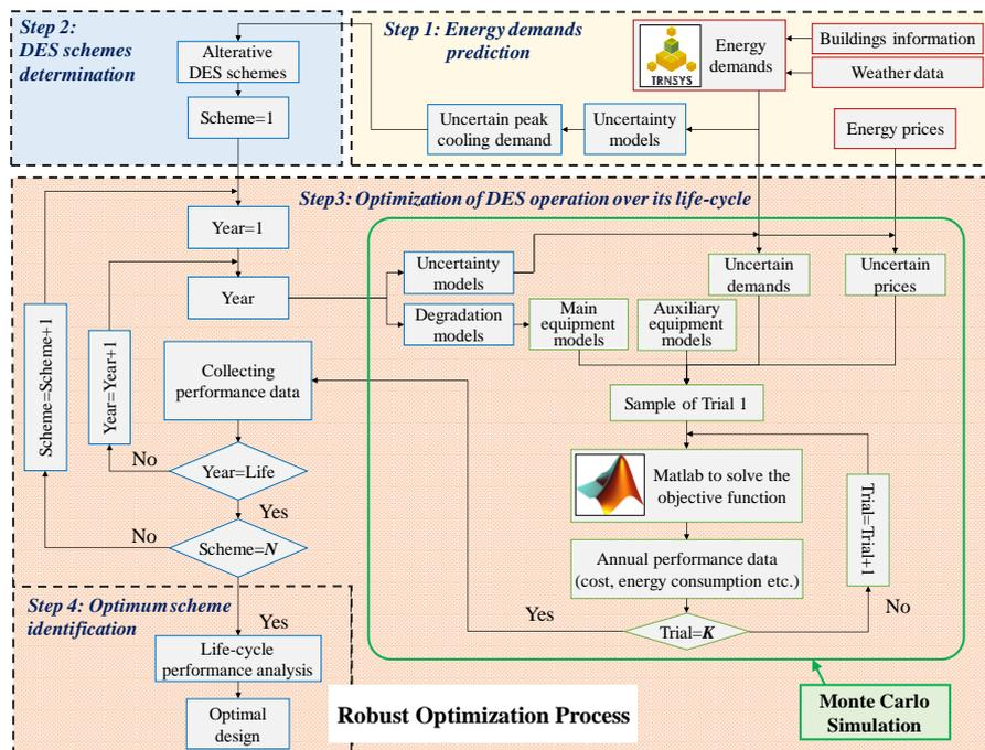
Figure 5.4 Flowchart of the proposed robust optimal design method
