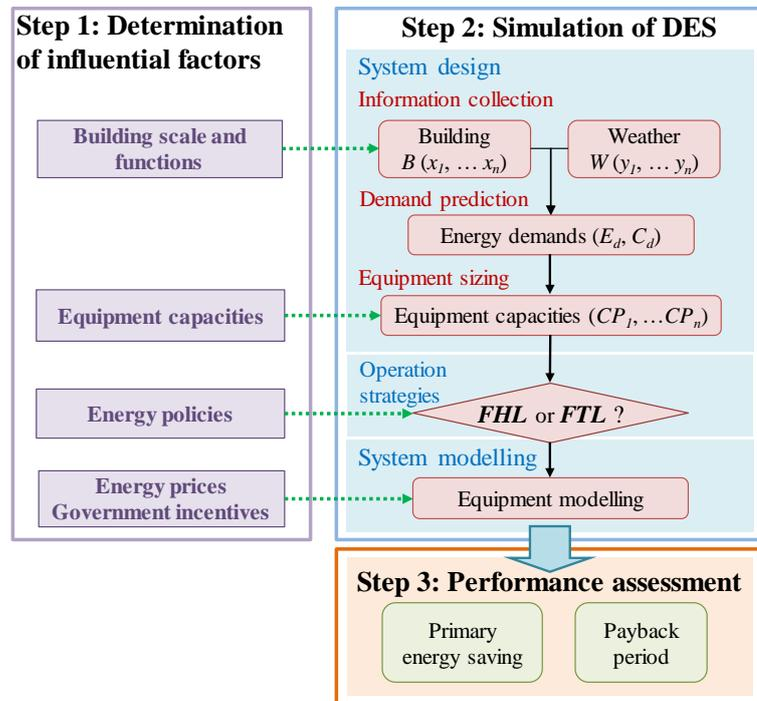
Figure 4.1 Procedures for identification of influential factors on DES performance
