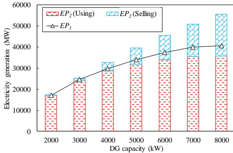
Figure 4.8 Annual electricity generations of DESs under different grid interaction policies
