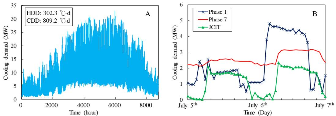
Figure 6.4 Annual profile of total cooling demand (A) and the cooling demands of three different buildings (B) of the district (Year: 2015)
