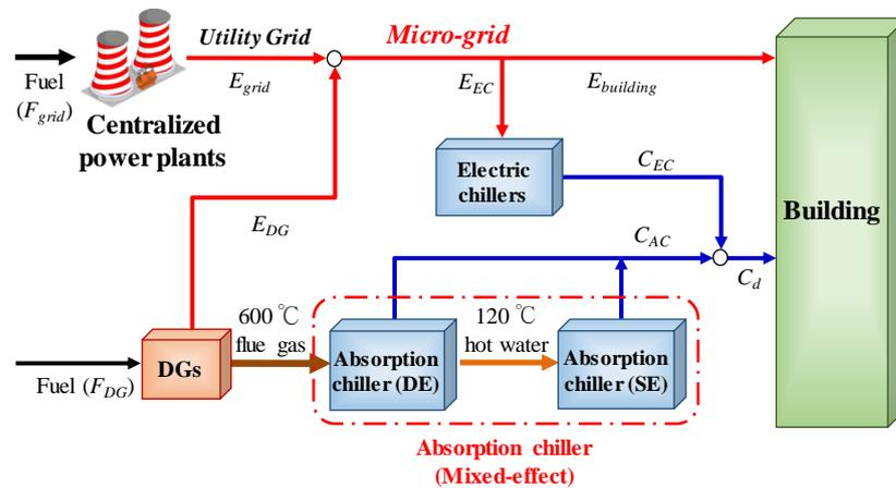
Figure 3.1 A typical configuration of the building level DES
