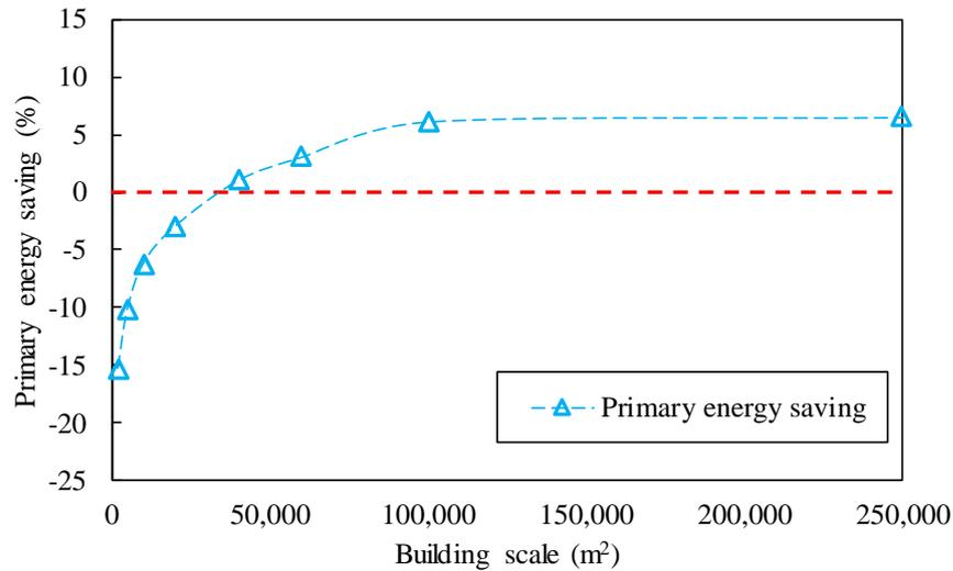
Figure 4.3 Performance of DESs vs building scale when selling electricity is not permitted
