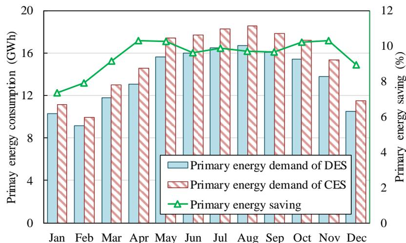
Figure 6.8 Monthly primary energy consumptions of energy systems and primary energy saving of the DES
