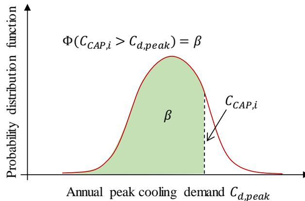
Figure 5.6 Determination of DES cooling capacity by a statistic method
