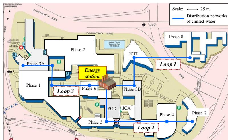
Figure 6.7 Schematic of the layout and the distribution networks of the DES
