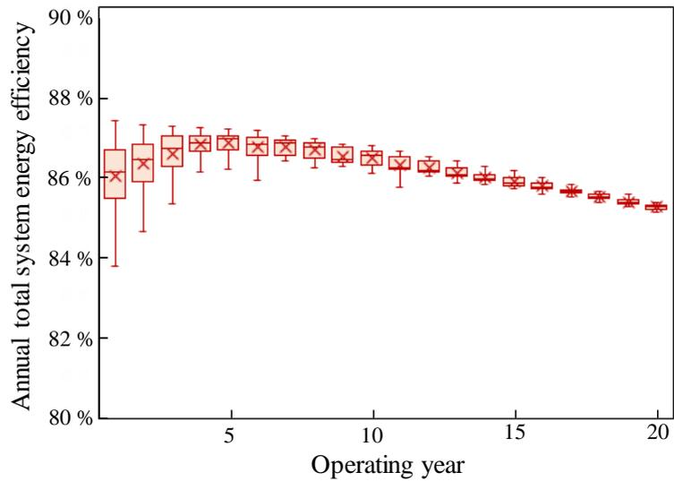
Figure 8.4 Variation of DES annual total system energy efficiency vs operating year
