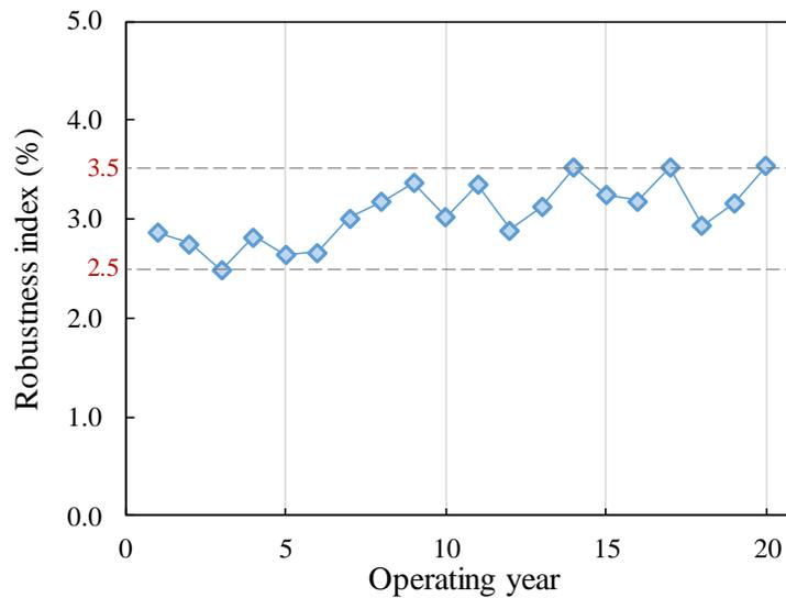
Figure 8.3 Robustness index of DES annual total cost vs operating year
