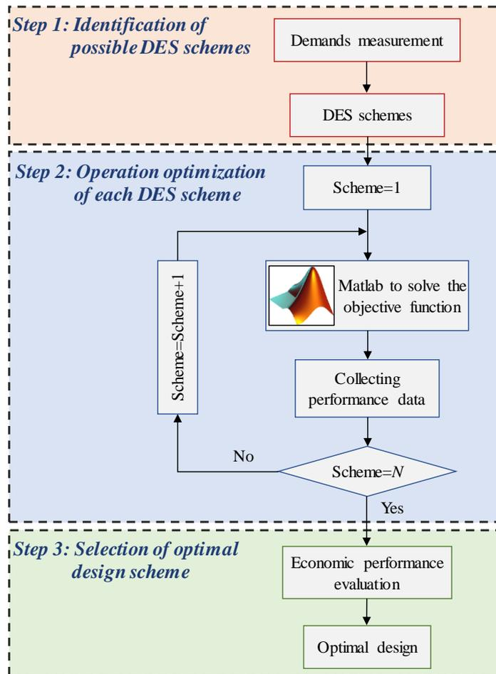
Figure 5.1 Flow chart of the optimal design for energy system retrofitting
