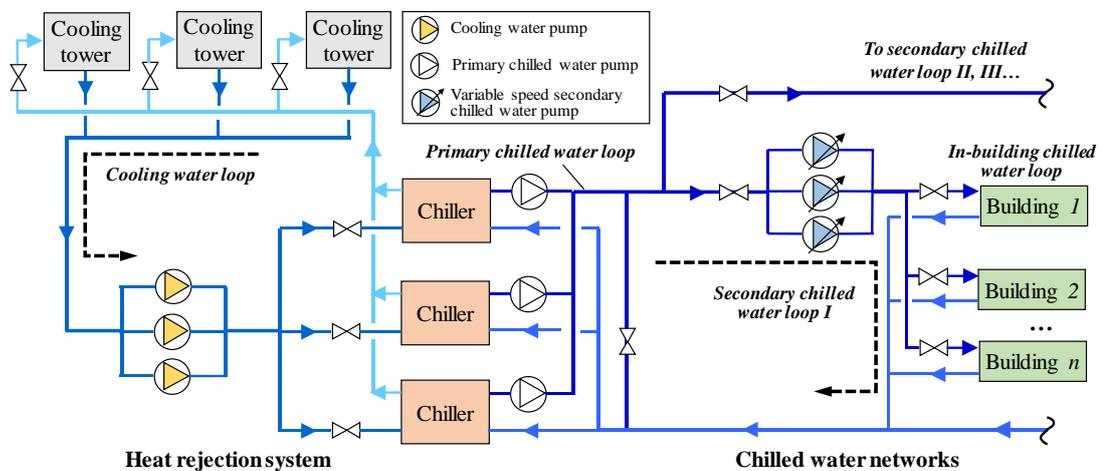
Figure 3.3 District cooling system in the DES
