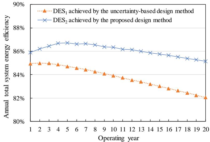
Figure 7.7 Comparison between annual total system energy efficiencies of DESs achieved by uncertainty-based and proposed optimal design methods
