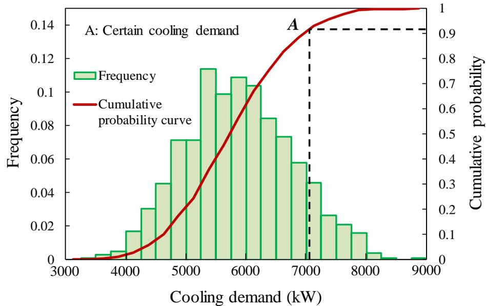
Figure 7.2 Distribution of uncertain cooling demand of a building in a typical hour
