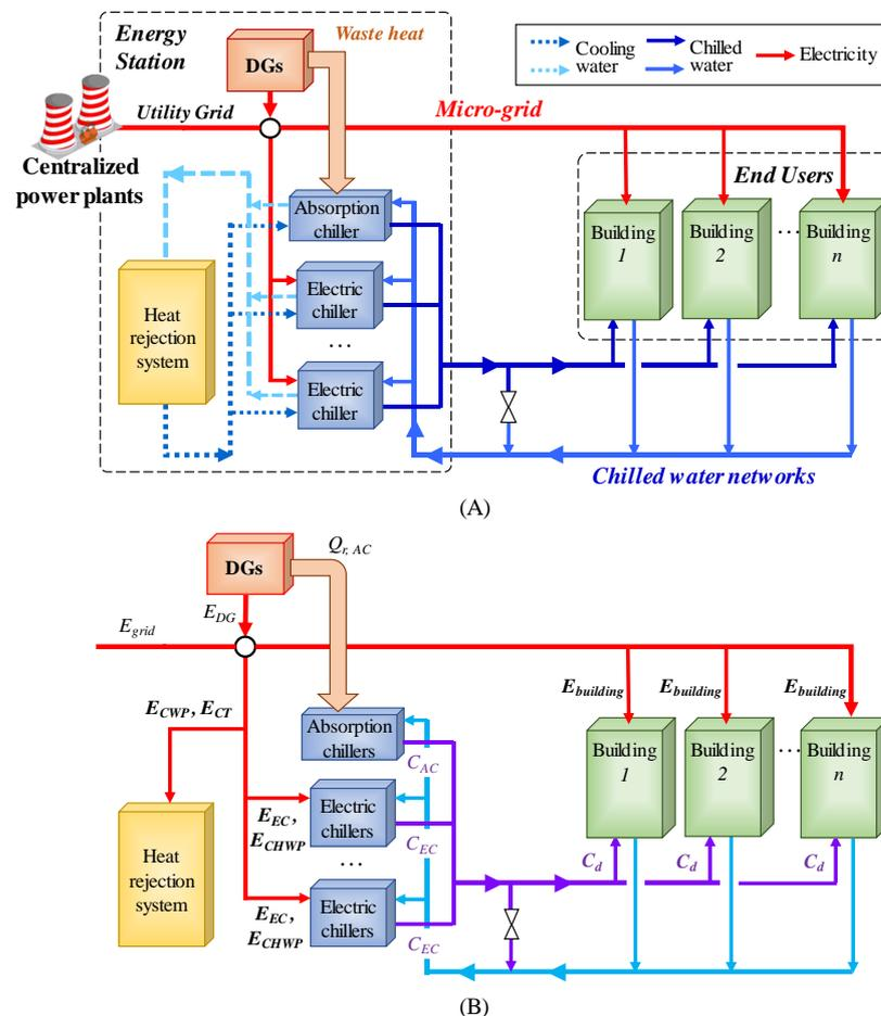
Figure 3.2 A typical configuration of a district level DES (A) and the energy fluxes in the DES (B)
