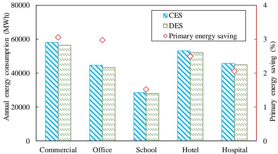
Figure 4.4 Performance of DESs in buildings of different functions when selling electricity is not permitted
