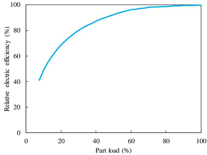
Figure 3.5 The relative electric efficiencies of DG at part loads
