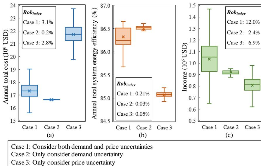
Figure 8.6 Comparison of DES performance robustness under impacts of different uncertainties
