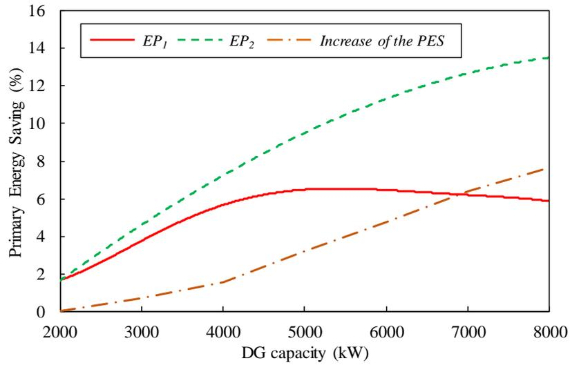
Figure 4.7 Energy performance of DESs under different grid interaction policies
