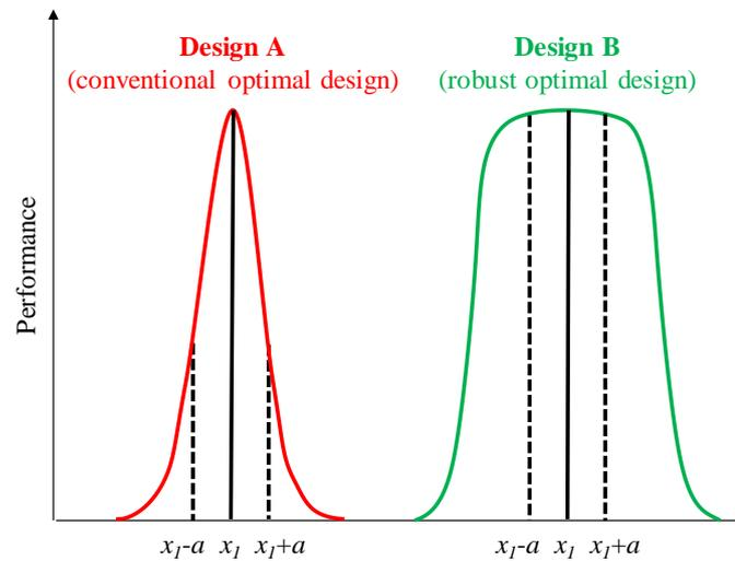
Figure 5.2 Illustration of the performance of robust optimal design
