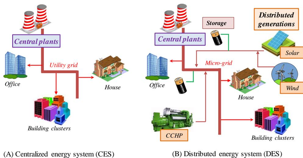
Figure 2.1 Schematics of centralized energy system (CES) and distributed energy system (DES)
