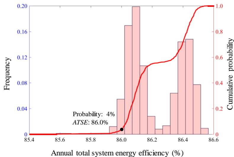
Figure 8.8 Probability distribution of annual total system energy efficiency of the optimum DES
