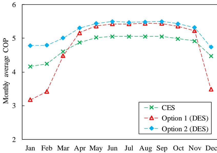
Figure 6.13 Comparison of monthly average COP of electric chillers of *Option 1* (DES) and *Option 2* (DES)
