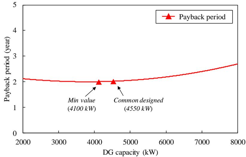
Figure 4.6 Economic performance of DES of variable DG capacities when selling electricity is not permitted
