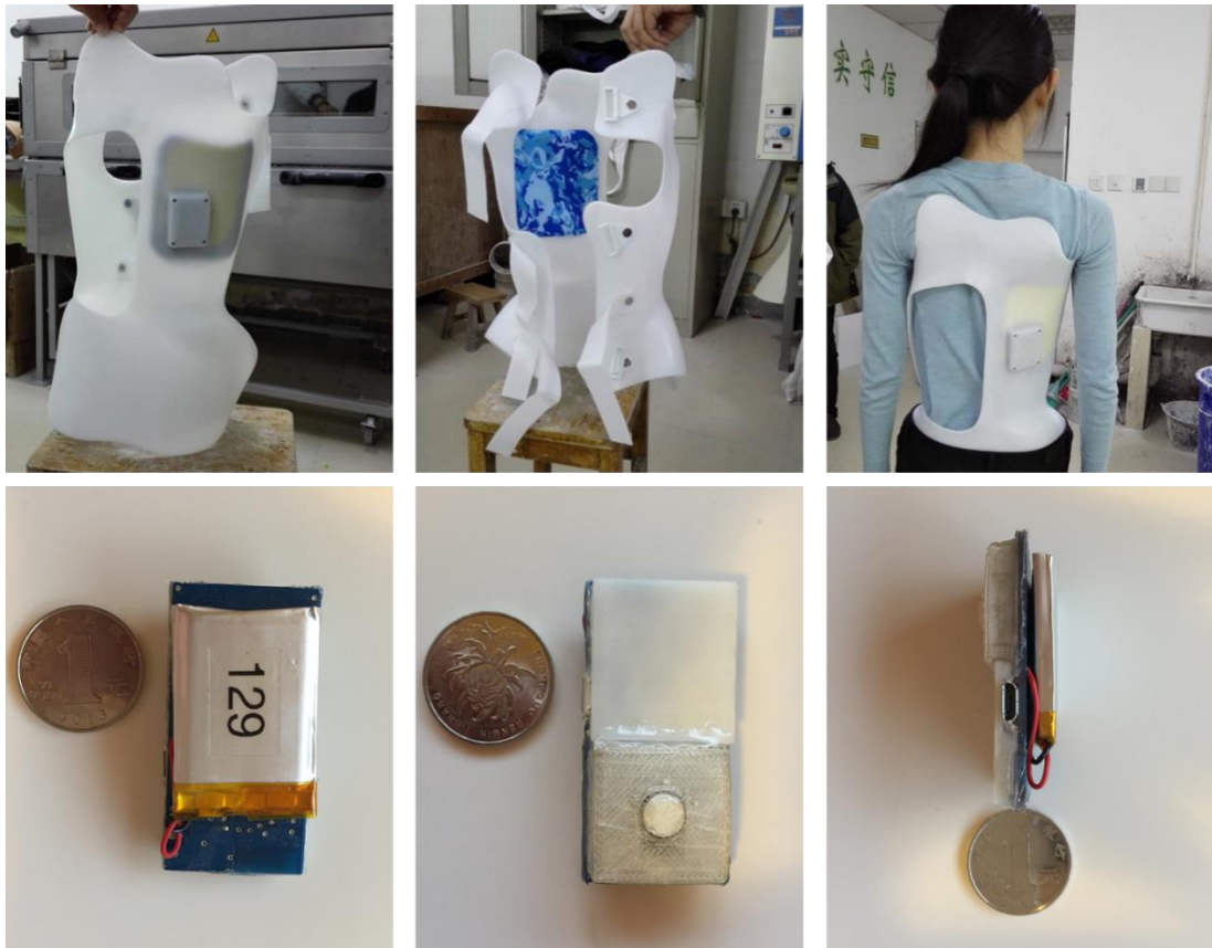
Figure 3.14 Embedded thermo-force sensor
