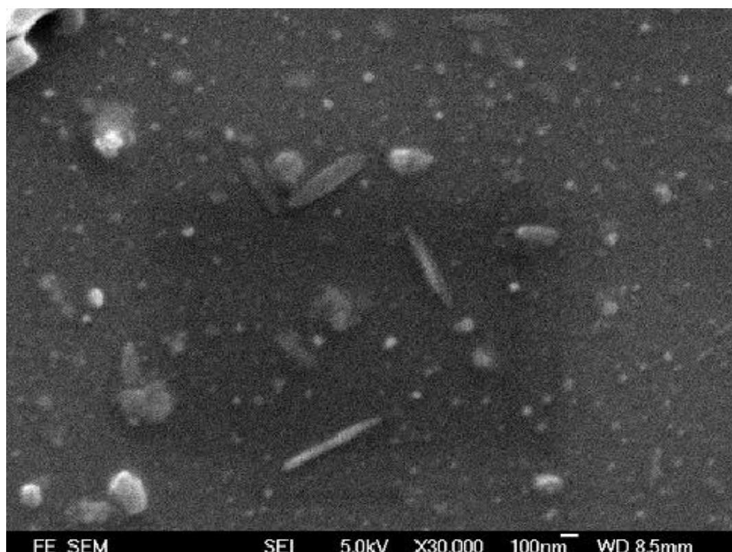
Figure 3.4 SEM image of the third pulverised wool particles of 30,000x
