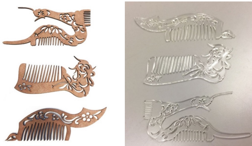
Figure 6.3 The outcomes of laser cutting combs in wood and acrylic materials.
