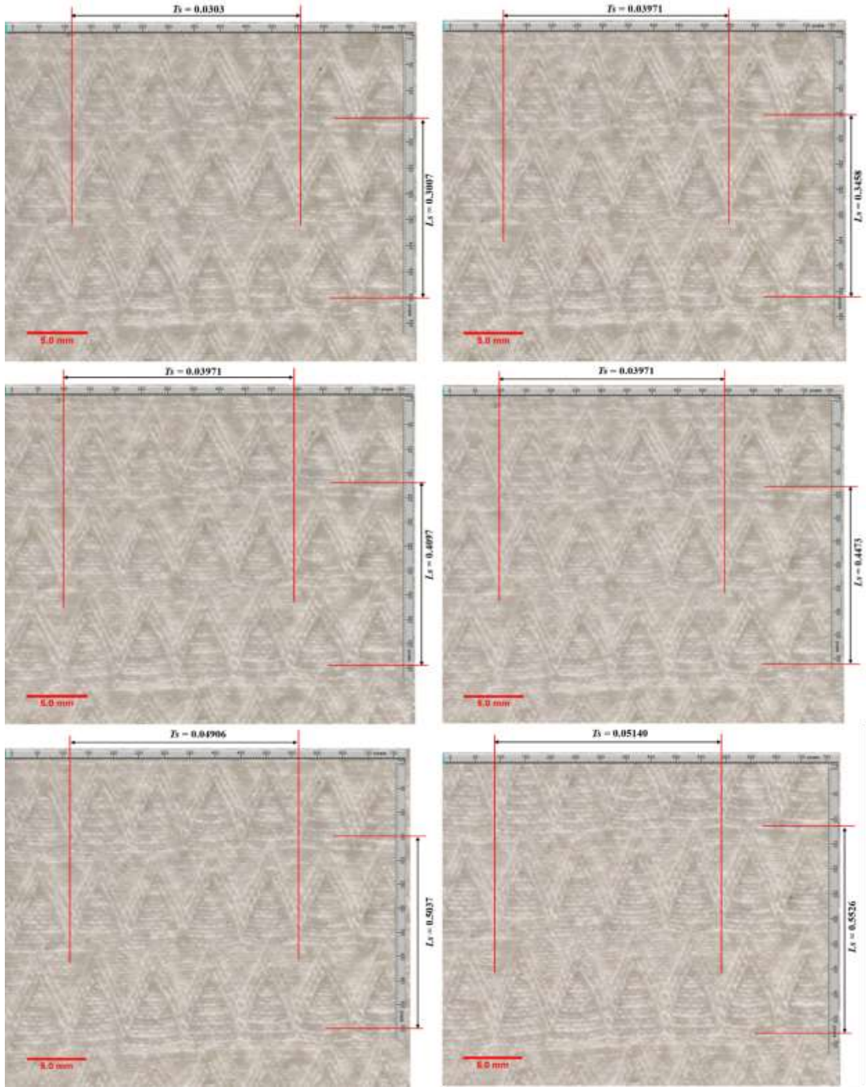
Figure 5.5 Photos of fabric V 2 F 3 taken at different tensile strain when stretched along WD
