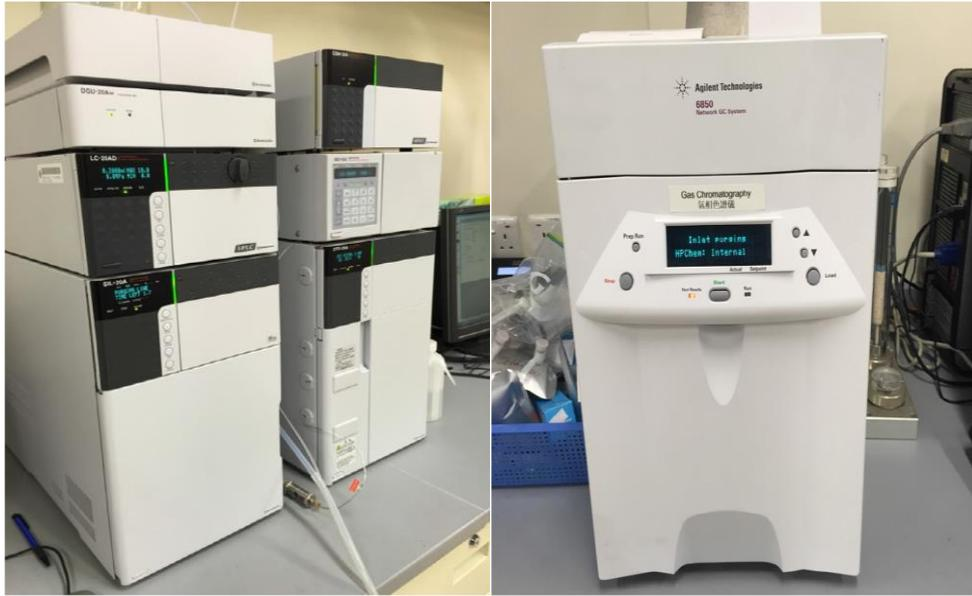
**Figure 3-3.** The HPLC system (SHIMADZU) used for quantification of the target compounds and GC system (Agilent) used for quantification of the target gases.
