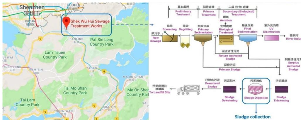
**Figure 3-1.** Source of the inoculum sludge used in our study (Drainage Services Department, Hong Kong).
