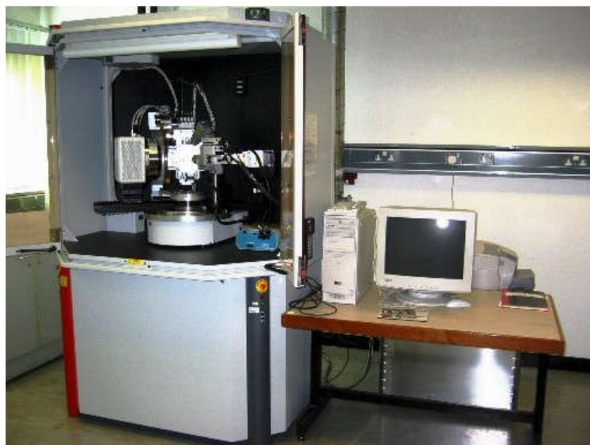
Figure 4.2 X-ray Diffractometer
