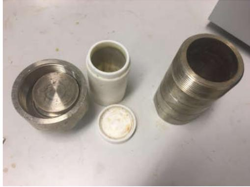
Figure 4.9 Hydrothermal Reactor
