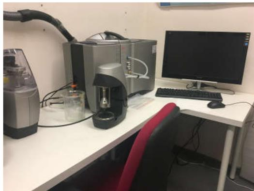
Figure 4.5 Laser Particle Analyzer (Mastersizer 3000)
