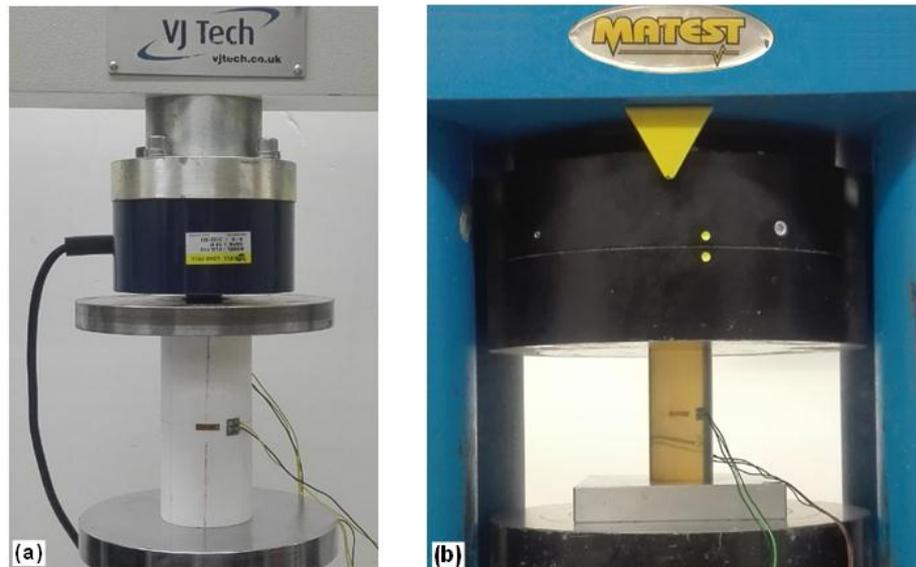
Figure 3.2 Testing equipment. (a) VJ Tech tester with a loading capacity of 100 kN; (b) Matest with a loading capacity of 3,000 kN
