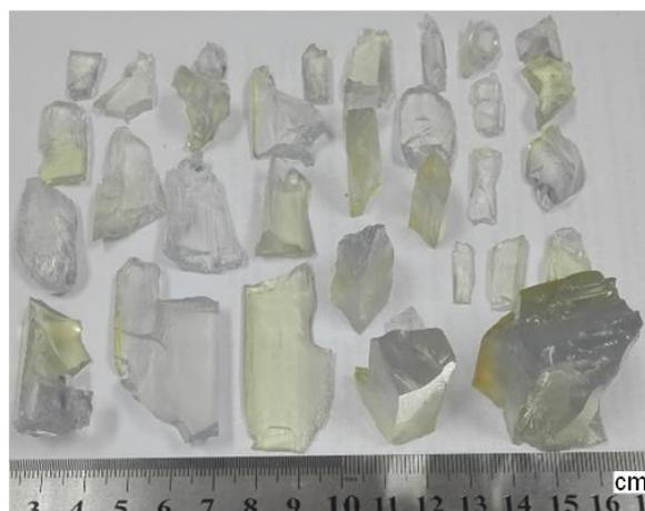
Figure 3.7 Fragments of resin sample after low temperature testing
