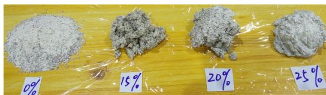
Figure 7.4 Illustration of sand-clay mixture with different water content
