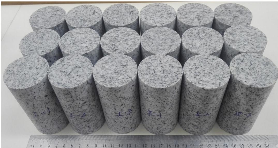
Figure 6.2 Prepared granite samples
