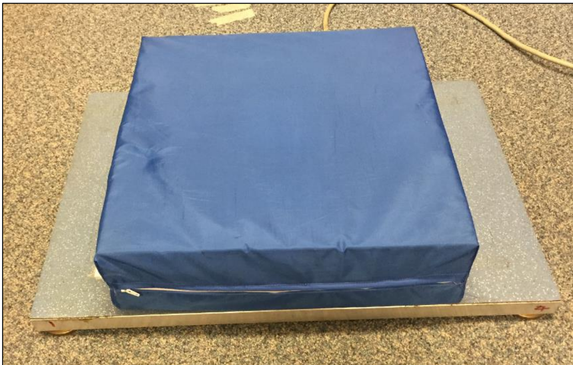
Figure 7.1 A foam (39 cm × 39 cm × 10 cm thickness) on a force plate
