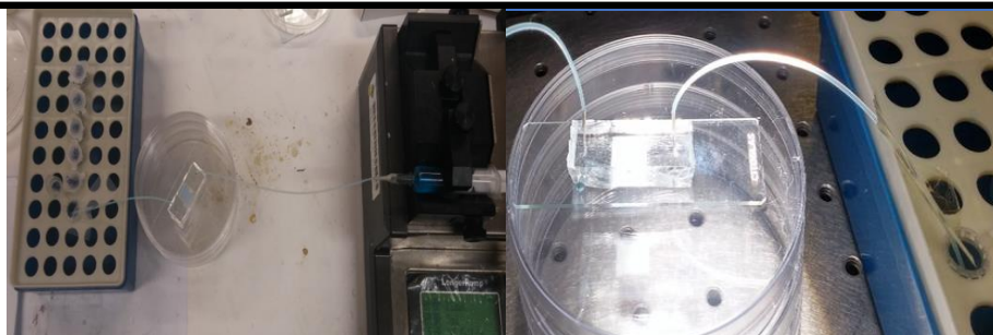
Figure 4.7 Experimental setup. Dark reaction in every cycle (Left). Light reaction, that is, the reactor is irradiated for photocatalytic degradation at different flow rate (Right). The degraded sample was collected and tested for its absorbance.
